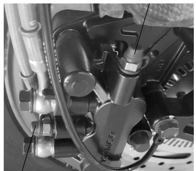
Secondary front brake tube bleed valve
