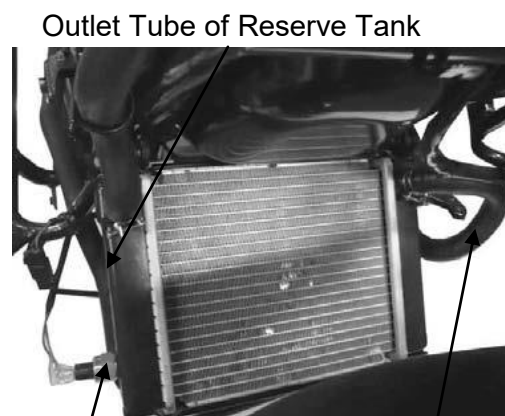
Outlet Tube of Reserve Tank Thermostatic Switch Outlet Tube of Reserve Tank
