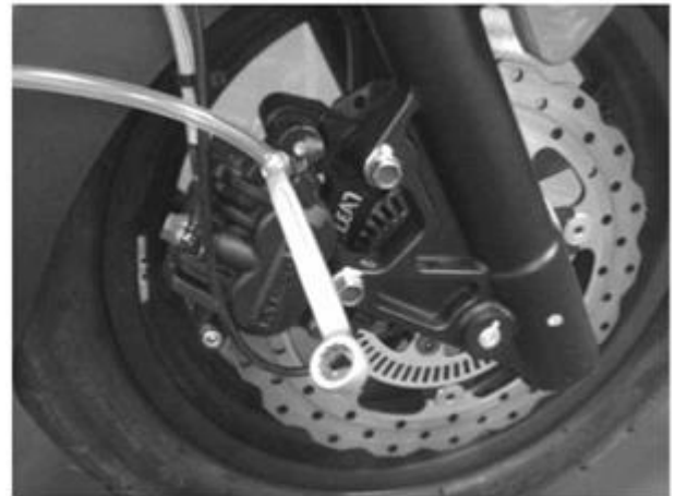
Master front brake tube bleed valve
