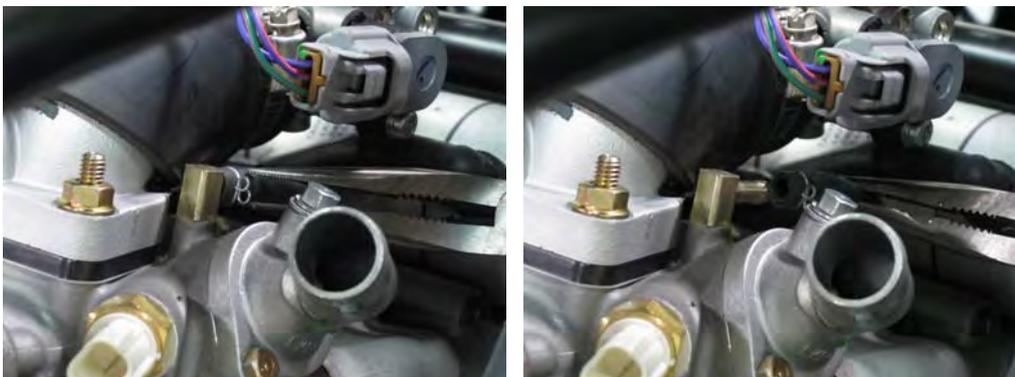
Squeeze the air bleed hose clamp with needle nose pliers and slide back the clamp. Free the air bleed hose from the thermostat.
