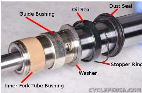
Slide off the dust seal, stopper ring, oil seal, washer and guide bushing.
