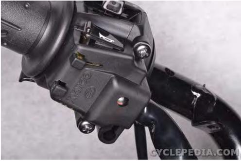
Insert the two housing screws and tighten them securely with a #2 Phillips screwdriver. Tighten the front screw before the rear.
