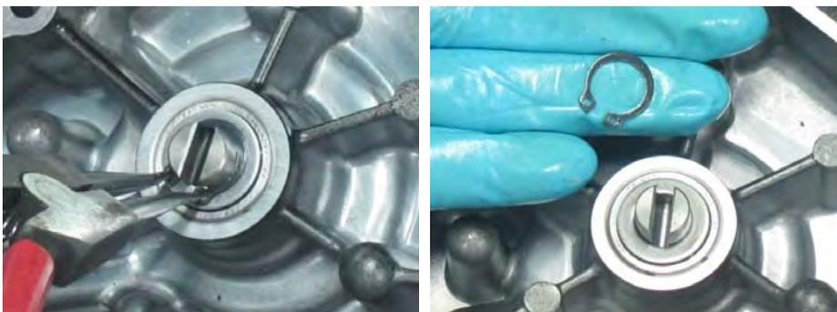
Remove the clip with the pliers and then remove the water pump shaft.
