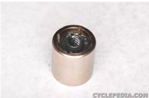
Clean the brake caliper pistons with steel wool. Inspect the brake caliper pistons for wear and damage.
