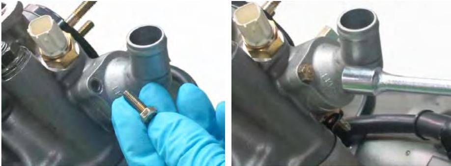
Insert the two thermostat bolts and tighten them securely with an 8mm socket.
