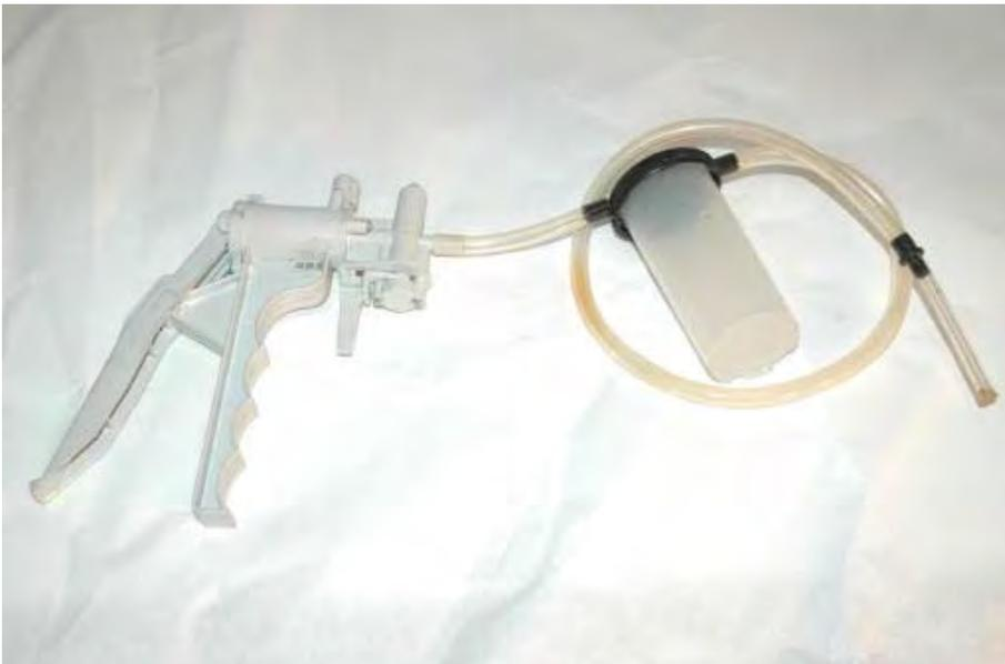
Open the valve and remove the old brake fluid with a Mighty -Vac or a similar device.
