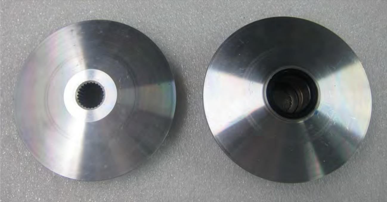
Inspect the faces of the drive pulley. Clean away any grease from the faces.
