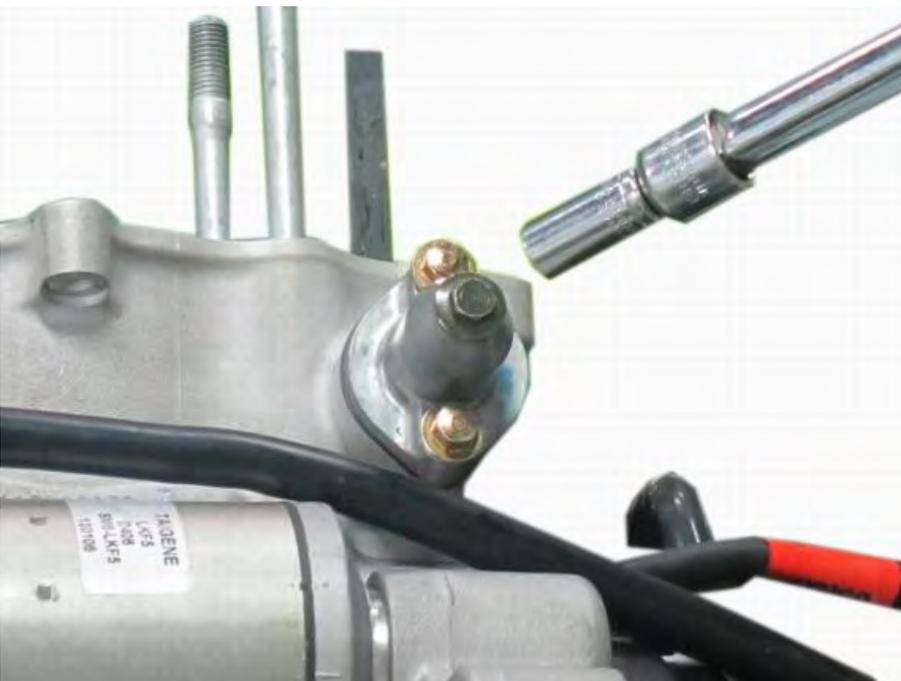
Install the cam-chain tensioner with a new gasket. Insert the mounting bolts and tighten them evenly to specification with an 8 mm socket. Remove the screwdriver and release the cam-chain tensioner rod.
