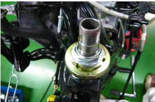
Support the lower fork clamp and thread on the steering stem adjusting nut.
