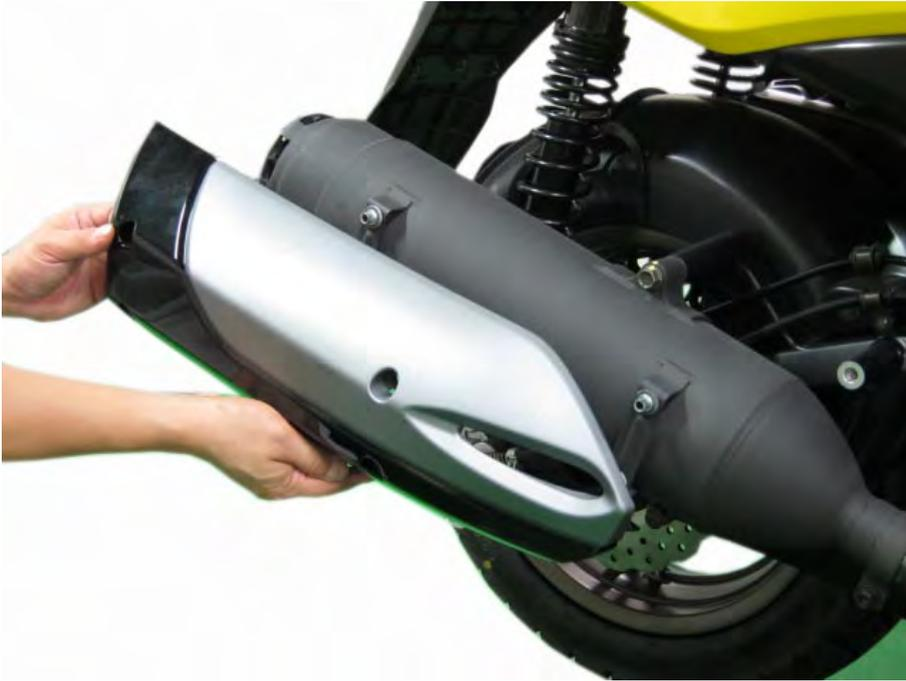
Remove the heat shield.
