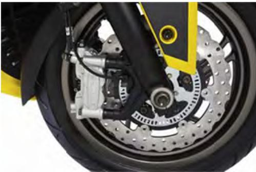
The brake calipers are each mounted to the front fork with two bolts.
