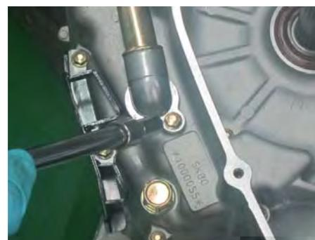
Fit the coolant hose to the right crankcase cover pipe. Secure the hose with the clamp and tighten the coolant hose clamp securely with a #2 Phillips screwdriver.
