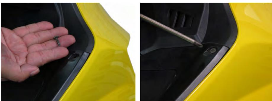
Install the four front cover mounting screws and tighten securely with a #2 Phillips. There are two screws on each side.
