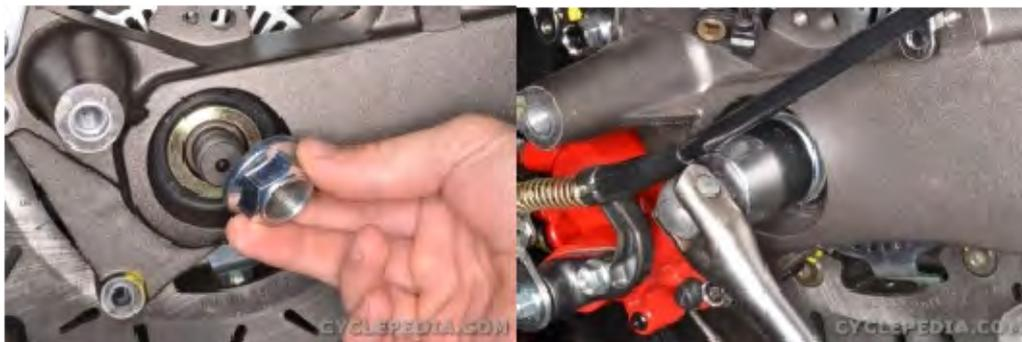
Install the rear axle nut and tighten it to specification with a 24 mm socket.
