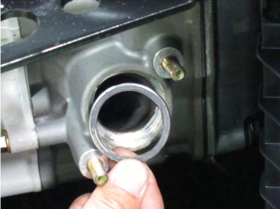
Remove the exhaust pipe gasket and discard it.
