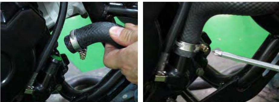
Connect the coolant hose to the water pump. Move the clamp into place and tighten it securely with a #2 Phillips screwdriver.
