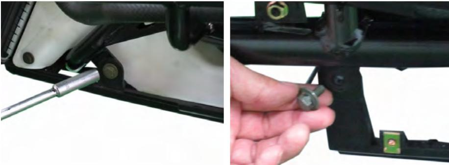
Remove the two under cover bolts on both sides with a 10 mm socket.
