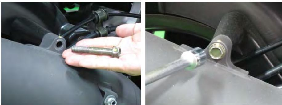
Install the three muffer mounting bolts and tighten to specification with a socket.
