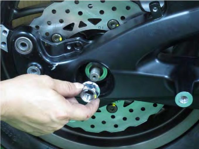
Install the rear axle nut and tighten it to specification with a 24 mm socket.
