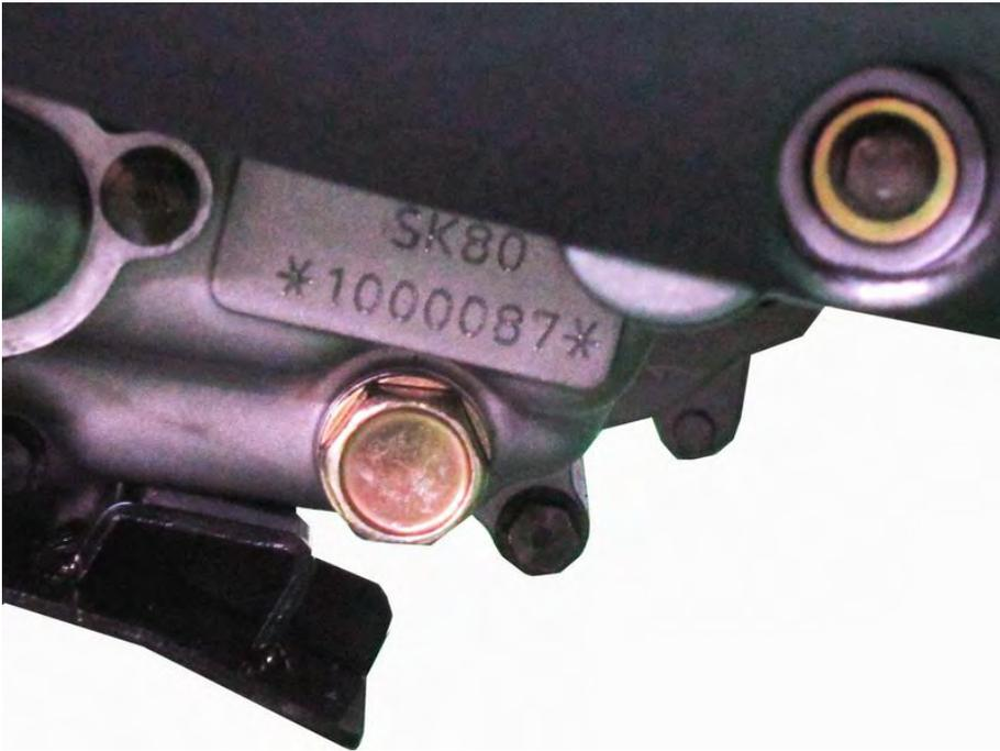
Place an oil pan under the engine. The oil drain bolt is located on the left side of the engine.
