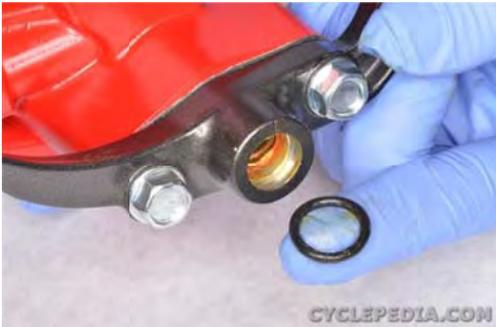
Lubricate the new parking brake O-ring with silicone grease and fit it into place.
