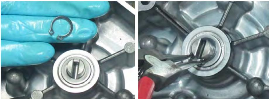
Hold the water pump shaft and install the impeller with pliers.
