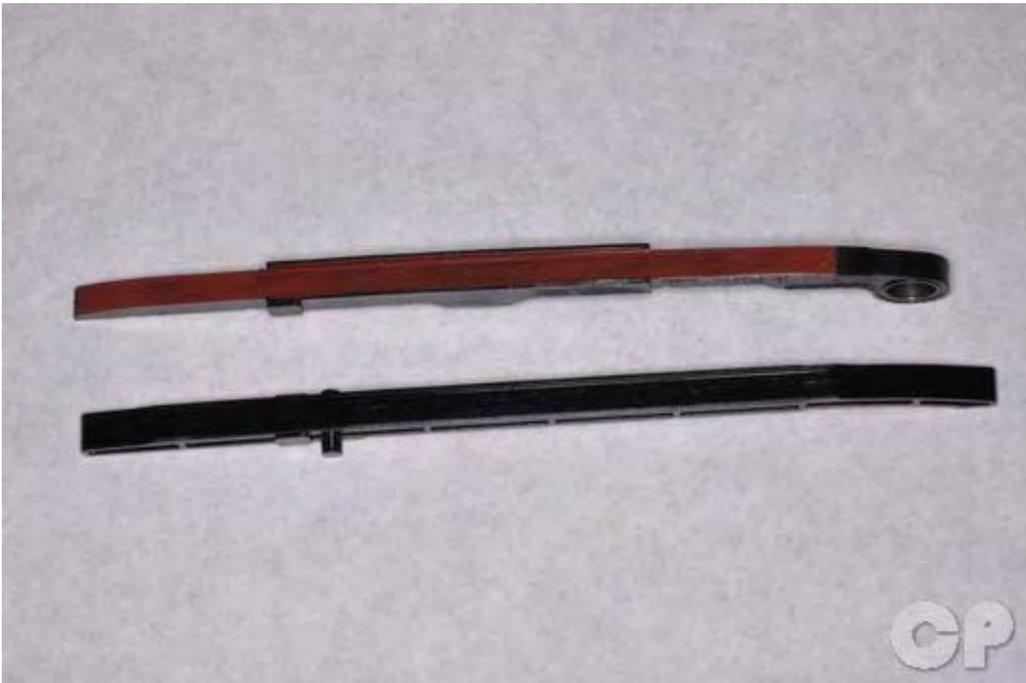
Inspect the cam chain guides for damage and excessive wear. Replace the guides as needed.
