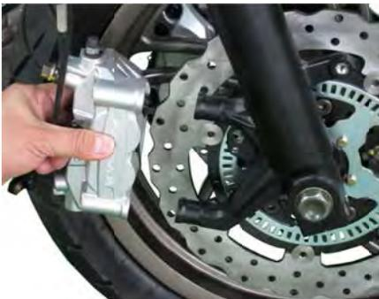
Install the front caliper. Guide the brake disc between the pads. Line up the caliper bracket mounts with the fork.
