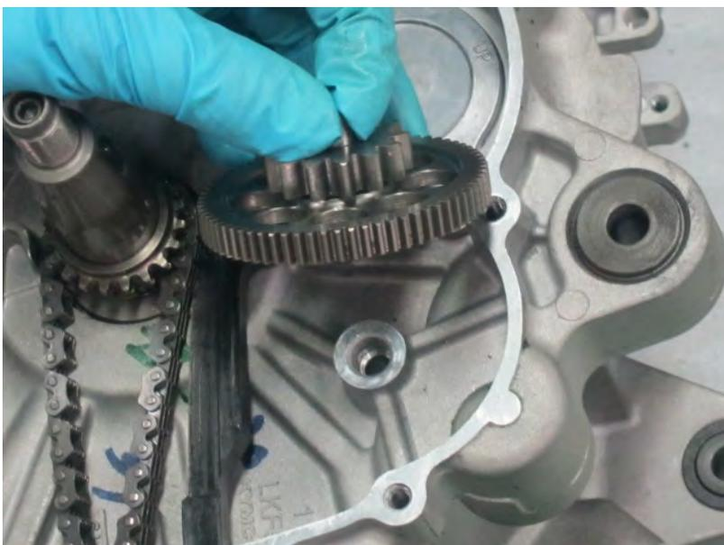
Lubricate the starter idle gear shaft with fresh engine oil. Install the starter idle gear and shaft into the crankcase.
