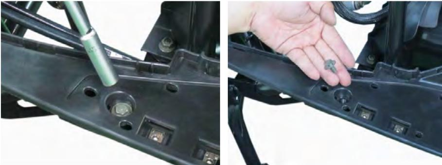
Remove the three mounting bolts on right side with a 10 mm socket.
