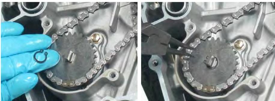
Install a new snap ring into its groove with snap ring pliers.
