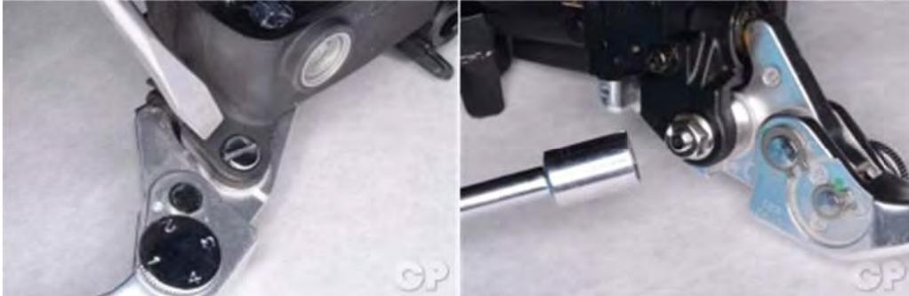
Tighten the brake lever bolt with a flat blade screwdriver and then tighten the nut with a 10 mm socket.
