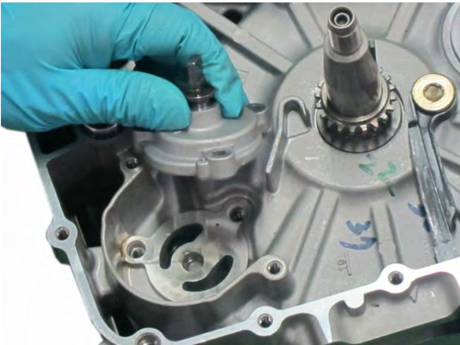
Fit the oil pump into place so that the arrow is pointing up.
