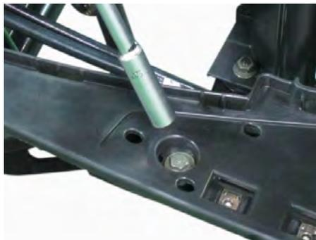
Install the three mounting bolts on right side with a 10 mm socket.
