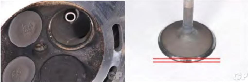
Inspect the valve seat and the valve seat width. The valve seat should be centered on the valve face. If the seat is pitted, worn out, or fits poorly on the valve face the valve seat must be resurfaced.
