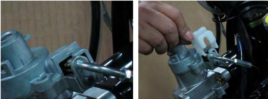
Install the seat latch cable cover.
