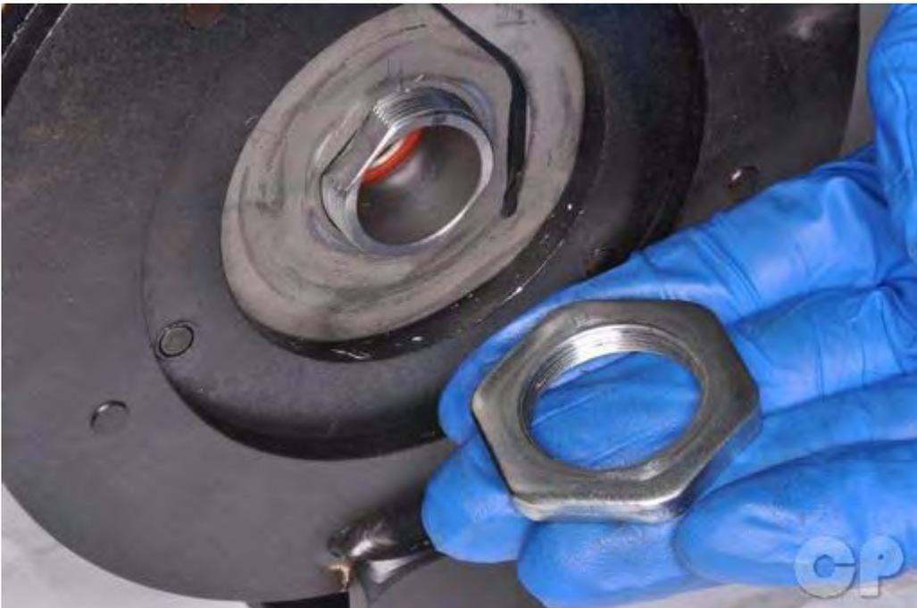
Remove the clutch drive plate nut.
