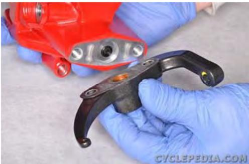
Remove the parking brake bracket and gasket.
