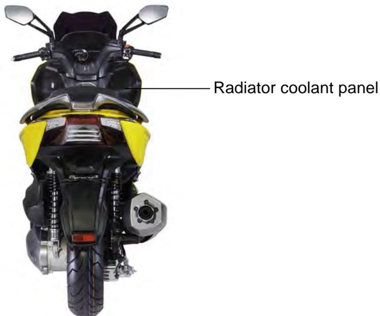
Remove the radiator coolant panel screws with a #2 Phillips screwdriver.
