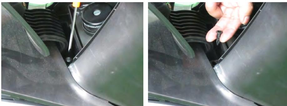
Remove the two plastic screws from the front of center cover.
