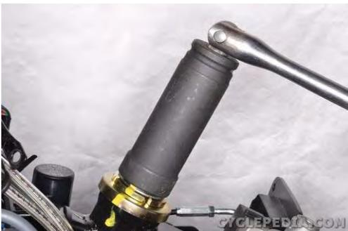
Torque the steering stem lock nut to specification with the lock nut wrench special tool.
