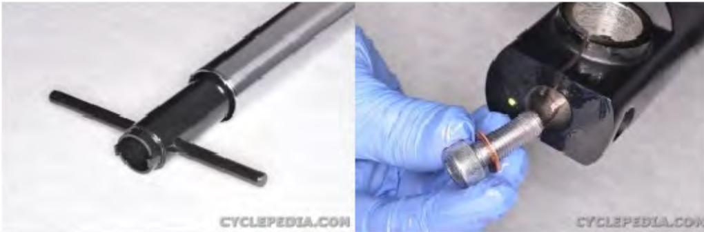
Place the axle holder of the outer fork tube in a soft jawed vise. Use a suitable damper rod holder tool to keep the damper rod from turning. Insert the fork bottom bolt with a new sealing washer. Tighten the fork bottom bolt securely with an 8 mm Allen socket. If a damper rod holder tool is unavailable temporarily install the fork components.
