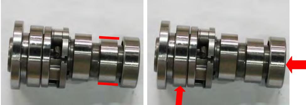
Inspect the camshaft cam heights for the intake and exhaust lobes.
