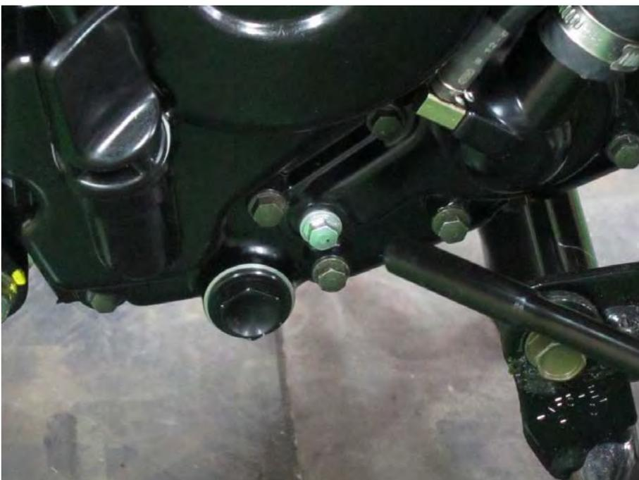
Loosen the coolant drain bolt with an 8 mm socket.
