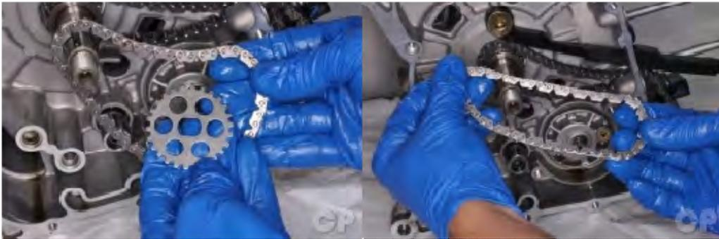
Inspect the oil pump drive chain and sprocket for signs of wear and damage. Replace the parts as needed.
