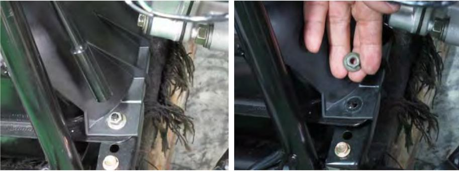
Remove the left fuel tank mounting nuts.
