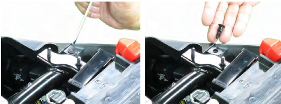
Remove the two seat plastic screws from the front of body cover.
