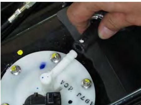
Remove the fuel hose with a plier. Slide back the clamp and free the injector fuel hose from the fuel pump pipe. Clean up any remaining fuel immediately.
