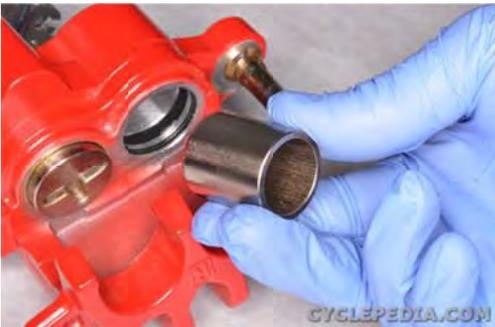
Remove the normal rear caliper piston.
