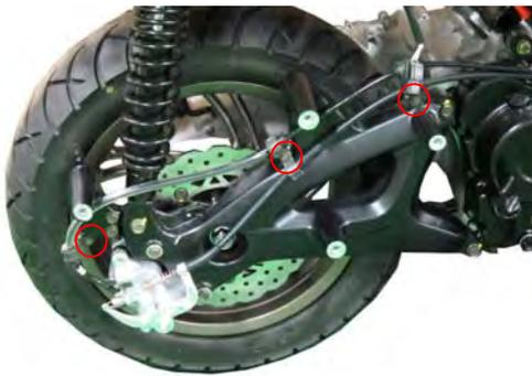
Remove the rear wheel hose clamp bolts with an 8 mm socket.
