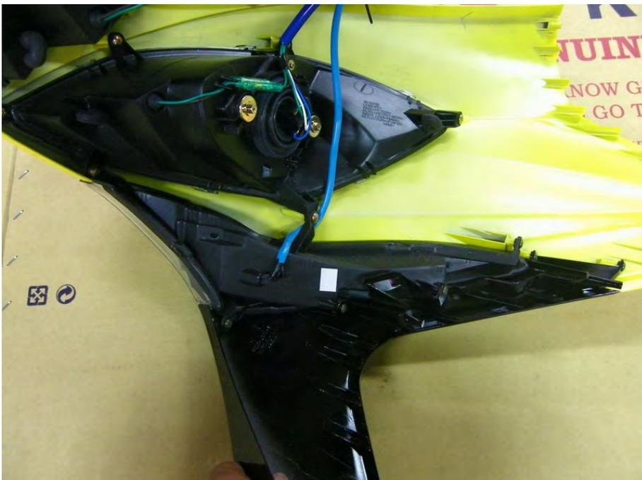
Remove the front turn signals LED mounting the front turn signals housing.
