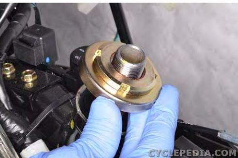
Support the lower fork clamp and remove the steering stem adjusting nut
