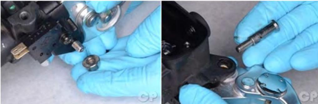
Remove the pivot nut and bolt.
