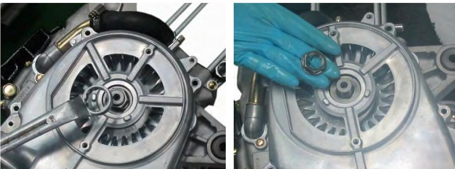
Remove the #M18 nut mounting the drive face.
