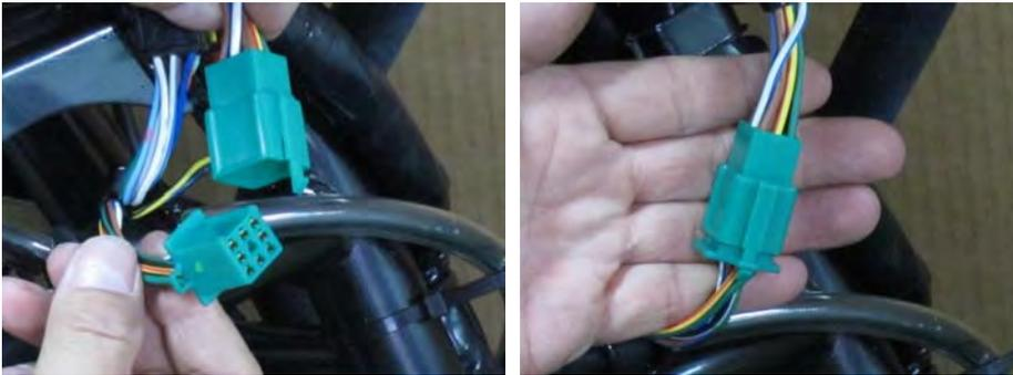
Plug in the green connectors for the right handlebar switches.
