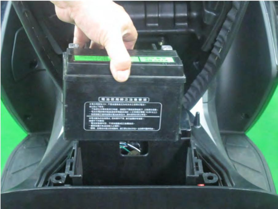
Lift the battery out of the battery tray.
