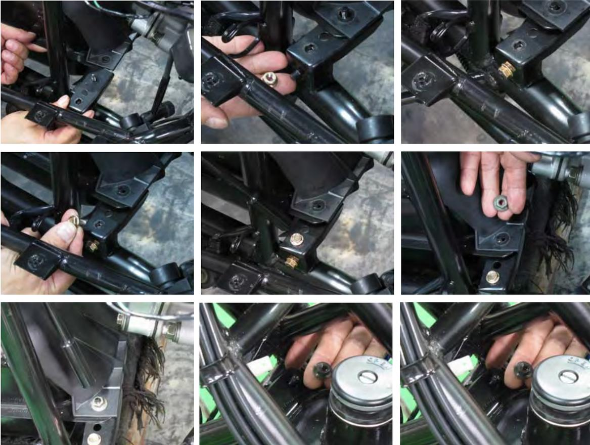
Install the brackets and nuts/bolts. Tighten the nuts/bolts securely.
