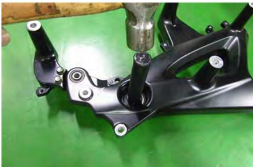
Drive in the new bearing with a suitable driver that is the same outside diameter as the bearing.
