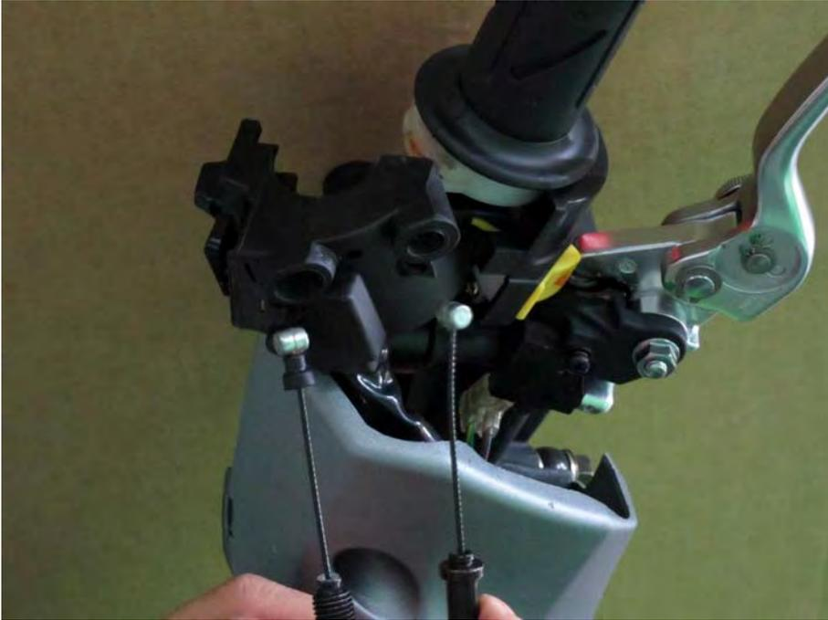
Guide the throttle cables out towards the handlebar side.
