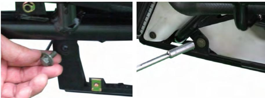
Install the two under cover bolts on both sides and then tighten securely with a 10 mm socket.
