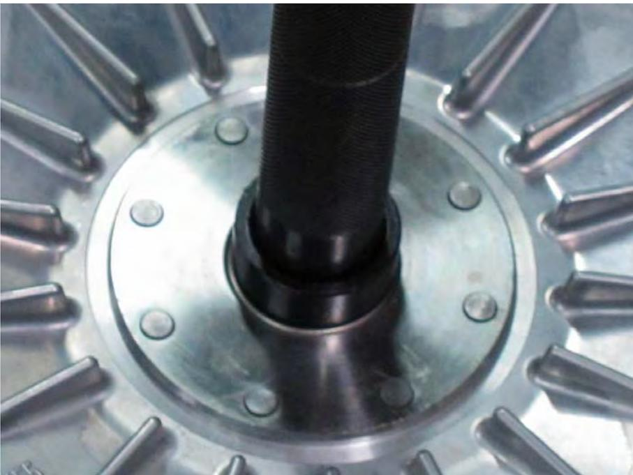
Drive in the new bearing so the sealed side face out towards the clutch. Install the snap ring into the groove. Install the collar and drive in the new needle bearing so that its markings face out. Drive in the bearings with a suitable driver with the same outside diameter as the bearing.
