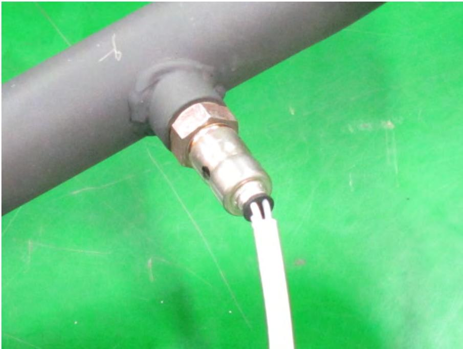
Apply anti-seize compound to the threads of the O<sup>2</sup> sensor. Install the O<sup>2</sup> sensor and tighten it to specification with a 17 mm wrench. Use care not to pinch the wires.
