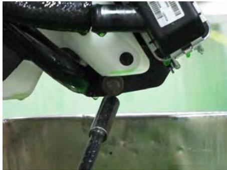
Install the two radiator bottom mounting bolts with a 10 mm socket.
