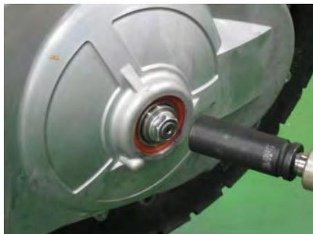
Install the driven pulley nut with a 24mm socket.
