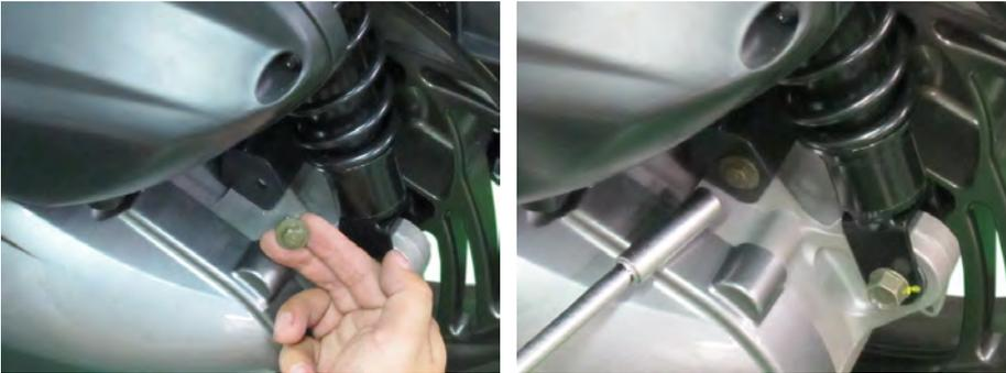
Install the left fender mounting bolts with a 10 mm socket on the back side.
