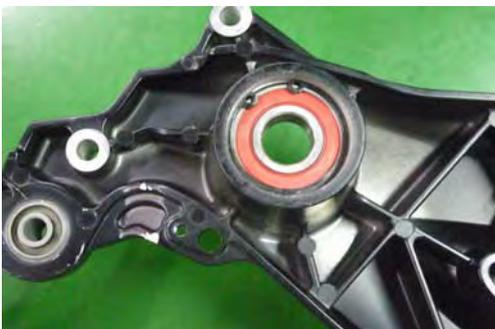
Remove the seal and snap ring.
