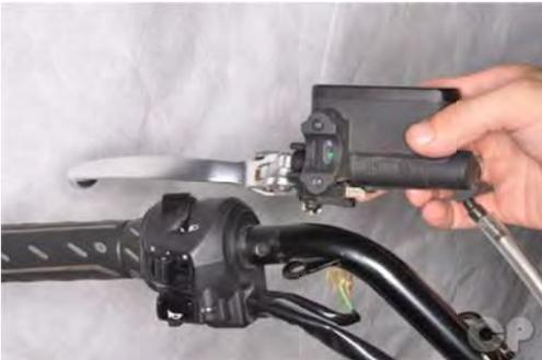
Position the master cylinder on the handlebar.
