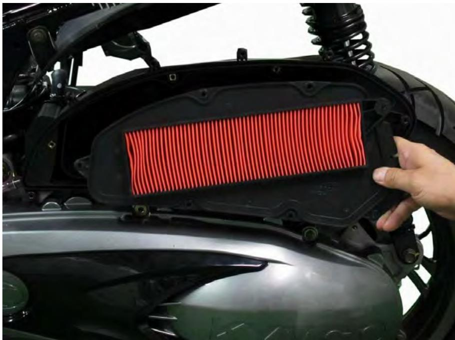
Fit the new air filter into place.
