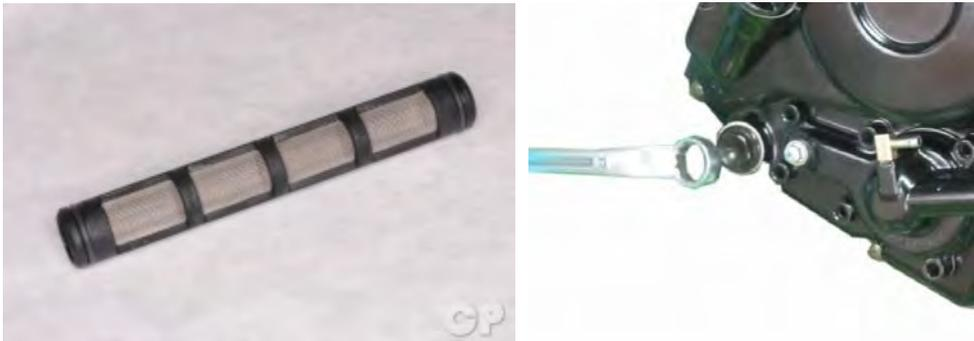
Return the O-rings to the oil strainer screen and install it into the left side of the engine. Tighten the oil strainer screen cap to specification with a 17 mm socket.
