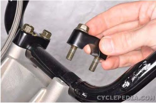
Install the upper handlebar holders so that their punch marks face forward. Insert the handlebar holder bolts.
