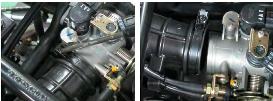
Loosen the air box connecting hose clamp screw at the throttle body with a #2 Phillips.
