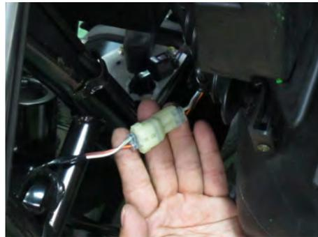
Install the connector output voltage device.
