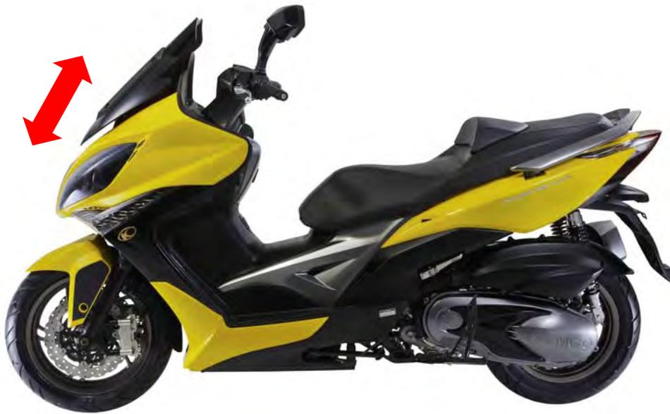
Check the action of the front shock absorbers by compressing them several times. Check the entire shock absorber assembly for oil leaks, looseness or damage.
