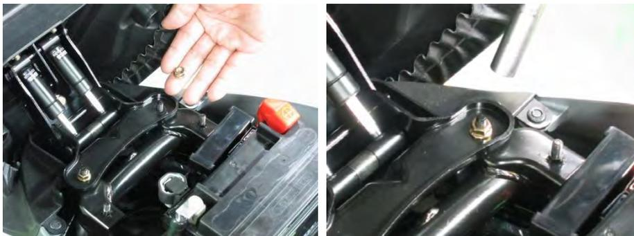
Install the two luggage box hinge nuts and tighten securely with a 10 mm socket.
