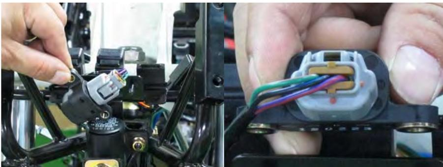
Incline the tilt switch  $65 \pm 10$  degrees to the left or right at the ignition switch "ON". Measure the voltage as below.
