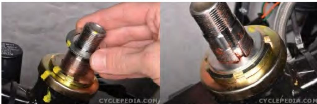
Slide the lock washer onto the steering stem as shown.
