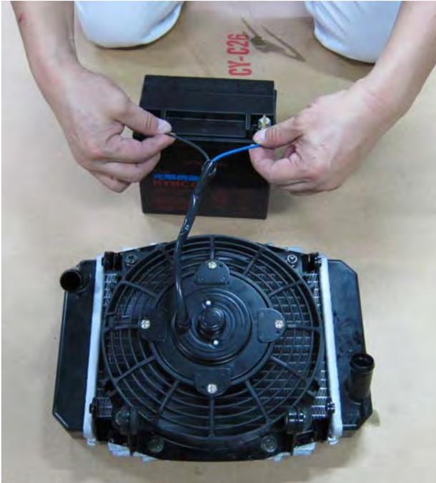
Jump a 12 volt battery to the fan connector and make sure the radiator fan operates.
