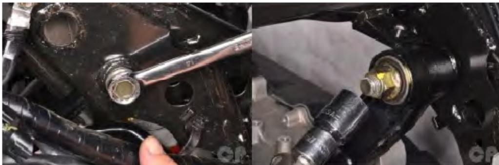
Hold the engine mounting bolts with a 14 mm wrench and loosen the nuts with a 19 mm socket.
