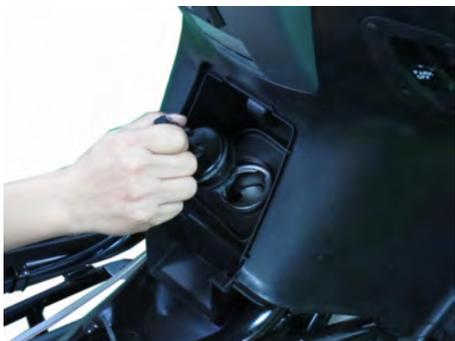
Install the gas cap overflow pad.
