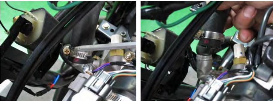
Loosen the thermostat hose clamp with a #2 Phillips screwdriver. Slide up the clamp and free the coolant hose from the thermostat.
