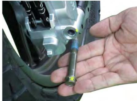
Remove the two caliper mounting bolts with a 12 mm socket.
