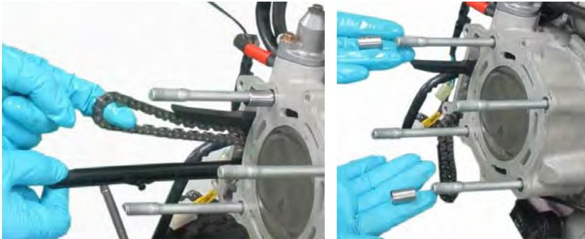
Slide out the lower cam chain guide. Inspect the guide for excessive wear and damage. Replace the guide as needed.
