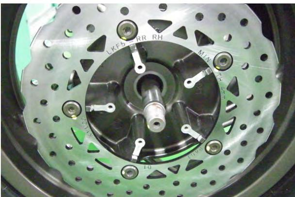
To remove the rear brake disc take out the five mounting bolts with a 6 mm Allen.
