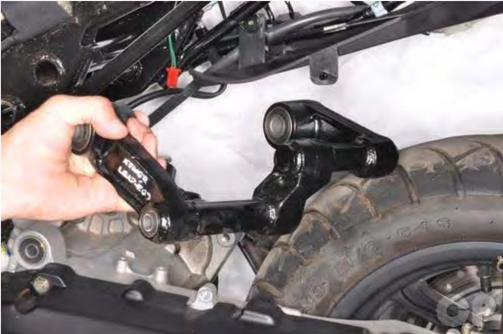
Remove the engine mounting bracket.
