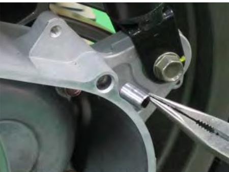
Remove the two dowel pins.
