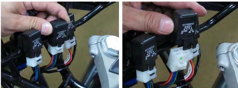
Remove and disconnect the high beam relay. The Low beam relay is on the left.
