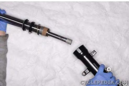
Separate the inner and outer fork tubes by pulling them apart using a slide hammer motion.
