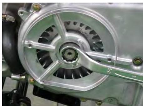
Install the drive pulley nut with a 24mm socket.
