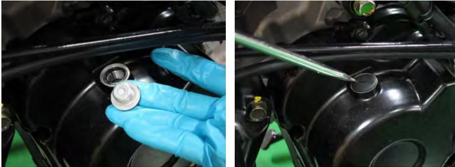
Make sure the O-rings on the timing plugs are in good condition. Replace it as needed. Install the timing inspection to the right side of the engine. Tighten the caps securely but not overly with a large flat blade screwdriver.
