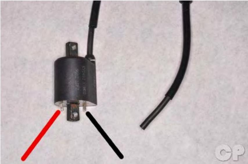
Touch the positive and negative meter leads to the ignition coil terminals as shown. Measure the resistance.
