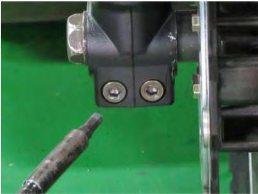
Tighten the front axle pinch bolt securely with a 6 mm Allen.
