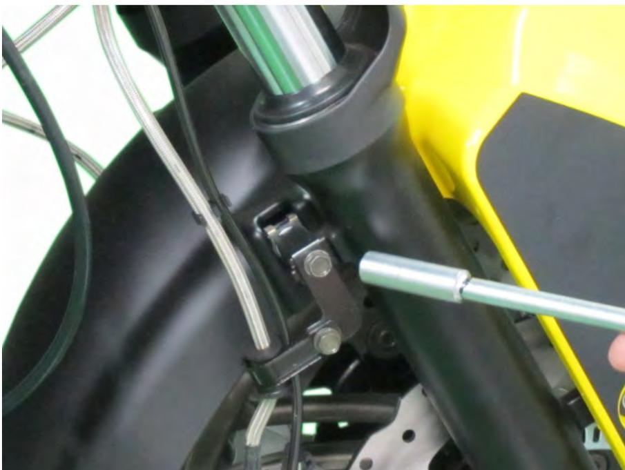
Remove the right forward front fender bolt with a 10 mm socket.
