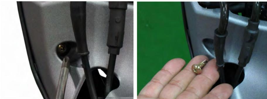
Remove the two upper handlebar cover screws with a #2 Phillips.
