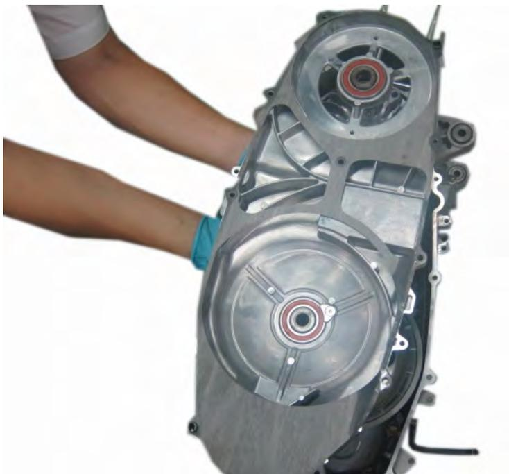
Inspect the belt case bearing by turning it with a finger.
