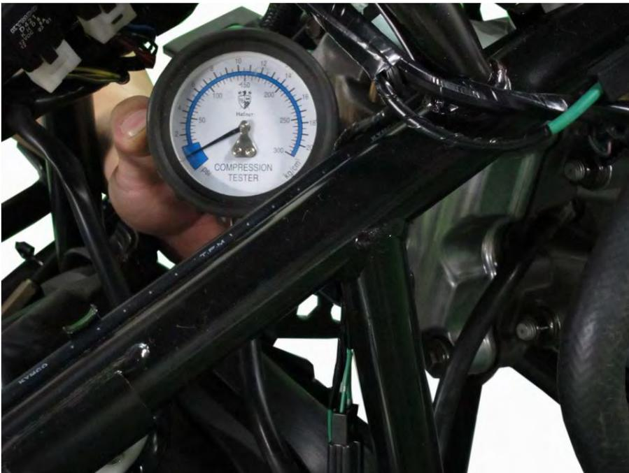
Thread a compression tester into the spark plug hole hand tight. Hold the throttle all the way open. Crank the engine with the starter motor until the needle on the gauge stops rising. Do not crank the engine more than a few seconds.
