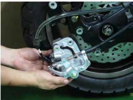
Remove the rear brake caliper from the rear fork.
