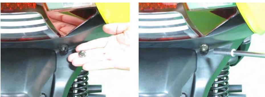
Install the two lower body cover nuts and tighten securely with a 10 mm socket.
