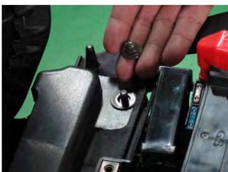
Remove the four luggage nuts with a 10 mm socket.
