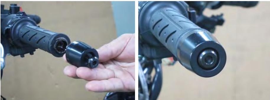
Install the bar ends with a 6 mm Allen.
