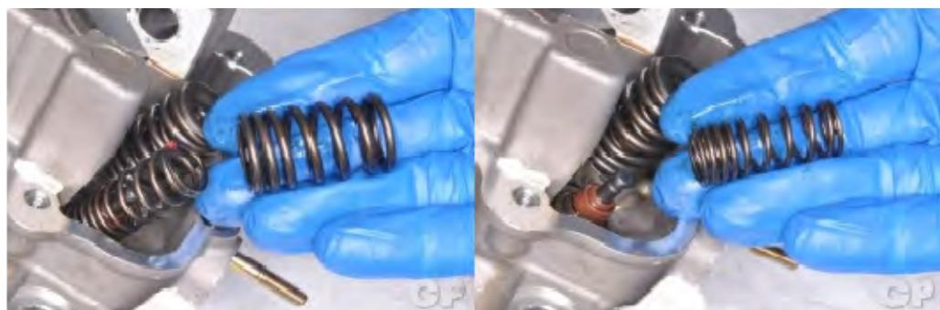
Remove the valve springs.
