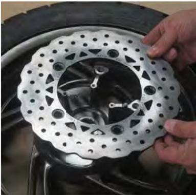
Lift off the rear brake disc.
