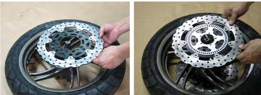
Remove the front brake discs.
