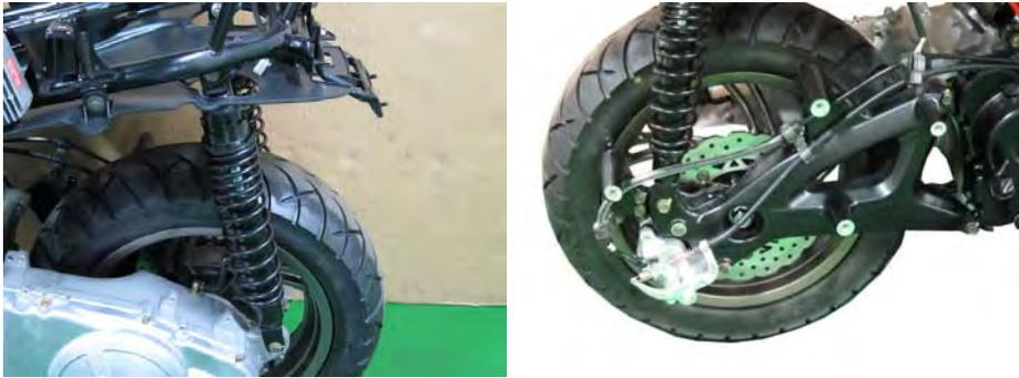
Install the lower shock absorber mounting bolts and torque them to specification with a 14 mm socket.
