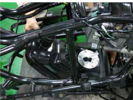
Fit the fuel tank into place.
