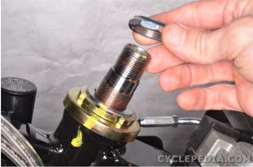
Thread the steering stem lock nut onto the steering stem.
