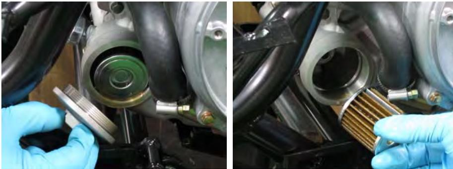
Remove the oil filter cap with spring and take out the used oil filter.
