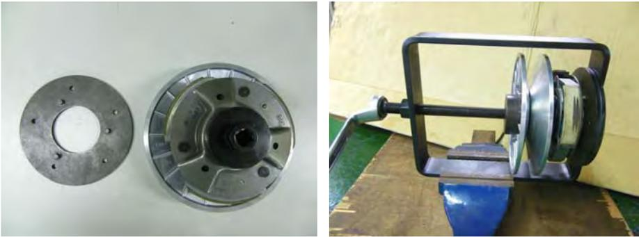
Use the clutch spring compressor tool to compress the spring in the driven pulley assembly.
