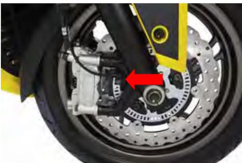
Install the speed sensor and its mounting bolt to the right fork leg. Tighten it securely with an 8 mm socket.
