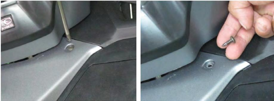
Remove the two screws below the handlebar.
