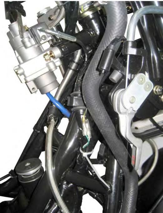
Remove the parking brake cable guide on the right side.
