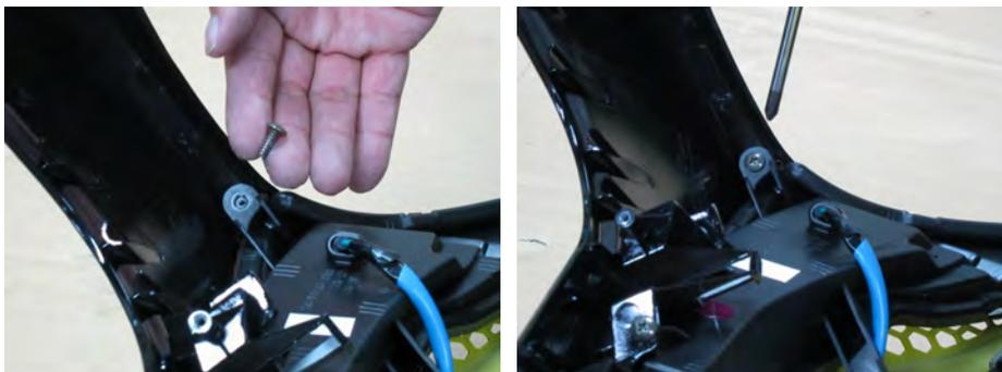
Install the ten front side skirt mounting screws with a #2 Phillips.
