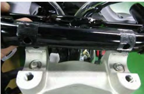
Install the handlebar onto the holders.
