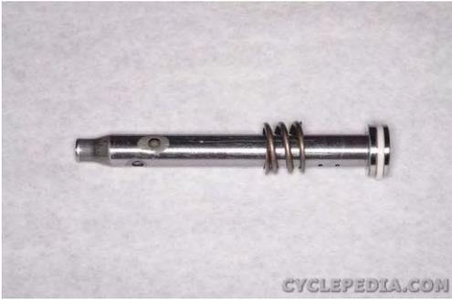
Remove the rebound spring from the damper rod. Inspect the damper rod seal ring and replace it as needed.
