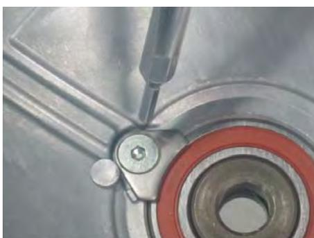
Install the bearing fixed plate with a 5 mm Allen
