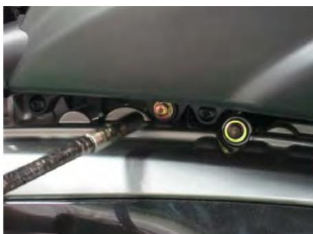
Install 2 the air cleaner bolts with an 8 mm socket.
