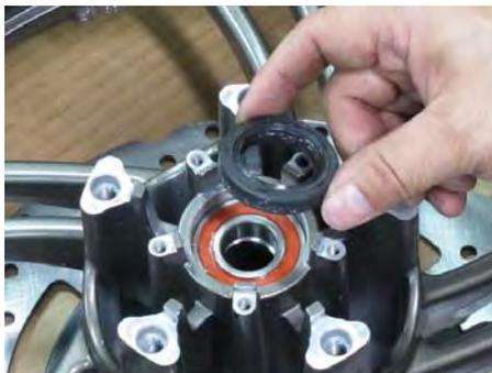
Remove the dust seals from the each side of the front wheel using a seal pick or large flat blade screwdriver. Discard the dust seal, it should be replaced by a new item.
