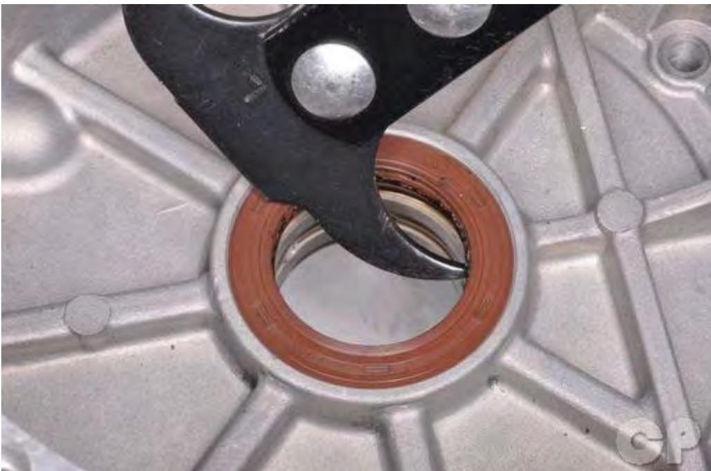
Remove the seal with a seal pick.
