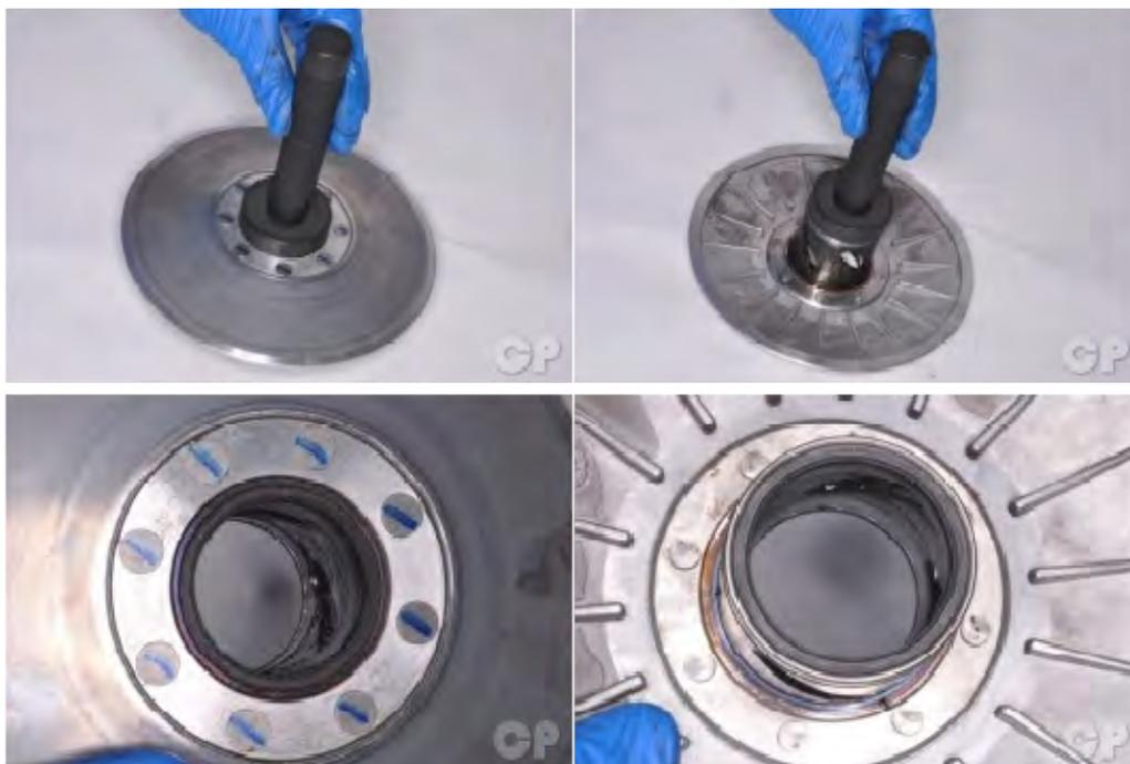
Drive in the new seals with a suitable driver with the same outside diameter as the seal.
