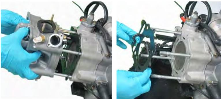
Remove the cylinder head assy and gasket.
