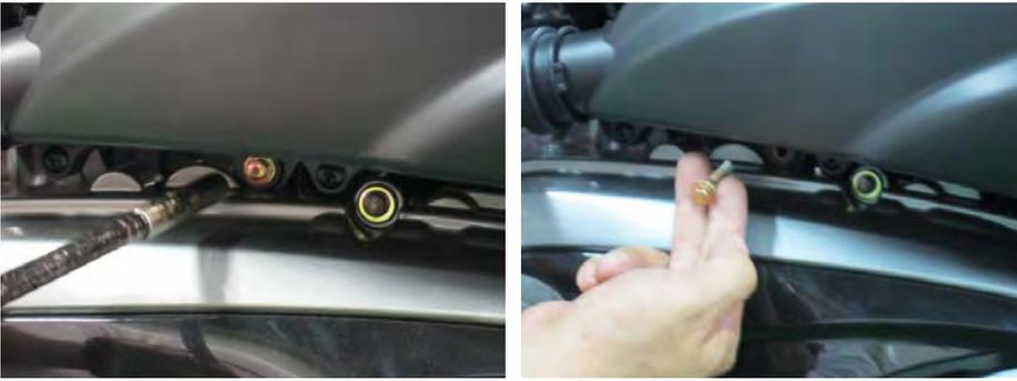
Remove 2 the air cleaner bolts with an 8 mm socket.
