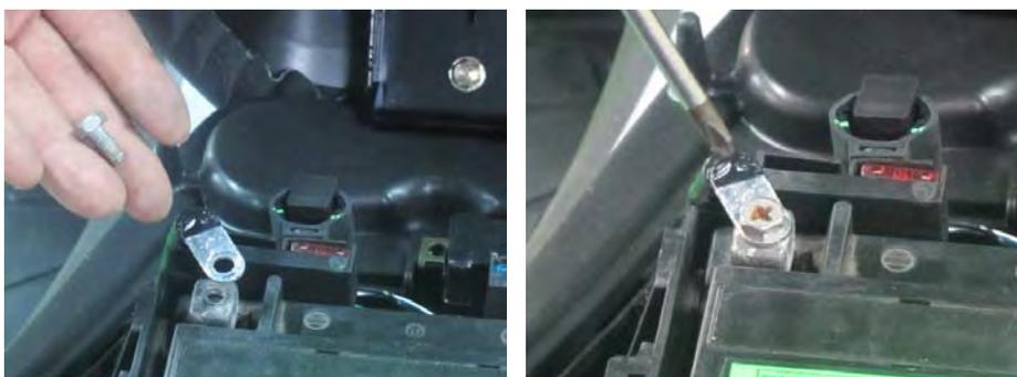
Connect the negative battery cable and install the bolt with a 10 mm socket or #3 Phillips screwdriver.
