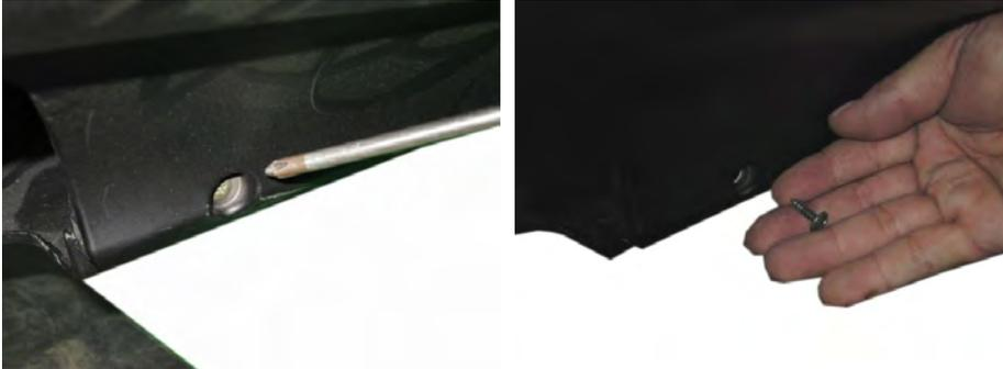
Remove the two under cover screws on both sides with a 10 mm socket.
