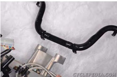
Remove the handlebar.
