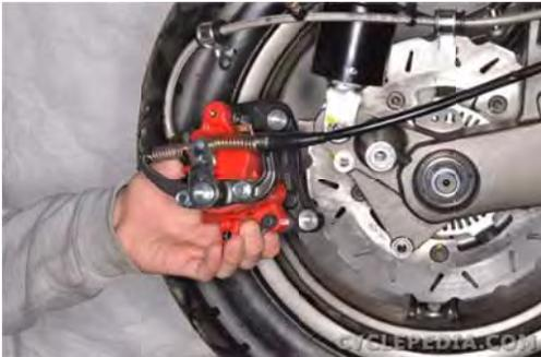
Fit the rear brake caliper into place. Insert two new mounting bolts.
