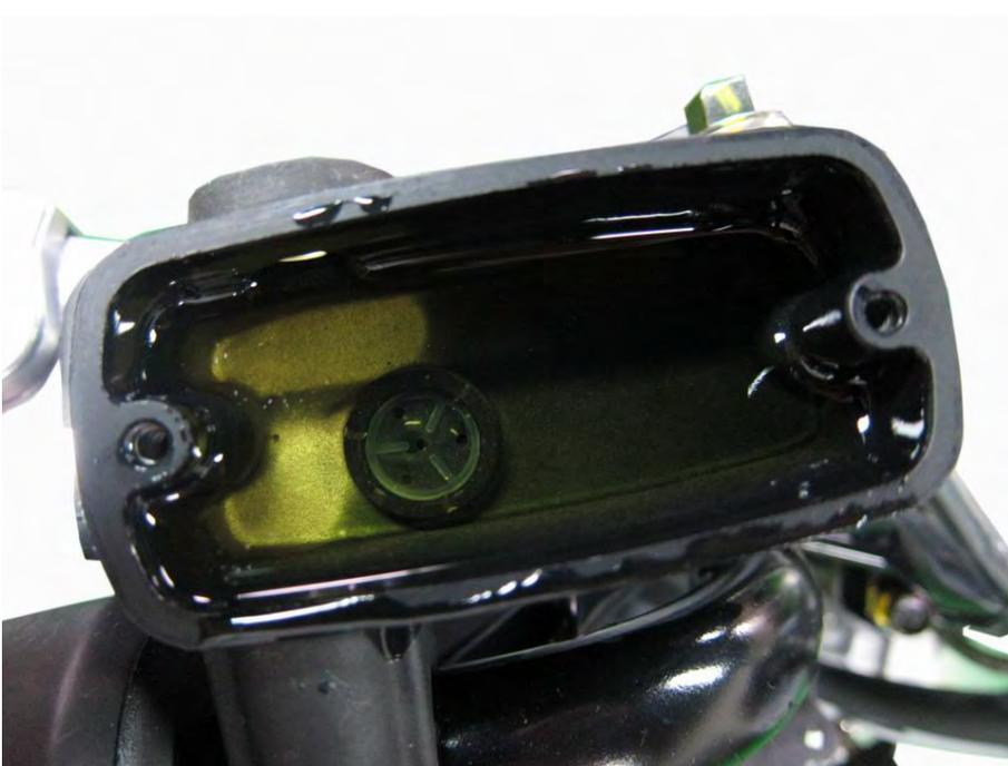
Fill the brake fluid with the proper type from a fresh, newly opened container.
