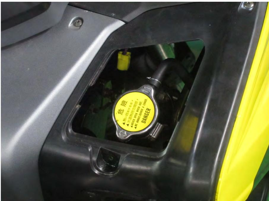
Install the radiator cap access panel.
