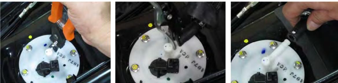
Loosen the fuel hose clamp with a special tool A120F00030. Slide back the clamp and free the injector fuel hose from the fuel pump pipe. Clean up any remaining fuel immediately.
