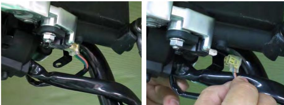
Unplug the brake light switch connectors.
