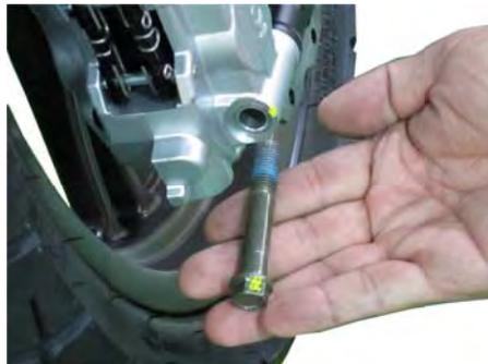
Remove the two caliper mounting bolts with a 12 mm socket. Discard the brake caliper mounting bolts.
