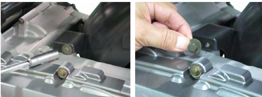
Remove the left fender mounting bolts with a 10 mm socket on the front side. Remove the airbox.
