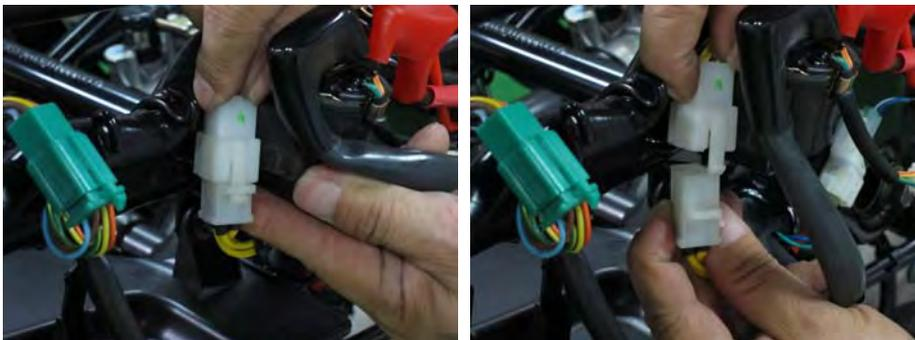
Plug in the regulator/rectifier 3-pin connector.
