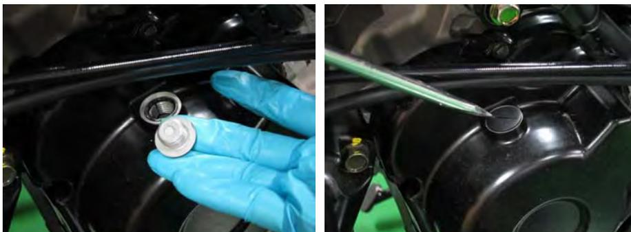
Make sure the O-ring on the timing plugs are in good condition. Replace it as needed. Install the timing inspection cap to the right side of the engine. Tighten the cap securely but not overly with a large flat blade screwdriver.
