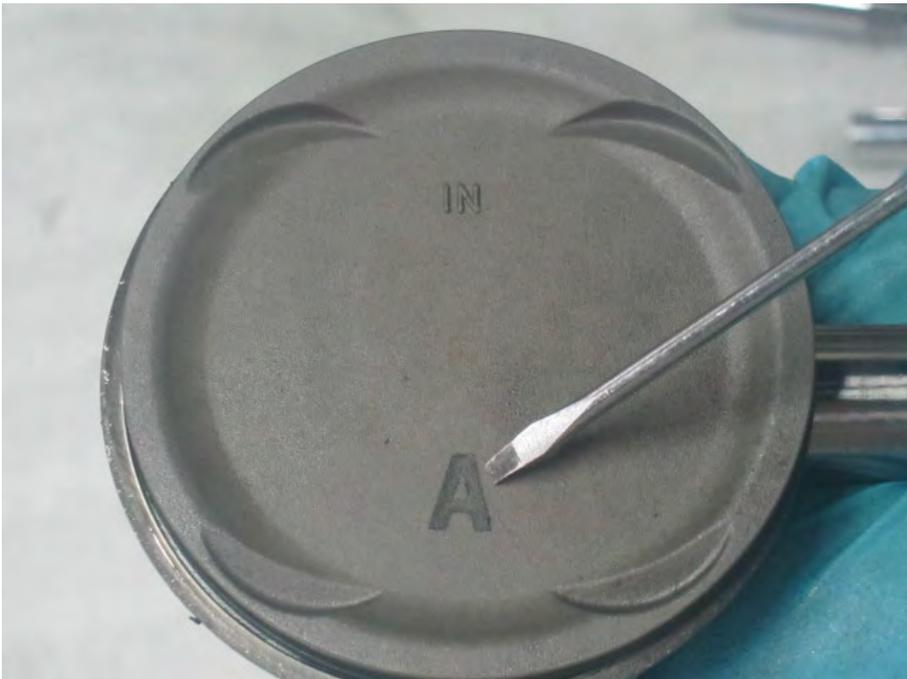
The "IN" mark should face the intake side (rear) of the engine.
