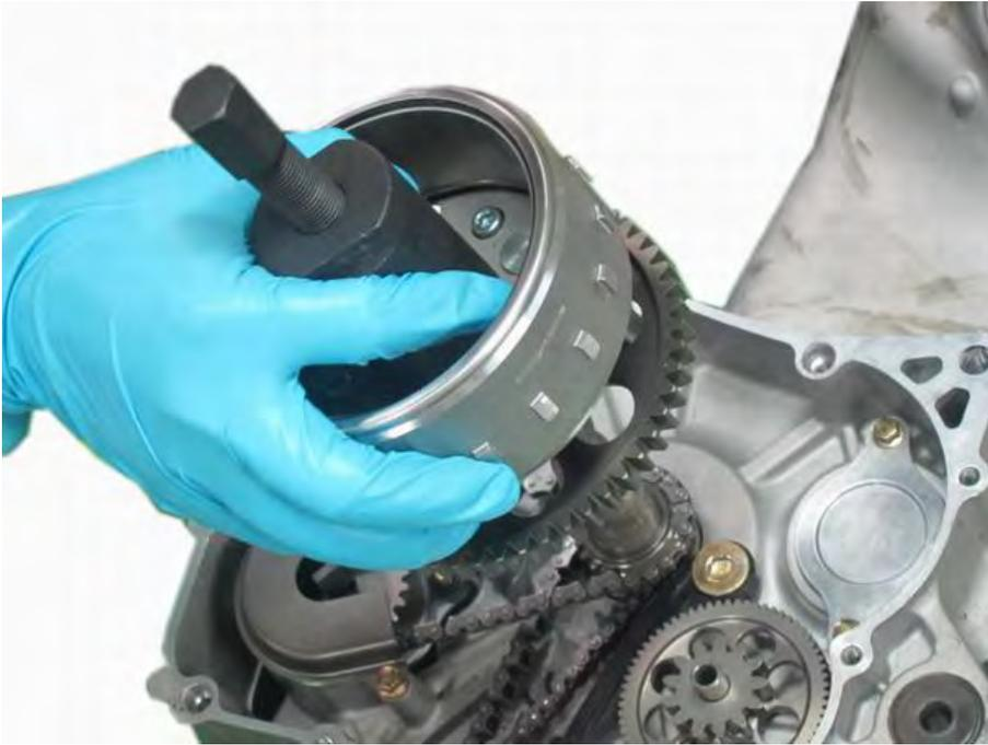
Line up the groove in the flywheel with the key and fit the flywheel onto the crankshaft. Guide the starter driven gear into the starter clutch on the back of the flywheel.
