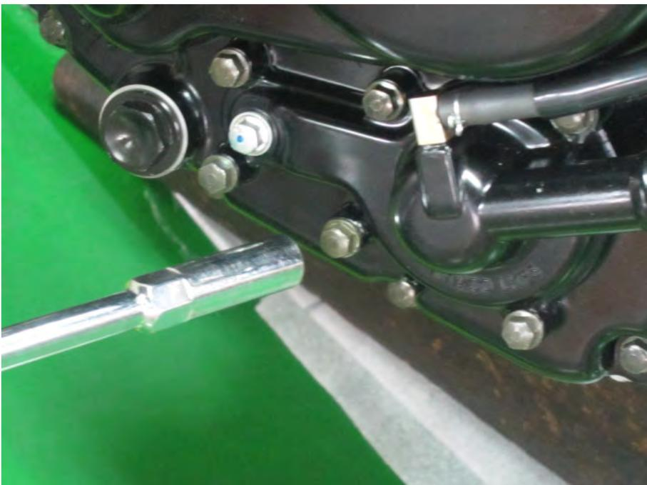
Loosen the four water pump cover bolts with an 8 mm socket.
