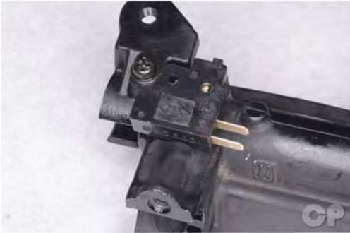
Install the brake light switch. Tighten the mounting screw securely with a #2 Phillips screwdriver.
