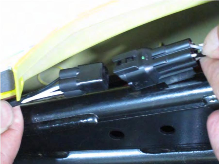
Measure the resistance between the white wire terminals of the O<sup>2</sup> sensor connector. Replace the O<sup>2</sup> sensor if the reading is out of specification.
