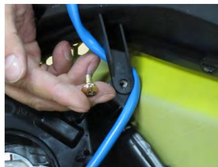
Remove the turn signal light assembly screws from the front cover.
