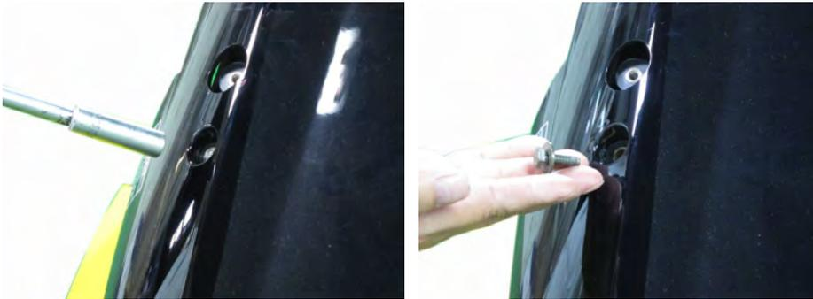
Remove the four windshield bolts with a 10mm socket.
