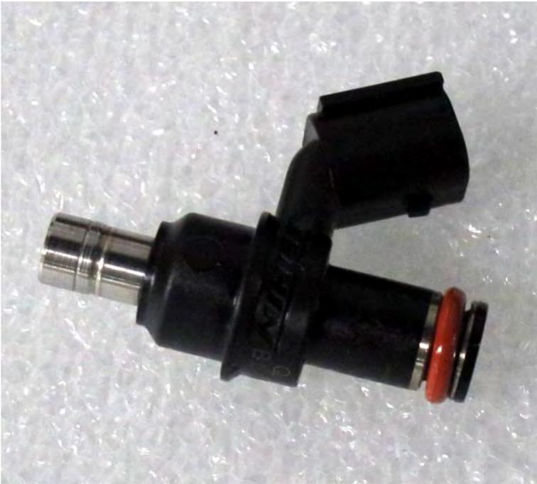
Inspect the seals on both sides of the fuel injector.
