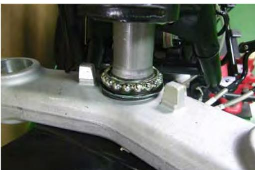
Slide the lower ball bearings up and off of the steering stem.
