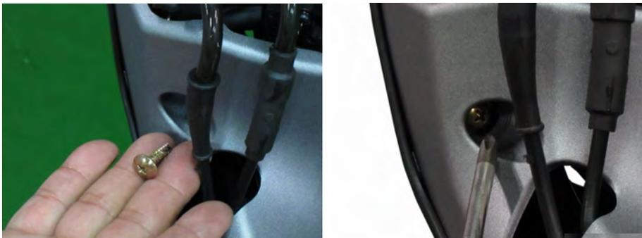
Install the two upper handlebar cover screws with a #2 Phillips.
