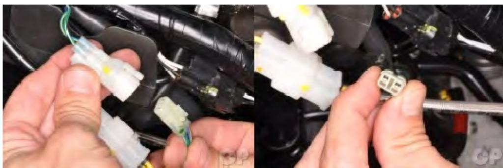
Disconnect the crank position sensor wire coupler.
