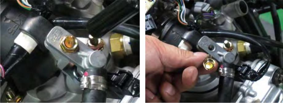
Remove the fuel injector mounting bolt with a 10 mm socket.
