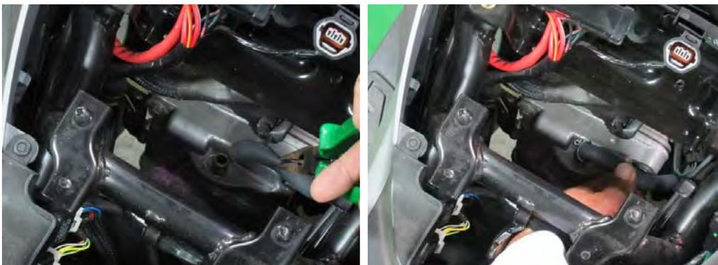
Squeeze the breather hose clamp with needle nose pliers and slide it back. Remove the breather hose from the cylinder head cover.
