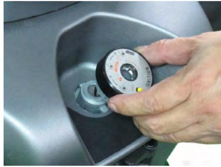
Remove the bolt mounting the ignition switch and then collar ignition switch.
