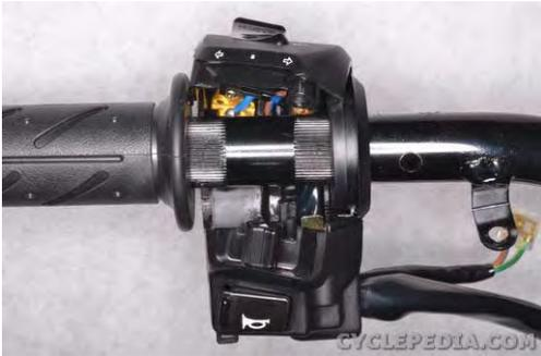
Separate the left switch housing from the handlebar.
