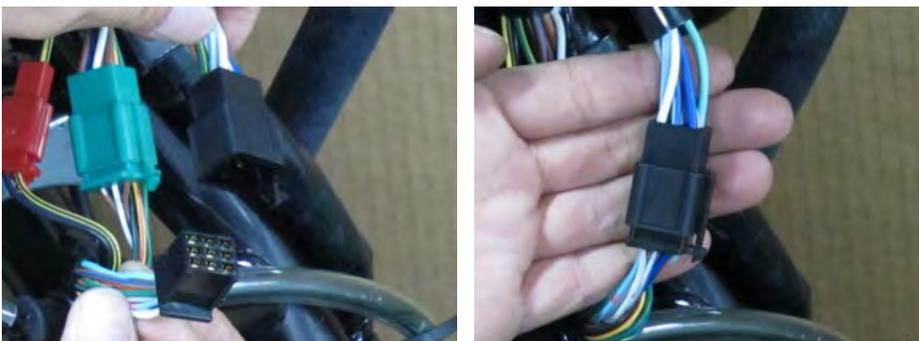
Plug in the black connector for the left handlebar switches.
