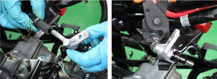
Fit the fuel hose onto the fuel injector pipe. Secure the hose to the fuel injector with the clamp. Tighten the clamp securely with a special tool A120F00030.
