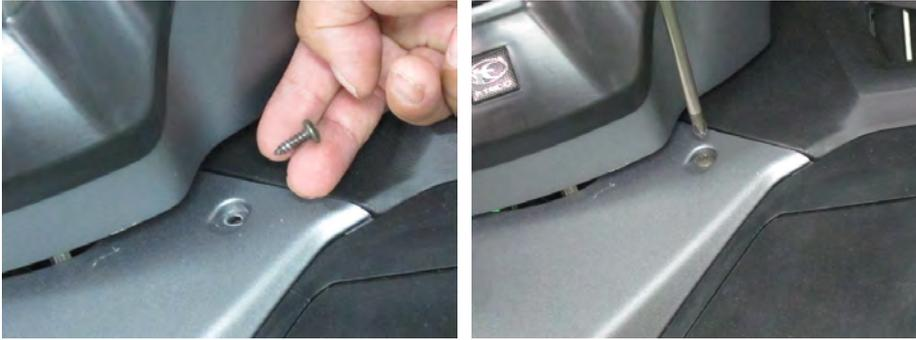
Install the two screws below the handlebar.
