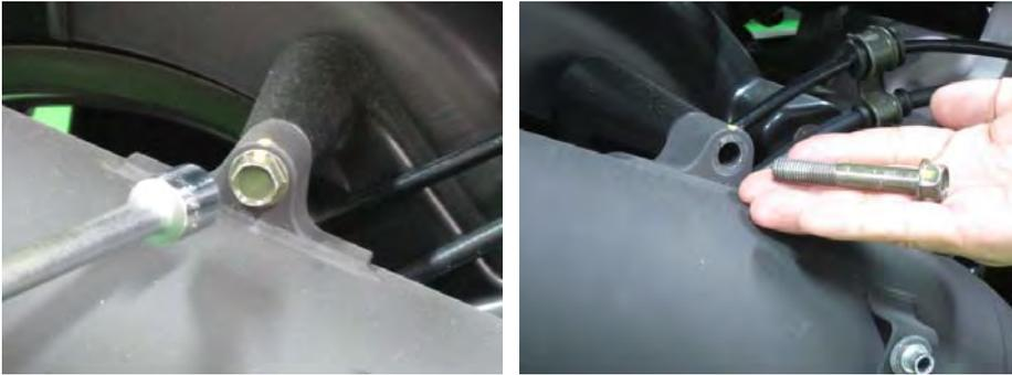
Remove the three muffler mounting bolts with a 14 mm socket.
