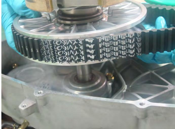
Remove the belt from the driven pulley.
