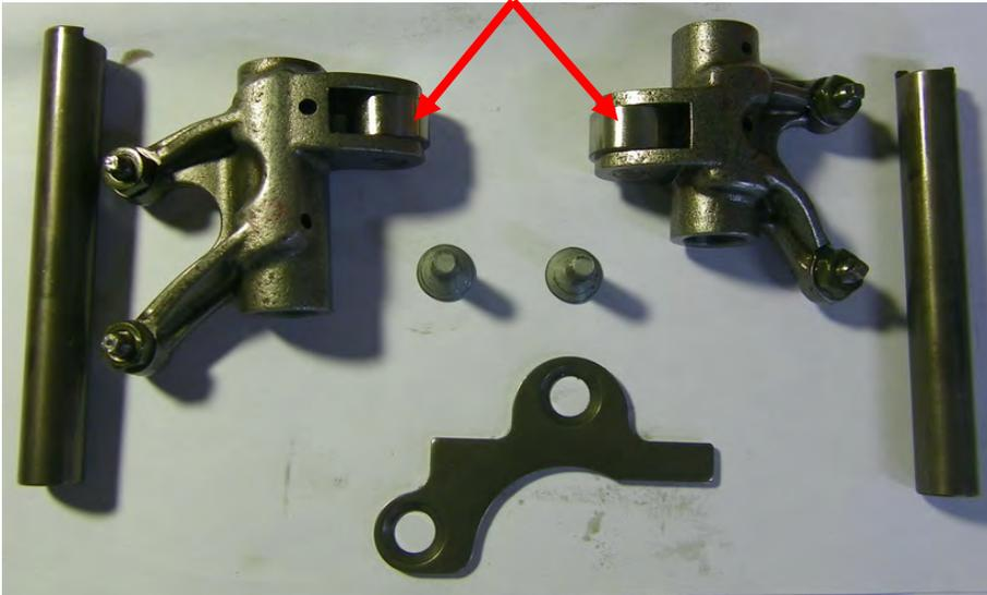
Inspect the rocker arm bearings for excessive play or roughness.
