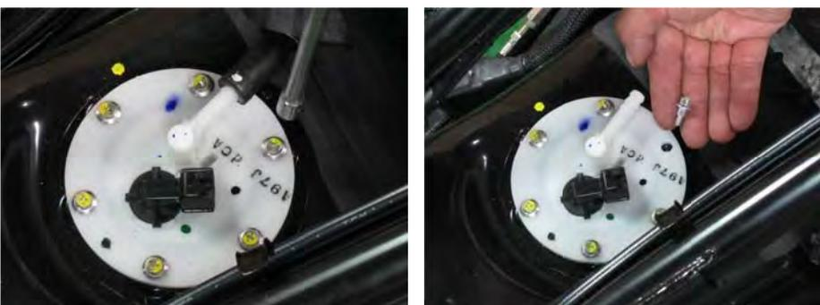
Remove the 6 fuel pump bolts with a 7 mm socket or #2 Phillips screwdriver.
