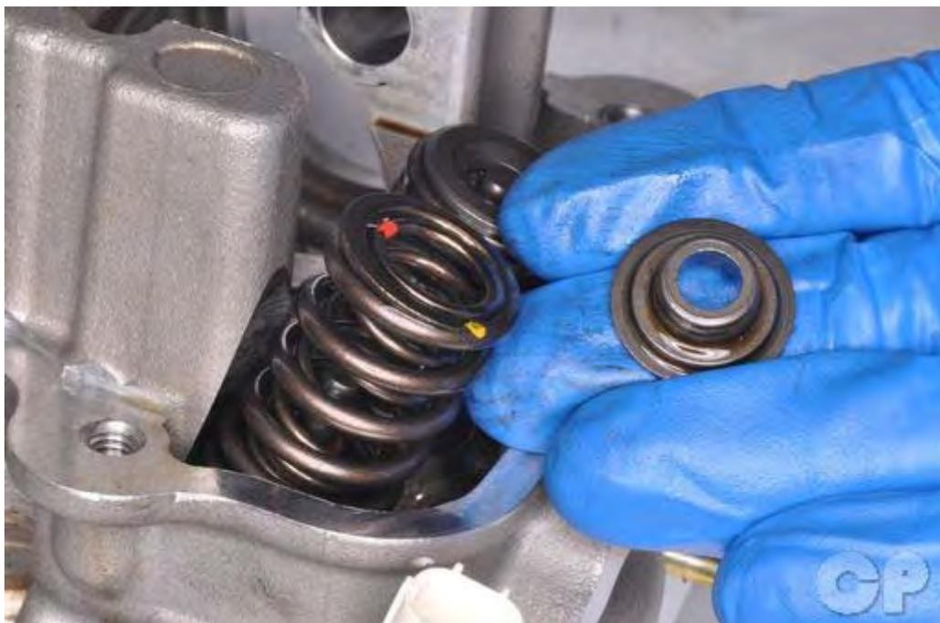
Remove the spring retainer.
