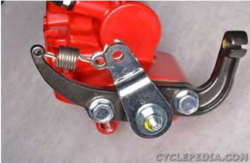
Loosen the parking brake lock nut with a 10 mm wrench.
