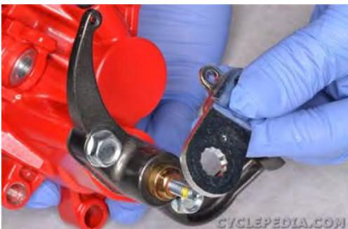
Free the parking brake return spring and remove the parking brake arm.
