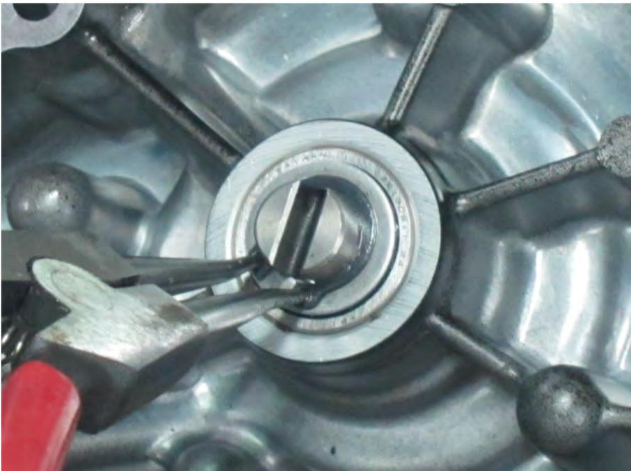
Lubricate the water pump shaft with fresh engine oil where it will ride in the case. Insert the water pump shaft into the generator cover from the inside.
