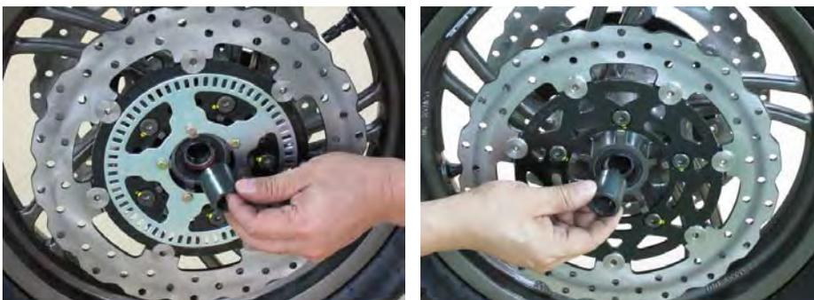
Apply grease to the lips of the dust seals and collar O-rings. Insert the collars into the hub as shown.
