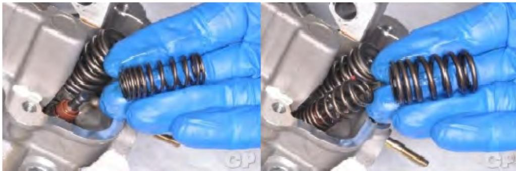
Install the valve springs. The tightly coiled end of the springs should sit against the spring seat.
