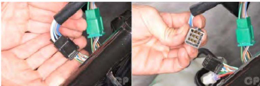
Unplug the black connector for the left handlebar switches.
