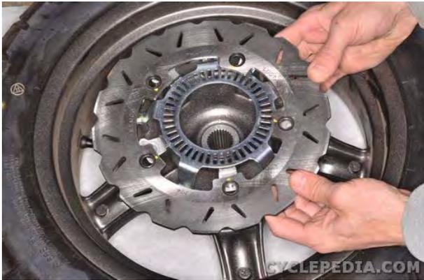
Lift off the rear brake disc.
