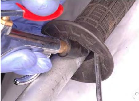
If you plan to replace the grips you can slice them lengthwise with a razor blade and peel them off. To remove the grips without cutting them use a screwdriver to open a gap between the grip and the handlebar. Spray in contact cleaner to break up the grip cement. Use compressed air to expand the grip so it can be easily slid off the end of the handlebar. Note the relationship between the angle of the grip and the throttle tube so that the new grip can be installed with the correct angle.
