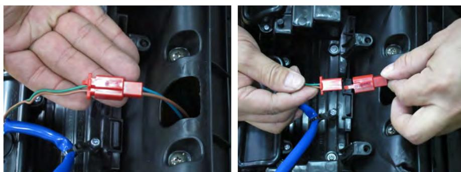
Disconnect the license light wires with the harness wires.
