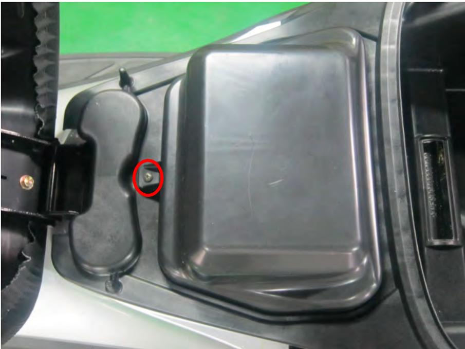
Remove the battery cover screw. Remove the battery cover.
