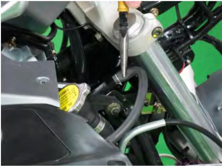
Install the bottom hose is the overflow hose that runs to the filler neck.
