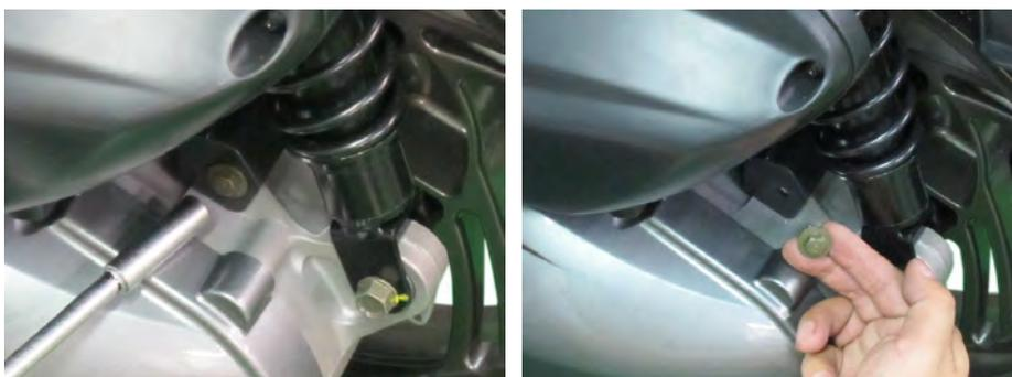
Remove the left fender mounting bolts with a 10 mm socket on the back side.
