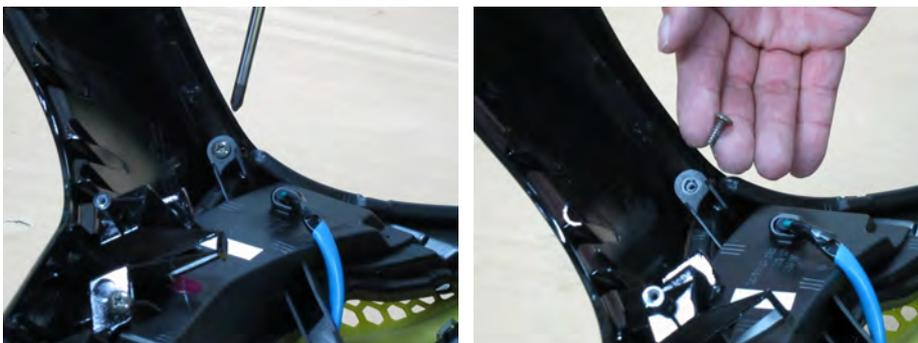
Remove the ten front side skirt mounting screws with a #2 Phillips.
