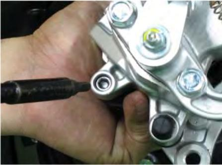
Loosen the brake pad pin with a 5 mm Allen.
