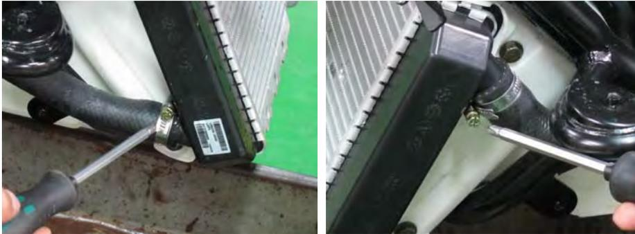
Remove the water pump and thermostat hoses in the same manner.
