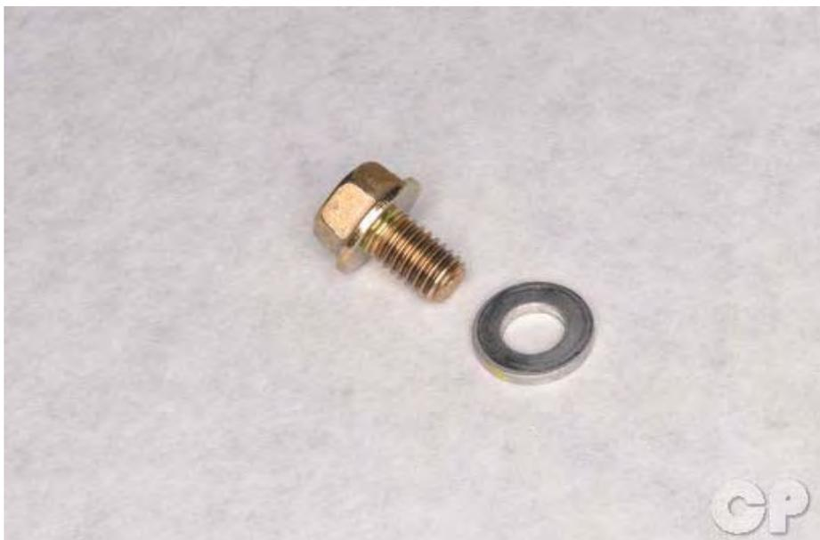
Inspect the drain plug and washer.
