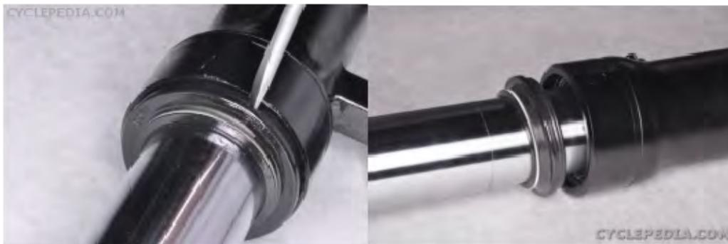
Use a flat blade screwdriver to pop the dust seal out of the fork slider. Take care to avoid scratching the fork tube.
