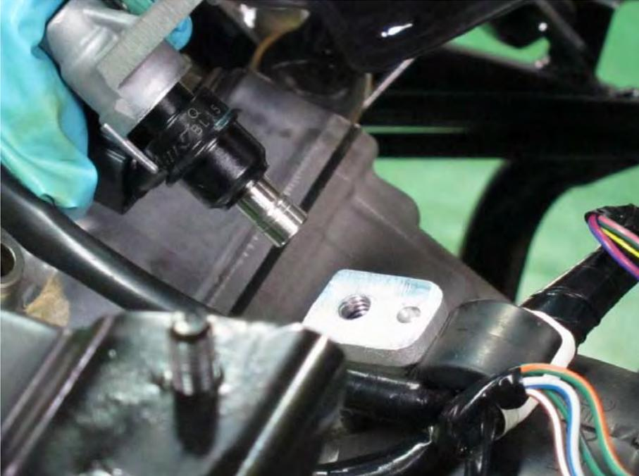
Fit the injector into the intake pipe as shown.
