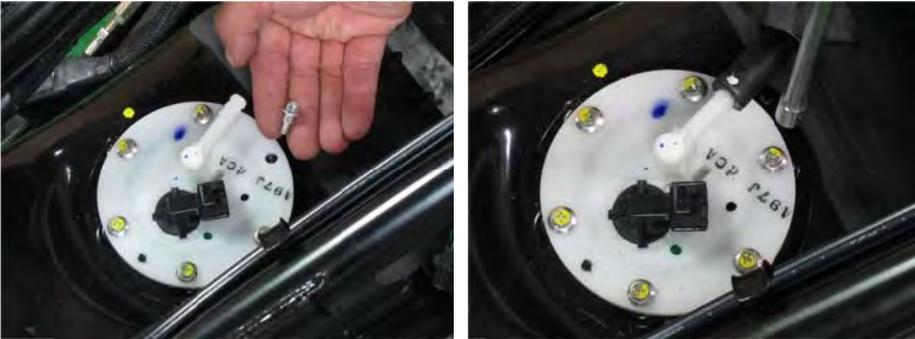
Insert the 6 fuel pump mounting bolts. Tighten the bolts to specification with a 7 mm socket or #2 Phillips screwdriver.
