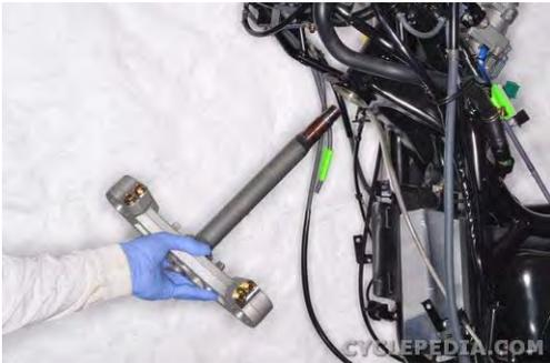
Lower the lower fork clamp and steering stem out of the frame.
