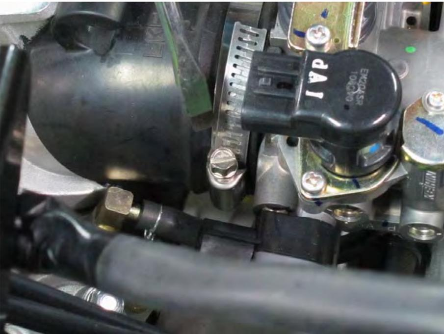
Tighten the intake hose clamp securely with a flat blade screwdriver.
