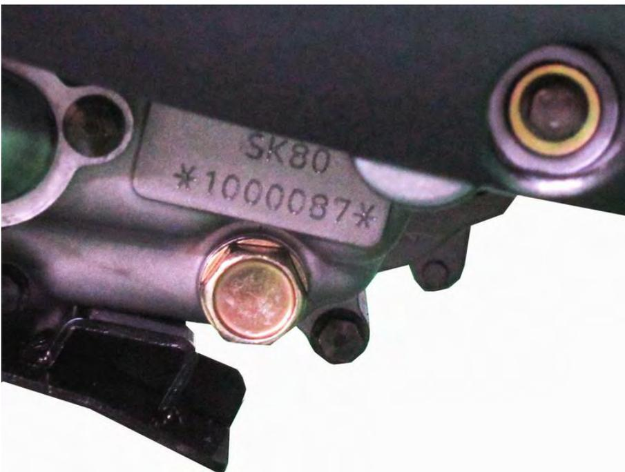
The engine serial number is stamped on bottom of the left crankcase.
