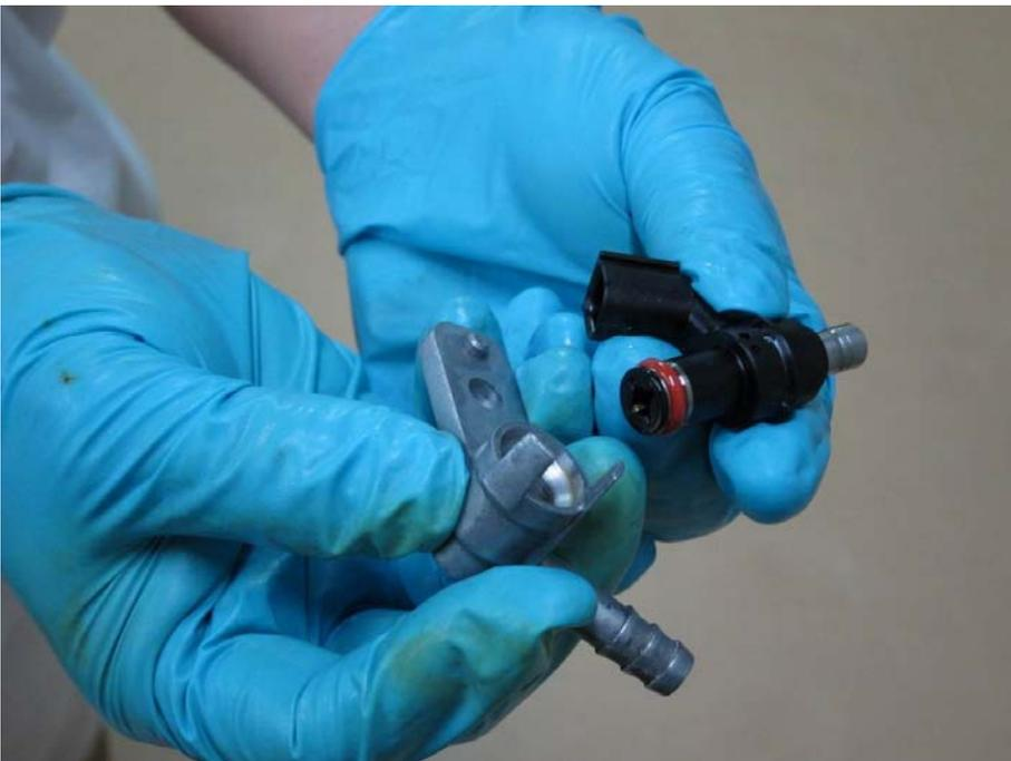
Fit the fuel injector pipe onto the top of the injector. The tab on the injector must fit into the pipe.
