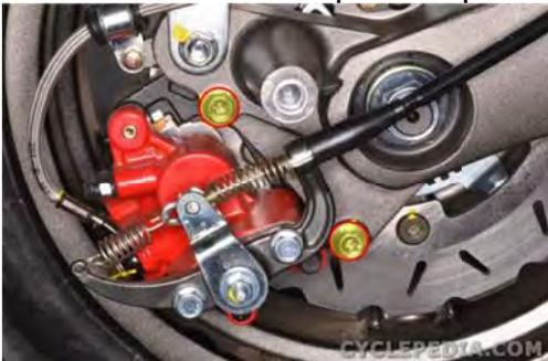
Torque the mounting bolts to specification with a 12 mm socket.
