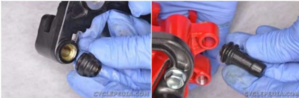
Install the caliper bracket pin boots.
