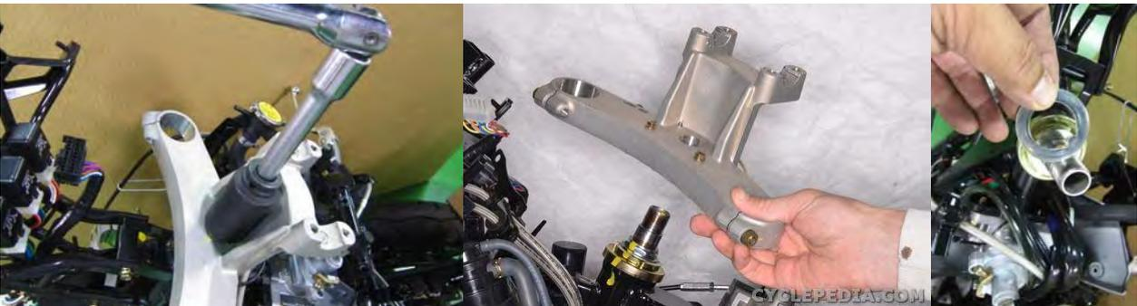
Remove the bridge stem nut and washer.
