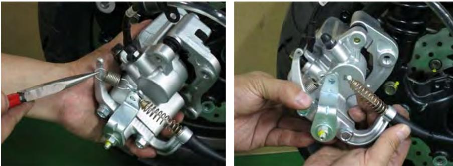
Free the parking brake cable from the rear brake caliper.
