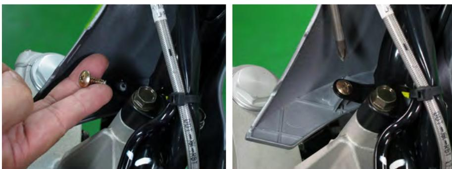
Install the two lower handlebar cover screws with a #2 Phillips.
