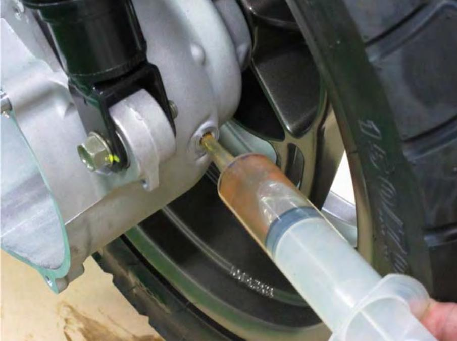
Fill the final drive oil with a syringe until oil begins to flow from the level check bolt hole.
