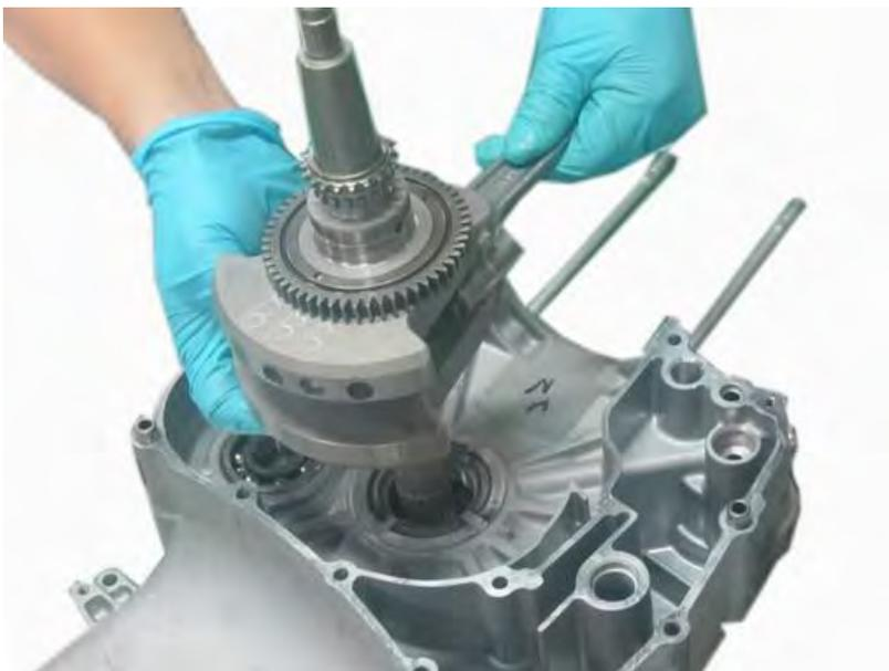
Fit the crankshaft into the left crankcase bearing. Take care to avoid damaging the new oil seal.
