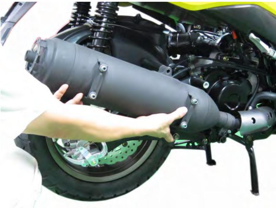
Fit the exhaust system into place
