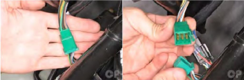
Unplug the green connector for the right handlebar switches.
