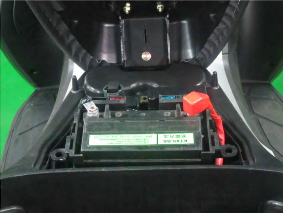
The battery is located under the seat.
