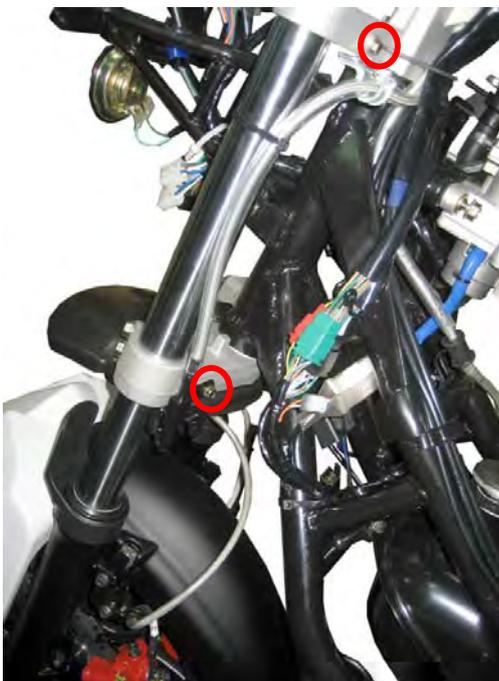
Remove the brake hose bracket on the left side of the lower fork clamp with an 8 mm socket.
