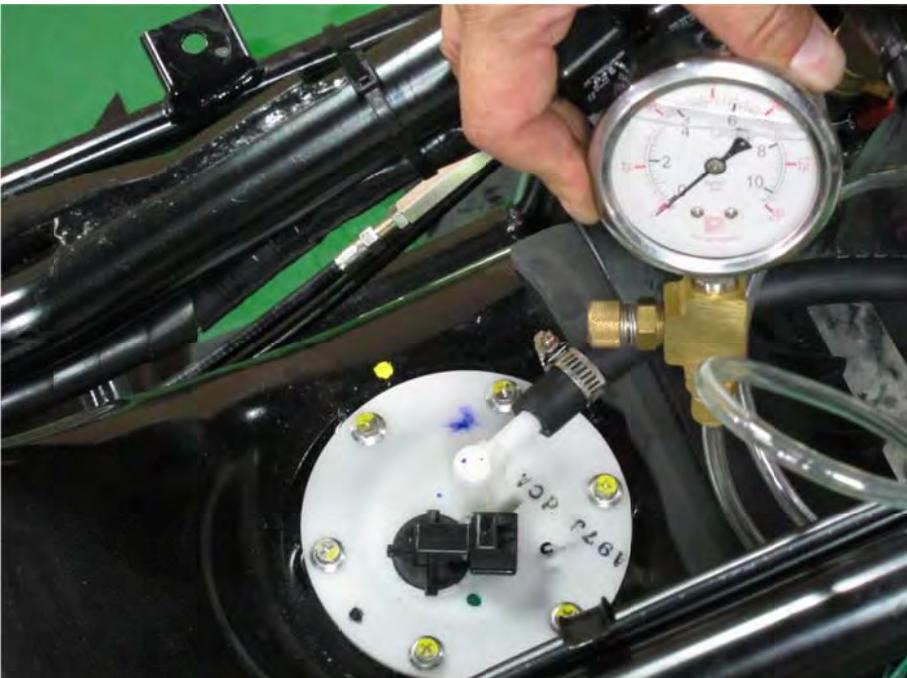
Disconnect the fuel hose from the fuel injector. Connect the fuel pressure gauge. Remove the fuel hose clamp. Turn the key to the ON position. Check the fuel pressure.
