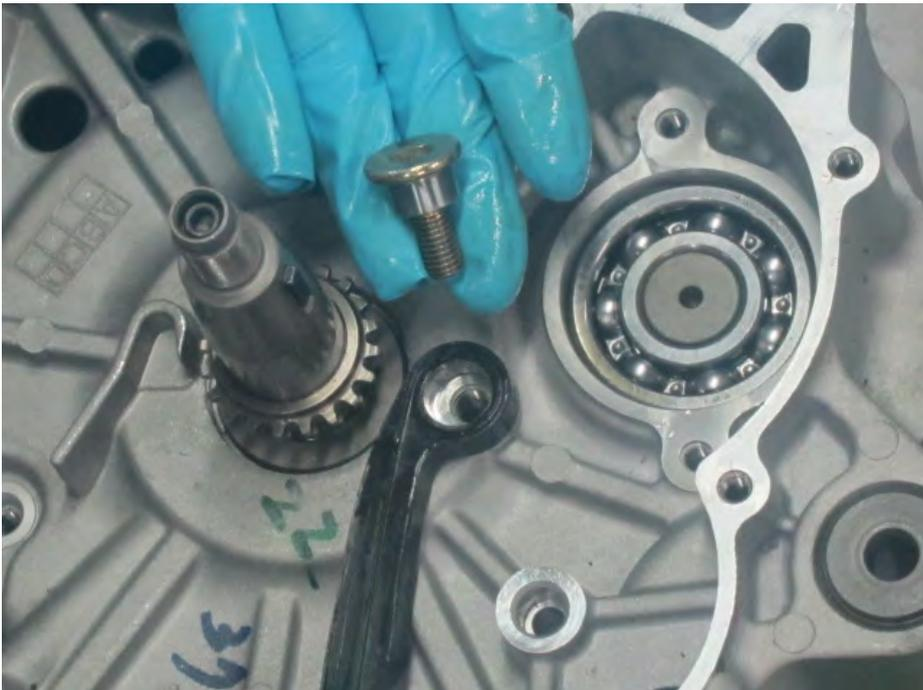
Remove the upper cam chain guide.
