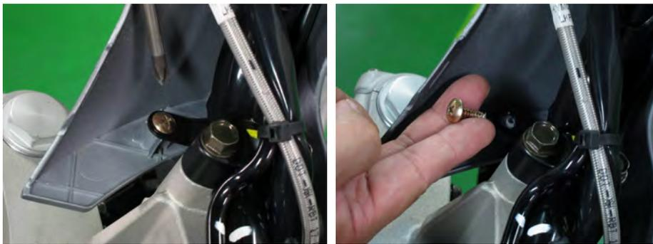
Remove the two lower handlebar cover screws with a #2 Phillips.
