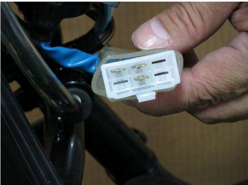
Use a digital multimeter to check for continuity to inspect the ignition switches. Continuity should exist between the wires as indicated.
