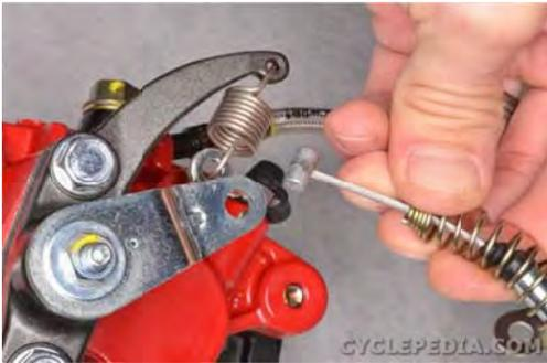
Connect the parking brake cable to the parking brake arm.
