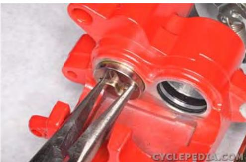
The parking brake piston must be unscrewed to be removed. Use a pair of needle nose pliers as shown to unscrew the parking brake piston.
