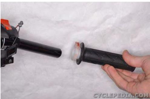
Slide the throttle tube and right switch housing off of the handlebar.
