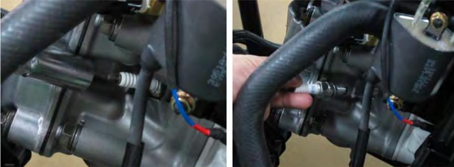
Remove the spark plug with a spark plug with a 5/8 in socket.
