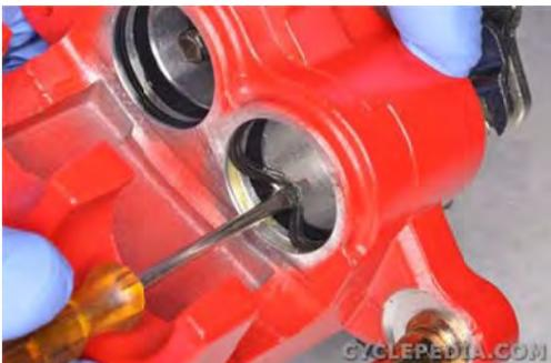
Remove the seals with a mechanics pick. Discard the old seals.
