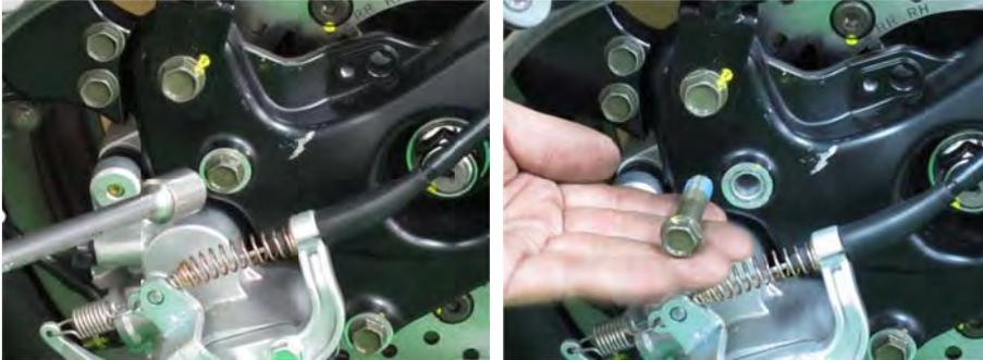
Remove the two rear caliper mounting bolts with a 12 mm socket.
