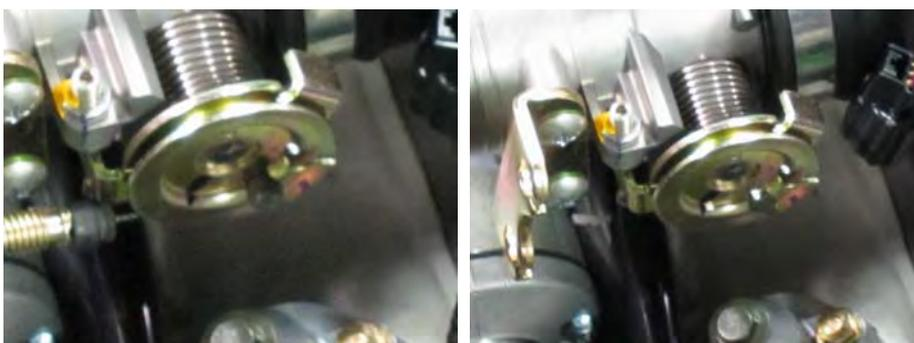
Free the throttle cables from the throttle drum.
