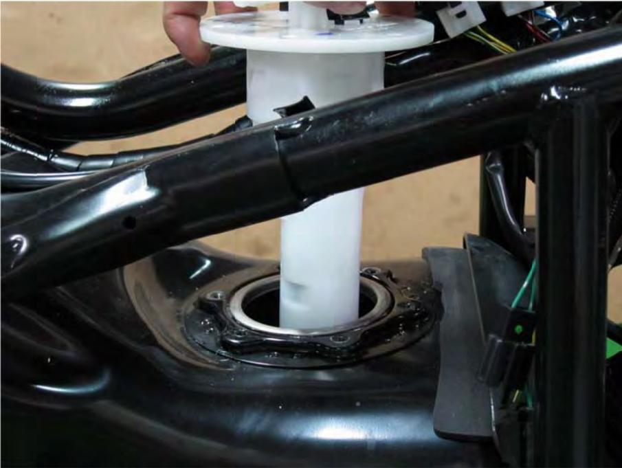
Lift the fuel pump out of the tank.
