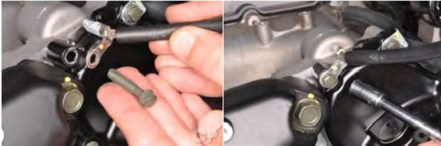
Install the main engine ground to the right side of the engine.
