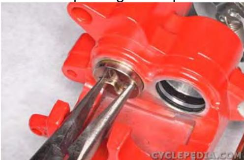
Turn the parking brake caliper piston clockwise to thread it into place.
