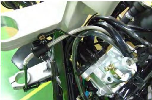
Route the throttle cables and handlebar switch wires down the back side of the upper fork clamp as shown. Install the wire and cable guide. Tighten the two cable guide bolts securely with an 8 mm socket.
