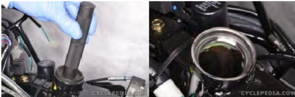
Drive the new bearing races into the steering head with a suitable driver with the same outside diameter as the bearing race.
