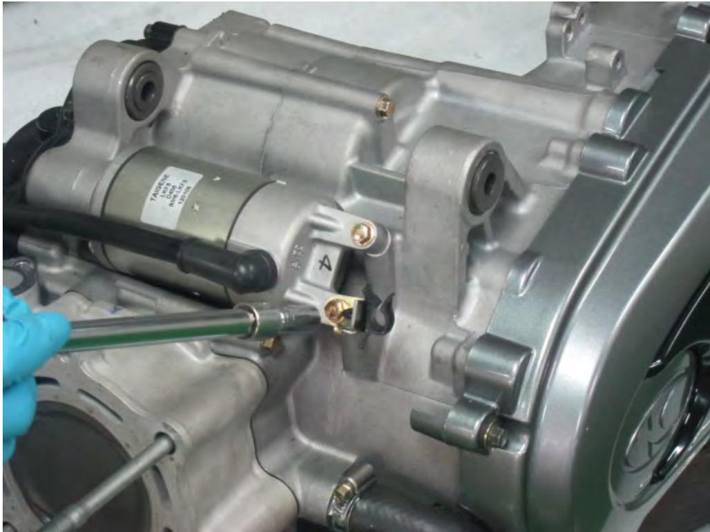
Fit the starter motor cable lead onto the terminal and thread on the nut. Tighten the starter motor lead nut securely with a 10 mm wrench.
