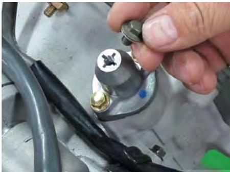
Make sure the cam chain tensioner cap bolt washer is in good condition. Install the washer and cam chain tensioner cap bolt. Tighten the bolt to securely with a 10 mm socket. Check the valve clearance.
