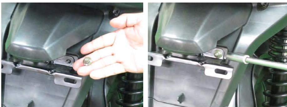
Install the two license plate nuts with a 10 mm socket.
