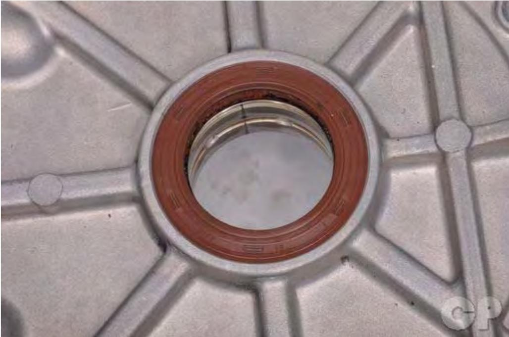
Replace the left crankshaft seal if the crankcases are separated.
