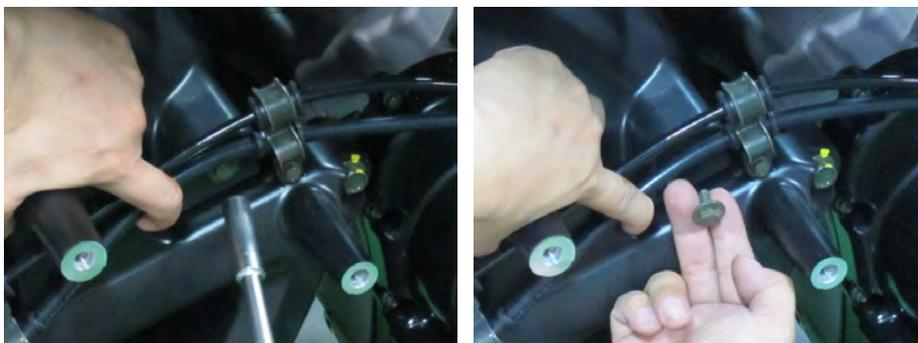
Remove the two right fender mounting bolts with a 10 mm socket.
