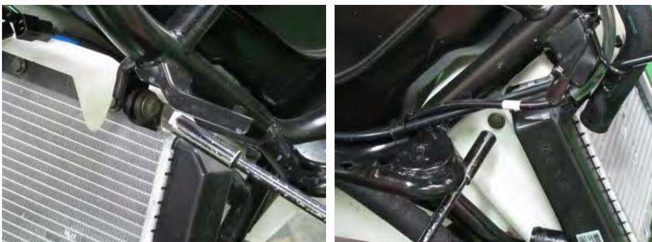
Remove the two radiator upper mounting bolts with a 10 mm socket.
