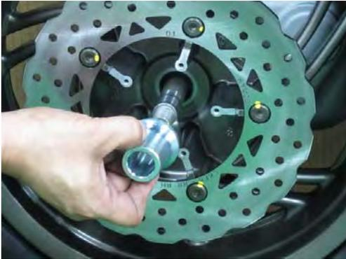
Apply grease to the lips of the dust seal and install the collar into the rear fork.
