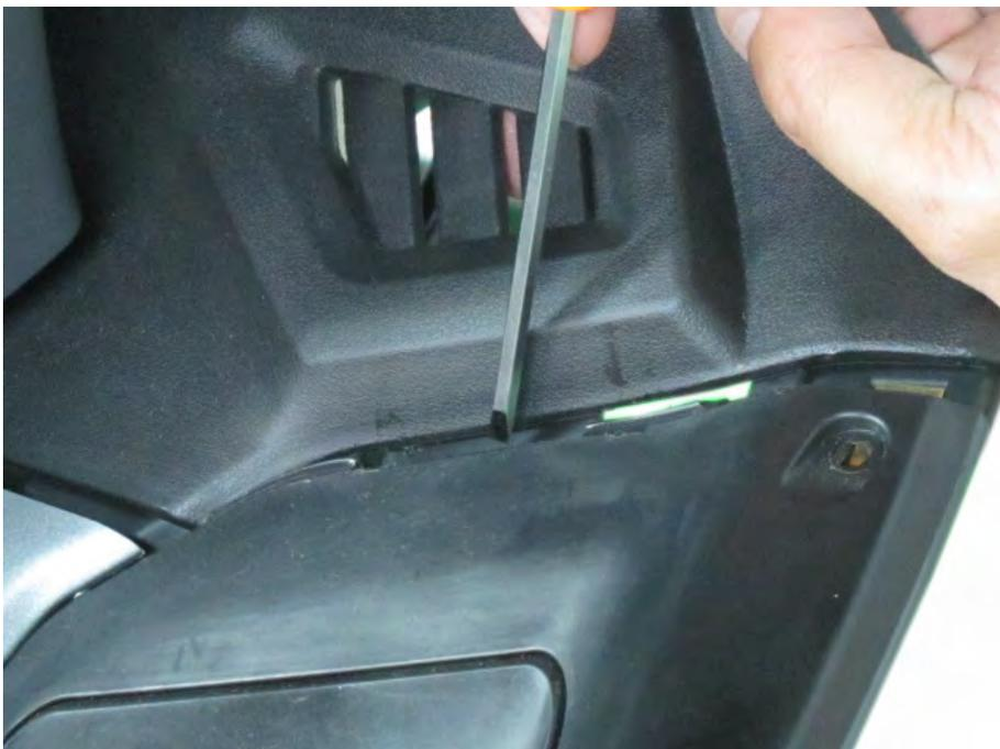
Gently separate the inner cover from the meter cover and free the tabs.
