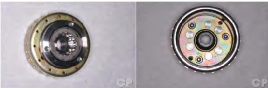
Fit the starter clutch to the back of the flywheel. Apply blue Loctite to the threads of the three starter clutch mounting bolts. Insert the three starter clutch mounting bolts.
