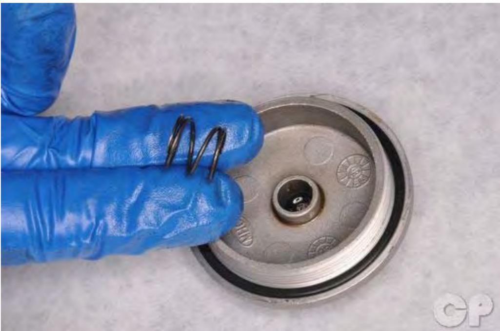
Install the spring to the oil filter cap. Apply a light coat of engine oil to the oil filter cap O-ring.
