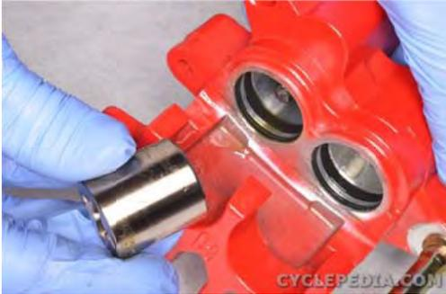
Remove the parking brake piston.
