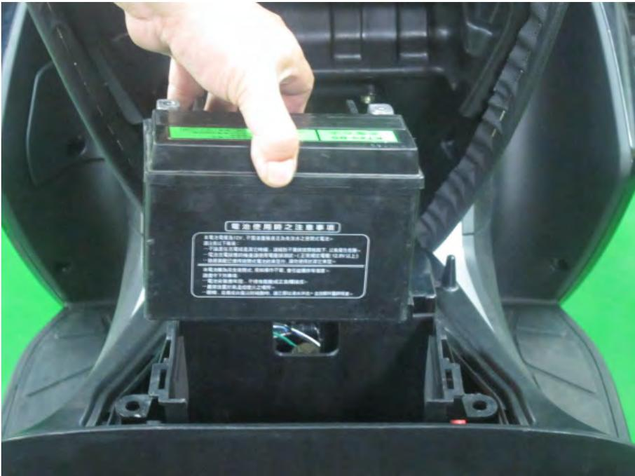
Fit the battery into the battery tray.
