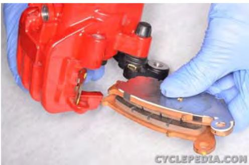
Fit the brake pads into place.
