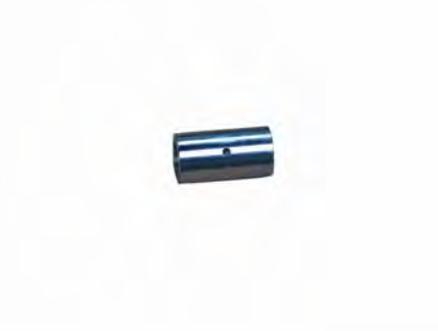
Inspect the movable drive face and bushing for wear and damage. Replace the parts as needed.
