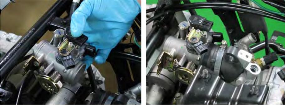
Fit the throttle body into the air box and intake boots.
