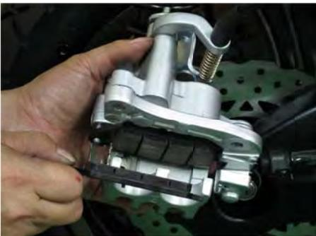
Free the brake pads from the pad retainer.
