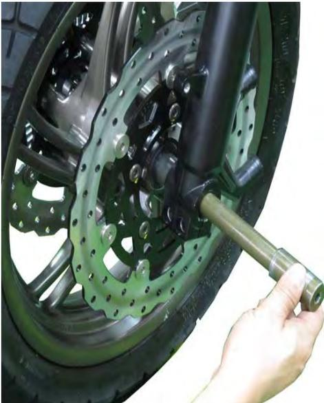
Apply a light coat of grease to the front axle. Insert the axle from the left side. Set the front wheel on the ground. Pump the front suspension up and down several times to seat the front axle.
