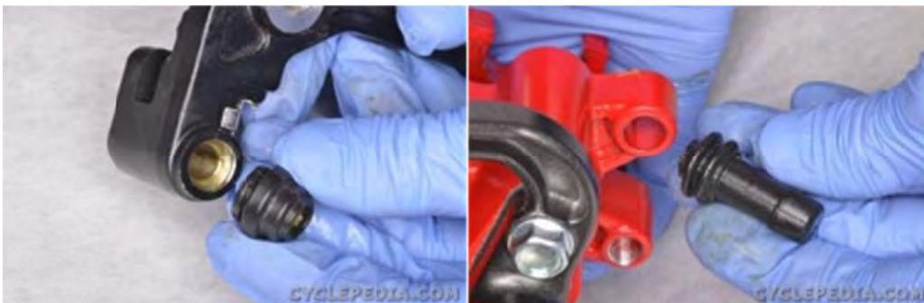
Remove the caliper bracket pin boots and inspect them for damage and deterioration. Replace the boots as needed.
