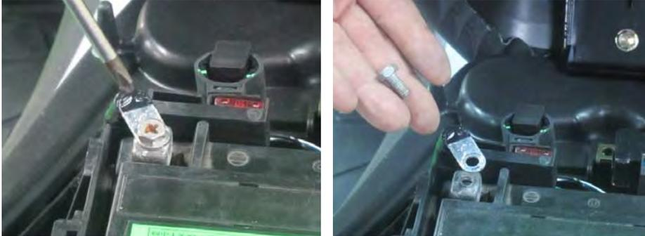
Remove the negative battery cable bolt with a 10 mm socket or #3 Phillips screwdriver. Free the negative cable from the battery.
