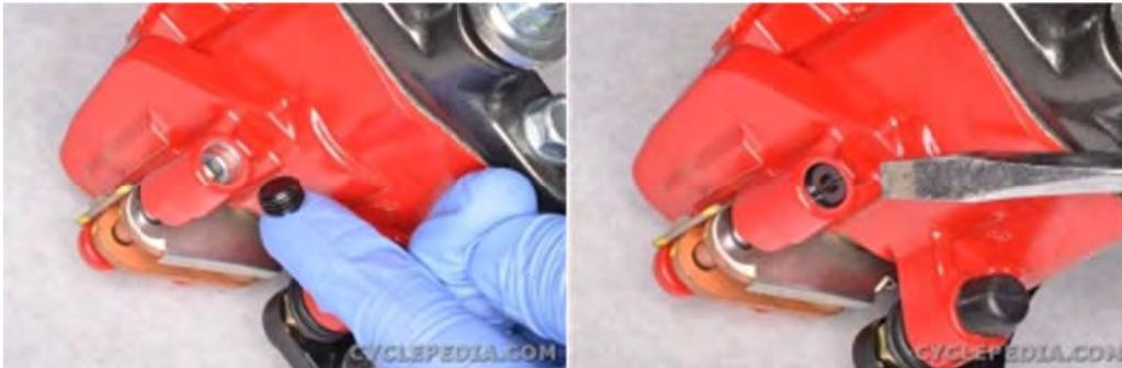
Install the brake pad pin plug and tighten it to specification with a flat blade screwdriver.
