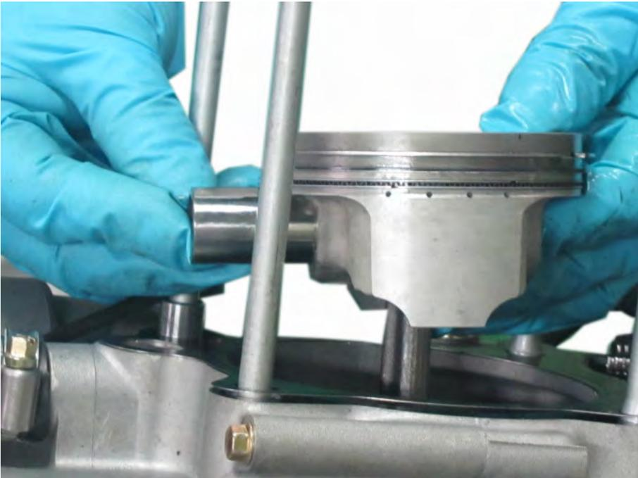
Remove the piston pin and the piston.
