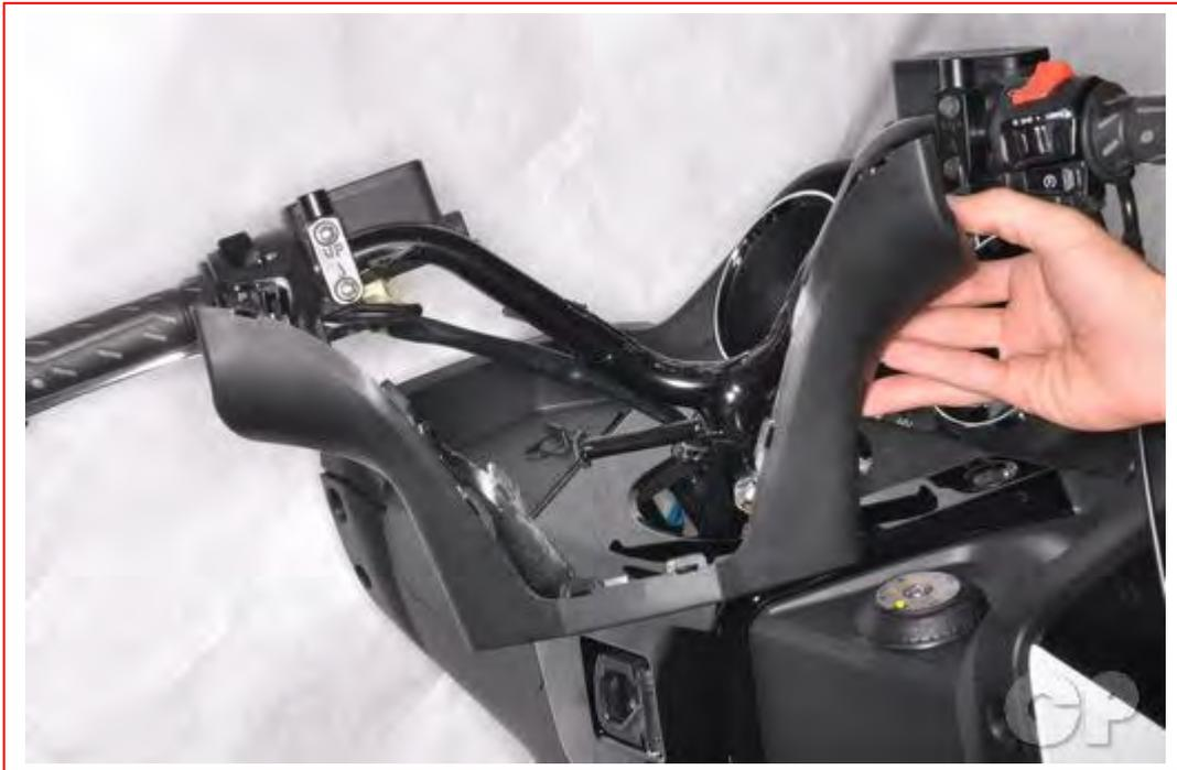
Place the lower cover onto the handlebar.
