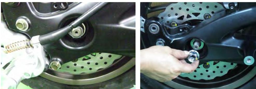
Remove the rear axle nut with a 27 mm socket.
