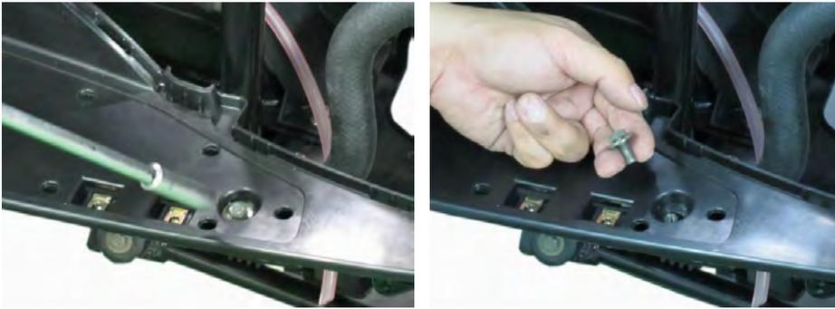
Remove the three mounting bolts on left side with a 10 mm socket.
