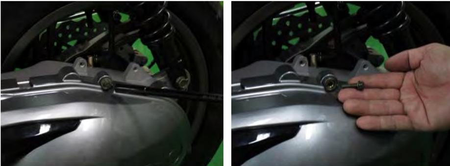
Remove 6 the belt case plastic cover bolts with an 8 mm socket.
