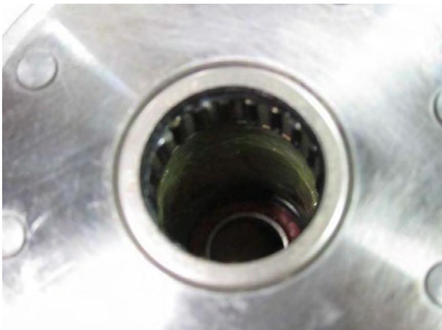
Lubricate the bearings in the right face of the driven pulley with grease.
