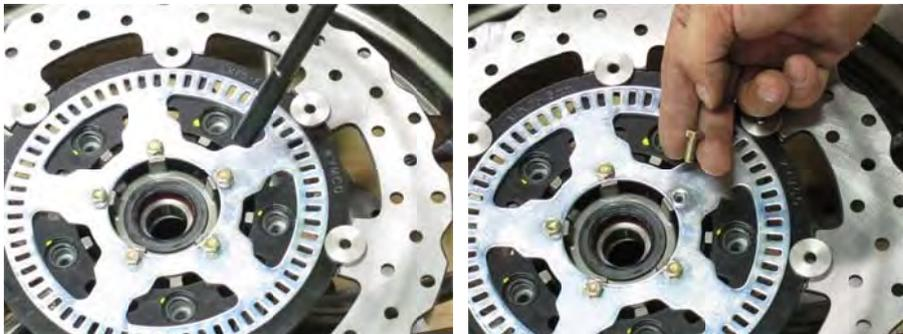
To remove the front brake disc take out the five mounting bolts with a 8 mm Allen.
