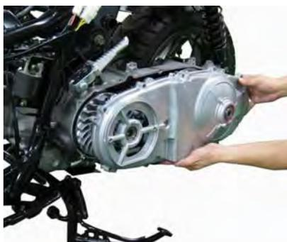
Install a new gasket with the belt case cover.
