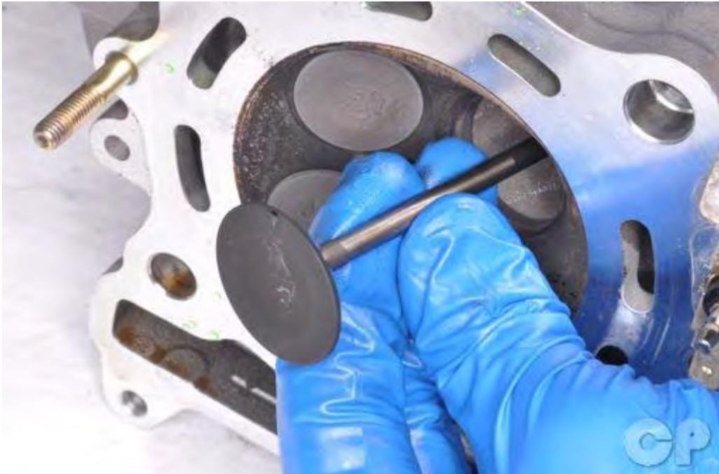
Coat the valve stem in fresh engine oil and insert the valve into the valve guide and through the seal. Turn the valve slowly as it is inserted. If you are installing a new valve you must ream the valve guide first. Make sure the valve will move smoothly in the valve guide without wobble.
