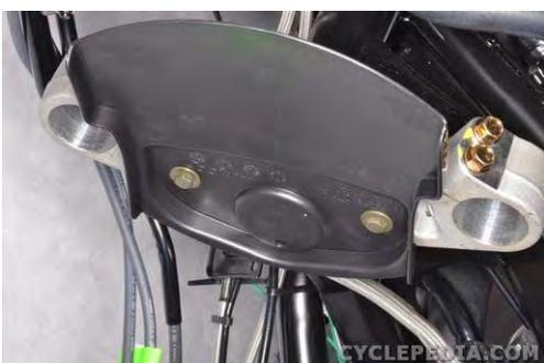
Install the inner fender and tighten the two bolts securely with an 8 mm socket.
