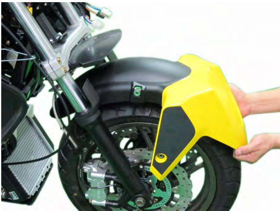
Remove the front fender from the forks.
