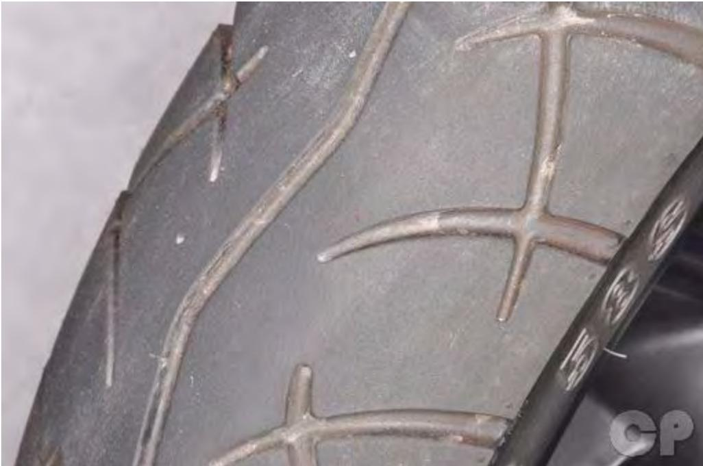
Replace tires if the tread depth reaches the wear mark or fails to meet the minimum tread depth.
