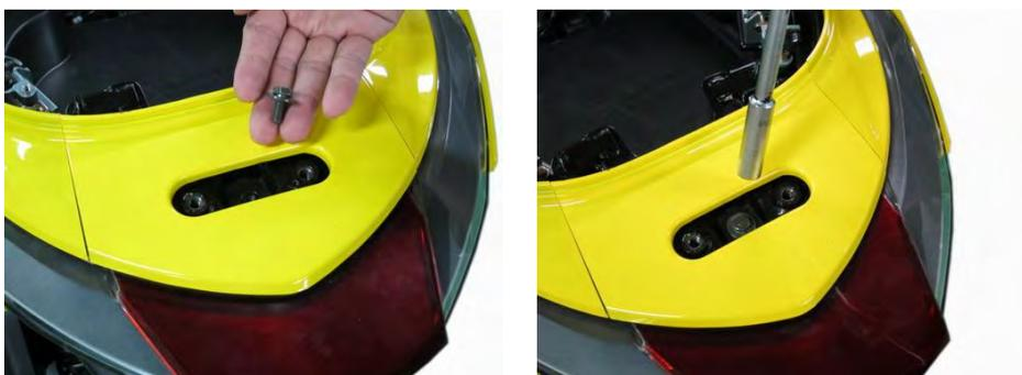
Install the upper body cover bolts and tighten securely with a 10 mm socket.
