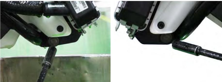
Remove the two radiator bottom mounting bolts with a 10 mm socket.
