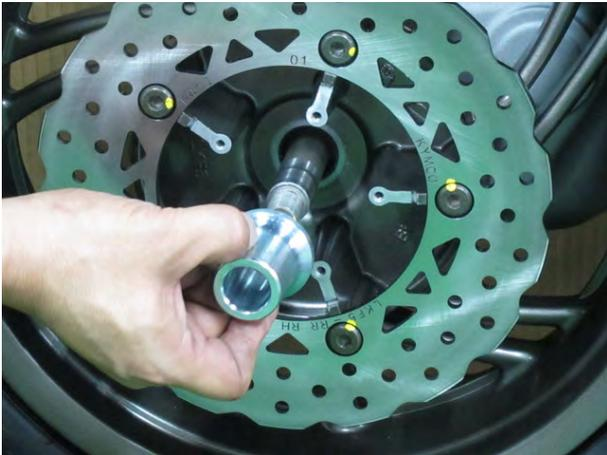
Install the rear axle collar as shown.
