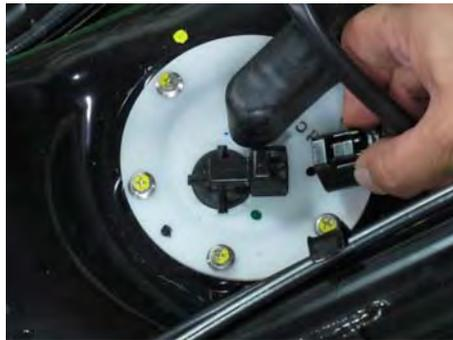
In order to drain the fuel from the fuel pipe and release the fuel pressure unplug the fuel pump connector. Start the engine and let it run until it dies of fuel starvation. Turn the ignition switch off.
