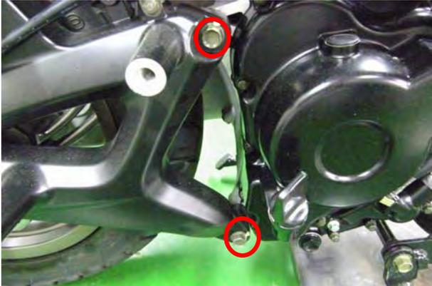
Install the two rear fork bolts and tighten them to specification with a 12 mm socket.
