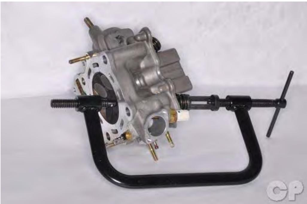
Push down the valve springs with a valve spring compressor to allow enough room to install the split keepers. The valve cotter installer tool can also be used to install the split keepers.
