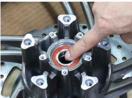
Inspect the wheel bearings by turning them in the hub. If the bearings have excessive play in them or are rough replace all the bearings for that wheel.
