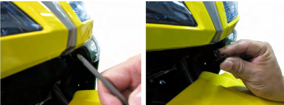
Remove the push pin. Depress the head of the fastener center piece.
