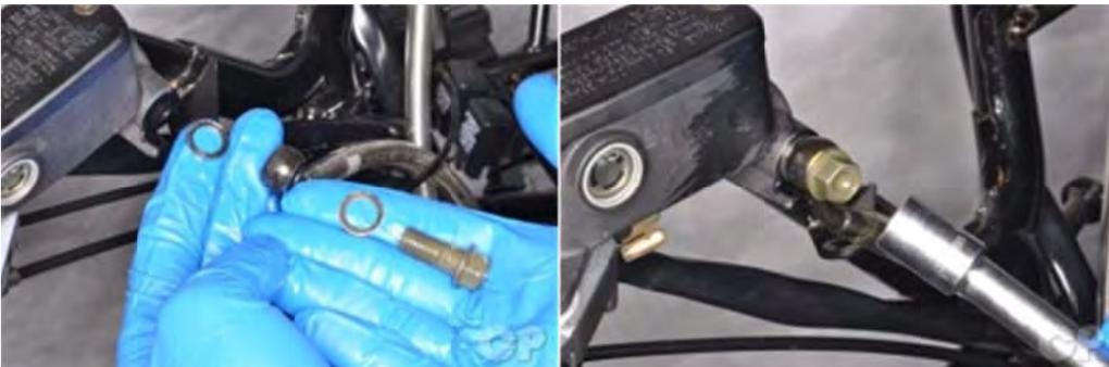
Install the brake hose to the master cylinder with the banjo bolt. Use new sealing washers. Tighten the banjo bolt to specification with a 12 mm socket.
