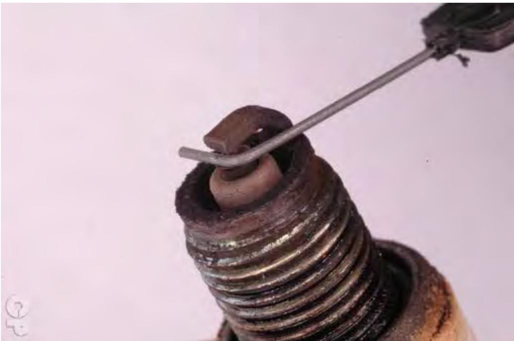
Always check the gap of the spark plug before installation. If the gap needs to be adjusted bend the ground electrode carefully. Inspect the color of the porcelain nose of the spark plug. The color of the spark plug can indicate how the mixture is burning. A white colored plug shows a lean mixture, where a dark plug shows a rich mixture. Do not hesitate to replace a spark plug. Always replace a spark plug if any part of it is damaged.
