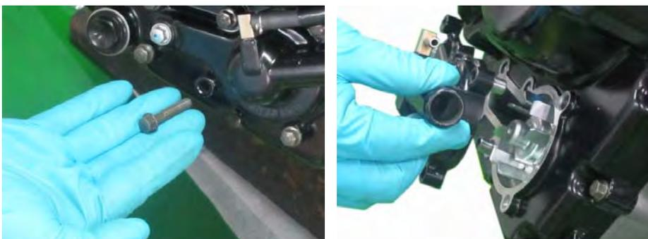
Remove the bolts and the water pump cover.
