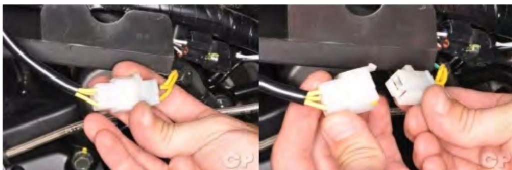
Disconnect the generator 3-pin connector.
