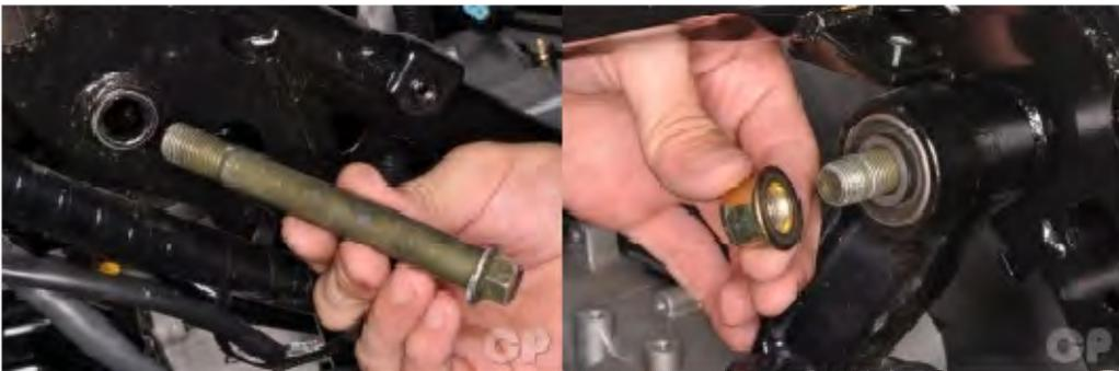
Install the two engine mounting bracket to frame mounting bolts and nuts. Insert the bolts from the outside of the frame.
