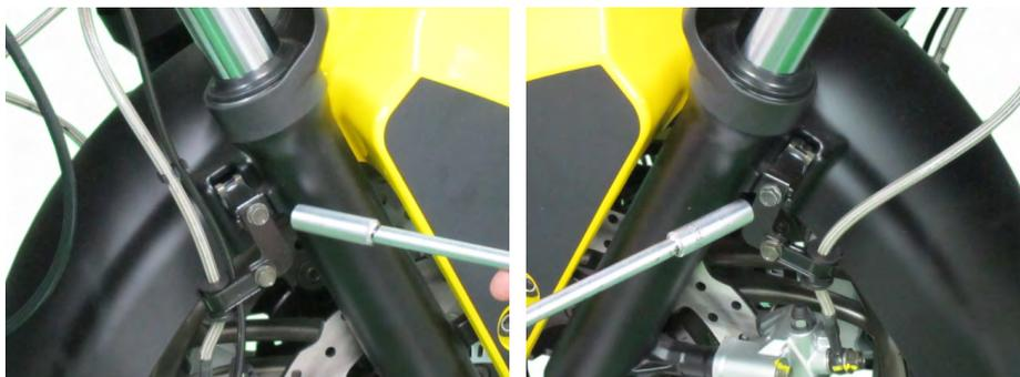
Install the forward front fender bolts with a 10 mm socket on both side.
