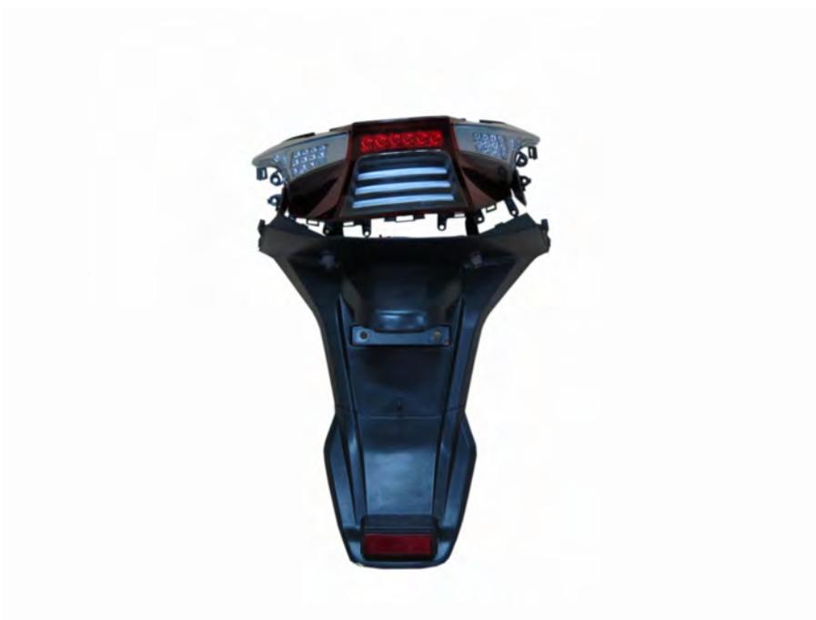
Separate the mud flap from the taillight assembly.
