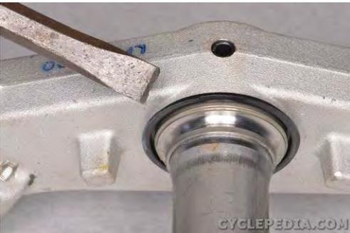
Use a chisel to remove the bottom bearing inner race and dust seal. Do not damage the steering stem.
