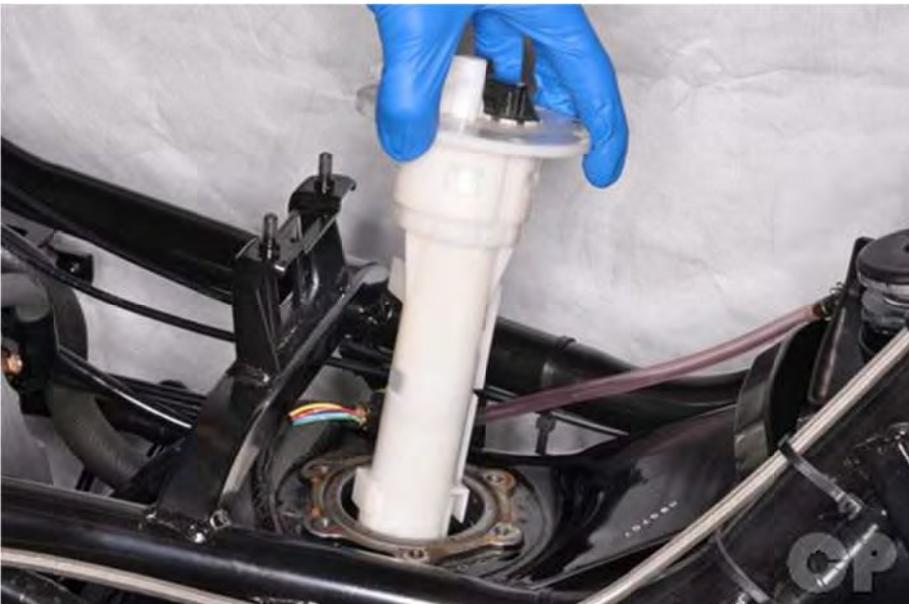
Carefully insert the fuel pump into the tank. Avoid damaging the fuel pump wire. The fuel delivery pipe should face to the rear.
