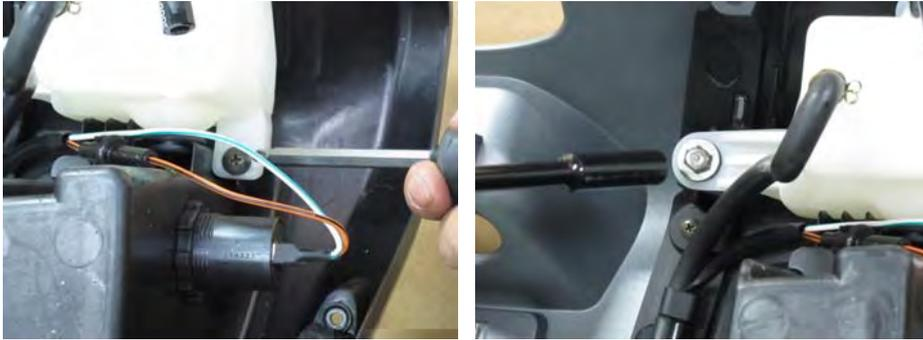
Install the left reserve tank mounting bolt with a 10 mm socket and bottom screw with a #2 Phillips screwdriver.
