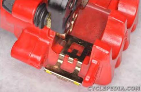
Remove the brake pad spring.
