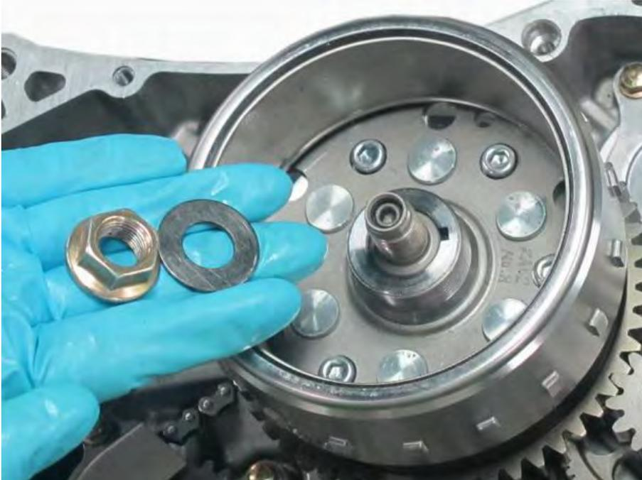
Remove the flywheel nut and washer.
