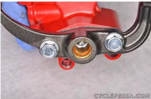
Install the two parking brake bracket bolts and tighten them to specification with a 12 mm socket.
