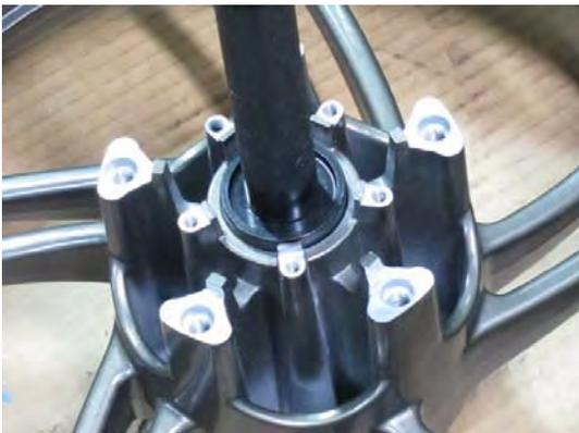
Drive in the other bearing. The bearing should fit against the distance collar. Do not continue to force the bearing in or the distance collar will begin to push the right bearing back out.
