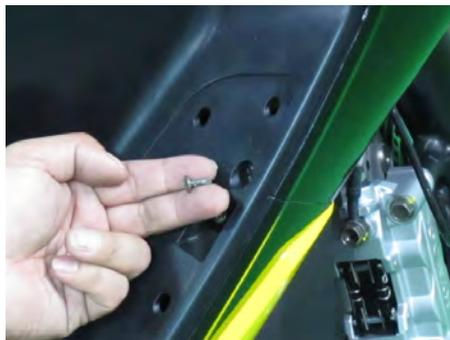
Remove the right leg shield mounting screws with a #2 Phillips.
