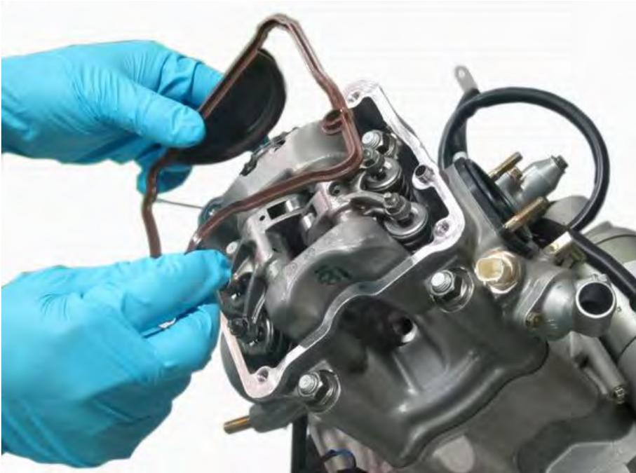
Fit the cylinder head cover gasket onto the cylinder head. Make sure the projection fits into the groove in front of the camshaft sprocket correctly.
