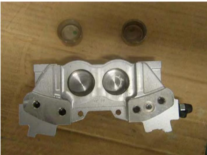
Lubricate the caliper pistons, the caliper piston bores with DOT 4 brake fluid from a tightly sealed container.
