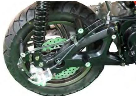
Remove the rear shock mounting bolts with a 14 mm socket.
