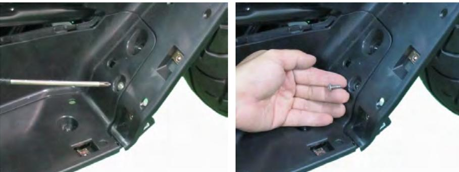
Remove the mounting screw with a #2 Phillips on right side.
