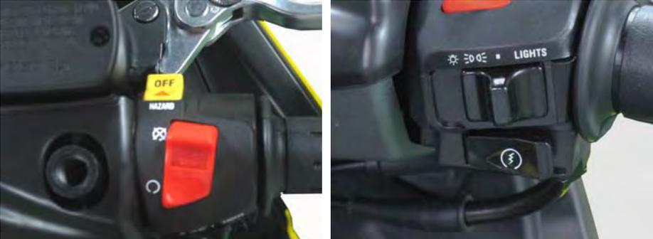
Use a digital multimeter to check for continuity to inspect the handlebar switches. Continuity should exist between the wires as indicated.
