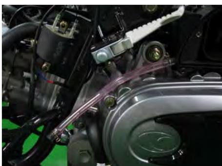
Fit the drain hose to the plastic belt case cover as shown.
