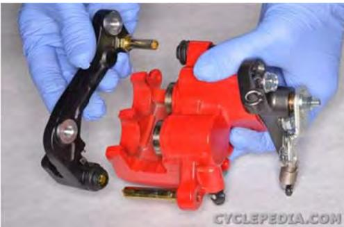
Slide the brake caliper bracket out of the caliper.
