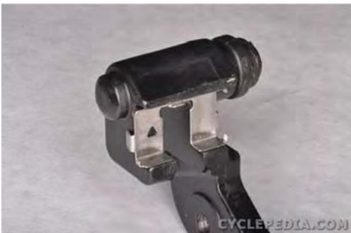
Install the pad retainer onto the caliper bracket.
