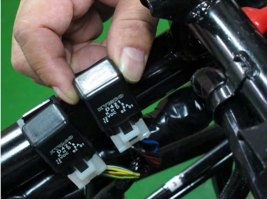
The fuel pump relay is located in front of battery. Remove and disconnect the fuel pump relay.
