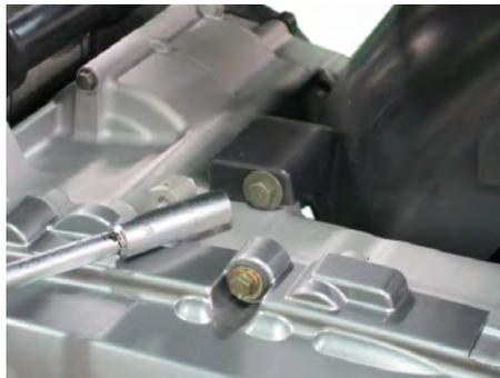
Install the left fender mounting bolts with a 10 mm socket on the front side.
