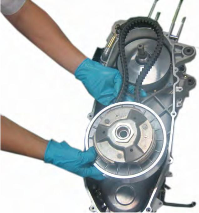
Slide the driven pulley off of the shaft.
