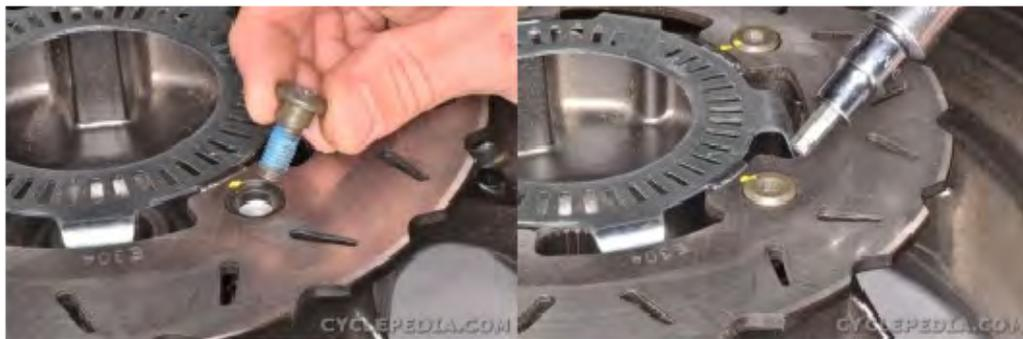
Apply a non-permanent thread locking agent to the threads of the rear disc bolts. Insert the bolts and tighten them to specification with a 6 mm Allen.
