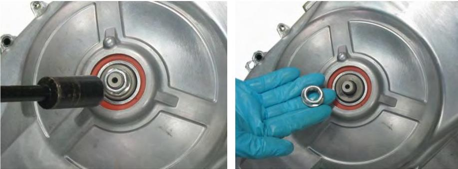
Remove the #M14 nut mounting the clutch outer.
