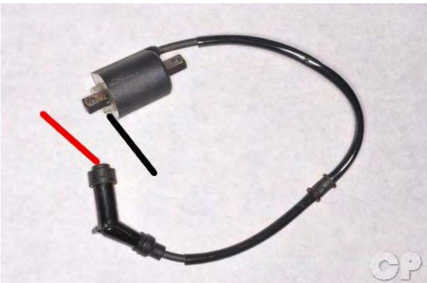
Check the secondary resistance between the ignition coil terminal and the spark plug cap. Touch the negative meter lead to the terminal and the positive meter lead to the spark plug cap as shown.
