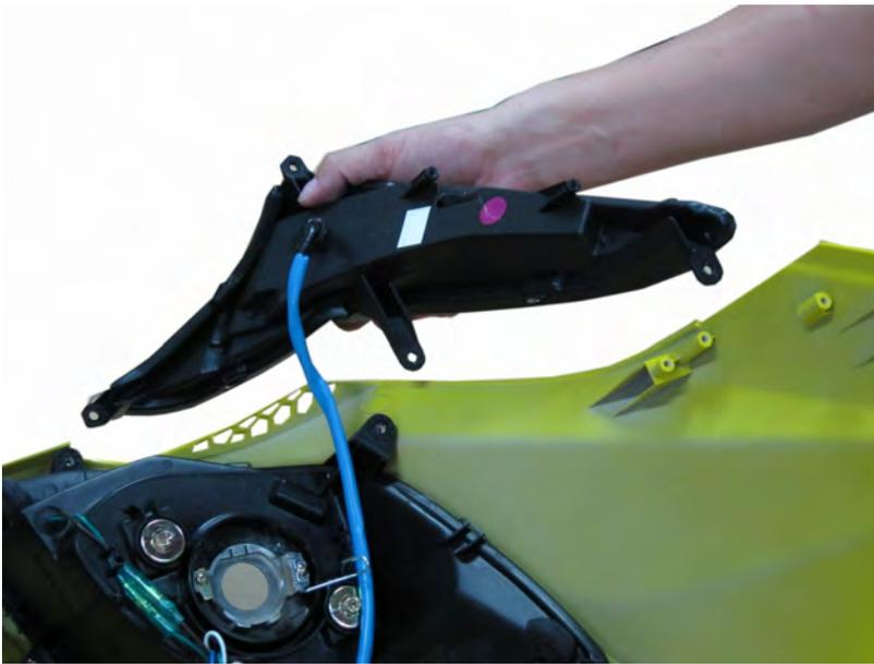
Remove the turn signal light assembly.
