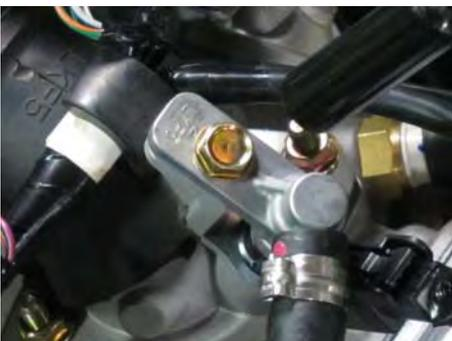
Tighten the fuel injector bolt securely with a 10 mm socket.
