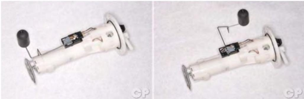
Using a digital multi meter set to ohms of resistance ( $\Omega$ ), measure the resistance between the fuel pump/level gauge connector terminals (green and yellow/white) with the float raised to the positions indicated below.
