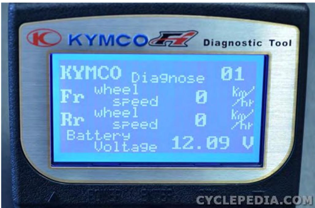
When using the DATA Analyze feature of the diagnostic tool with the ABS system the front and rear wheel speed sensors should show speed when the wheels are rotated.
