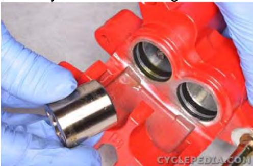
Install the parking brake piston into the caliper.
