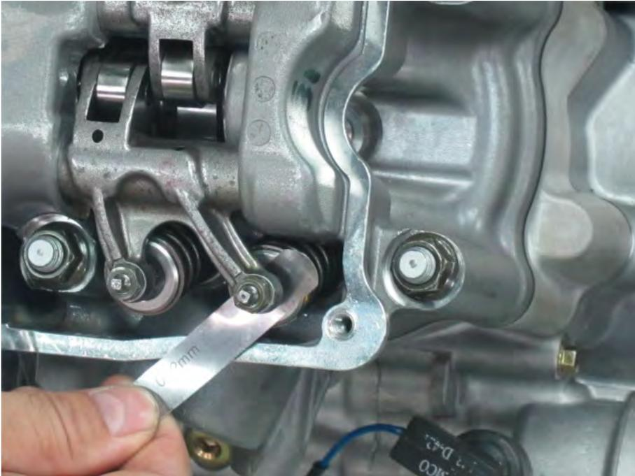
Measure the valve clearance with a thickness feeler gauge. Insert the feeler gauge between the tappet adjusting screw and the valve stem. The clearance is correct when there is a light drag on the feeler gauge. The clearance is the same for the exhaust and intake valves. If the clearance is out of spec, move on to the adjustment section.
