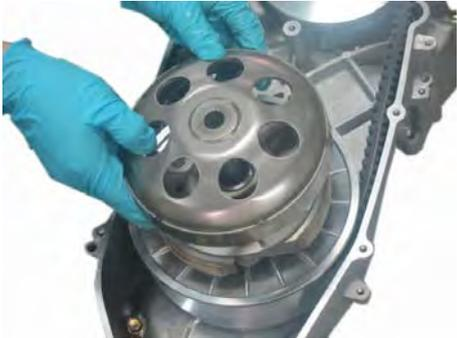
Remove the outer clutch.
