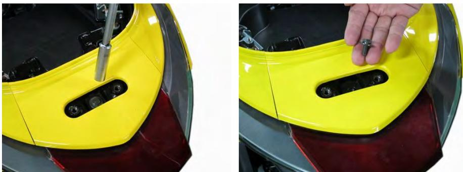
Remove the upper body cover bolt with a 10 mm socket.
