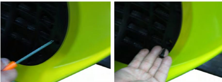
Remove the six lower fairing push pins.
