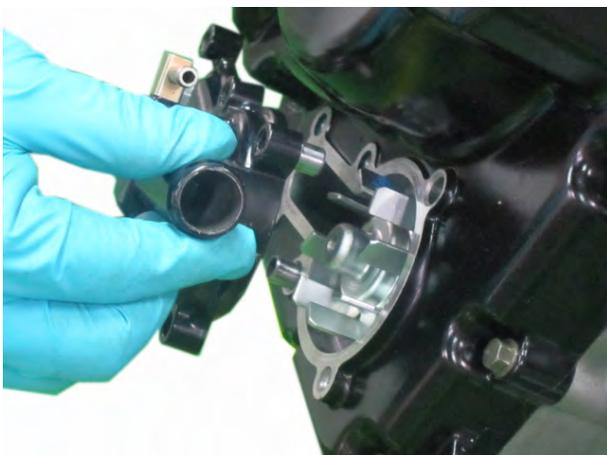
Install the two dowel pins into the generator cover and set a new water pump cover gasket in place.
