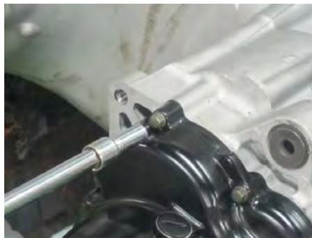
Insert the 12 generator cover bolts. Note the upper bolt holds a wire stay. Tighten the bolts securely in a with an 8 mm socket.
