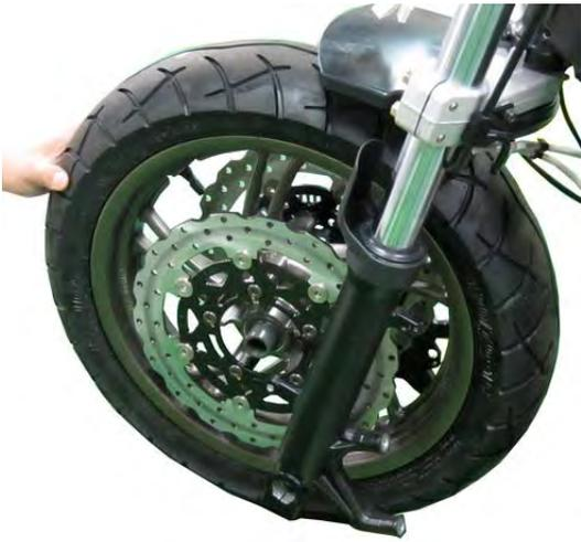
Make sure the tire direction of rotation marker is correct.
