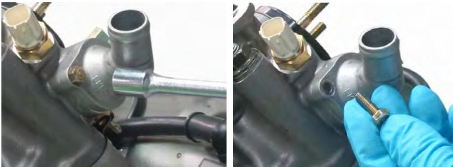
Remove the two thermostat mounting bolts with an 8mm socket.
