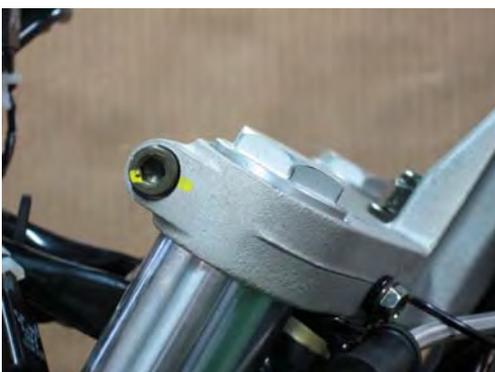
Fit the fork into place so that the mark on the top of the fork tube lines up with the upper fork clamp as shown.
