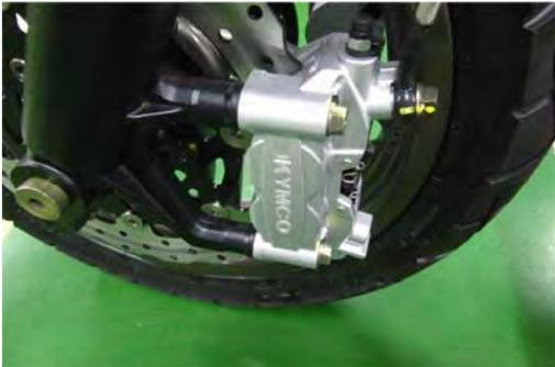
Push the caliper body inward to push in the pistons.
