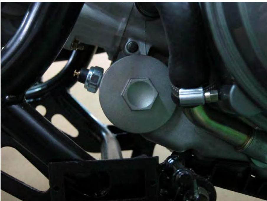
The oil filter compartment is located on the bottom of the engine below the oil filler cap/dipstick. Ready an oil drain pan to catch any remaining engine oil.
