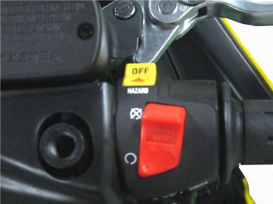
Set the engine stop switch to the “RUN” position.
