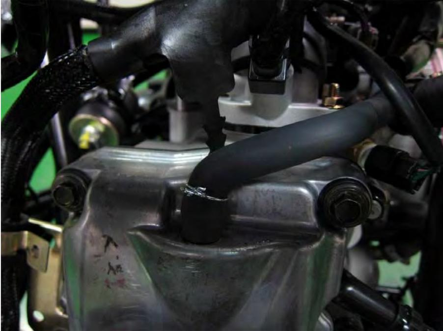
Inspect the breather hose for damage and deterioration.
