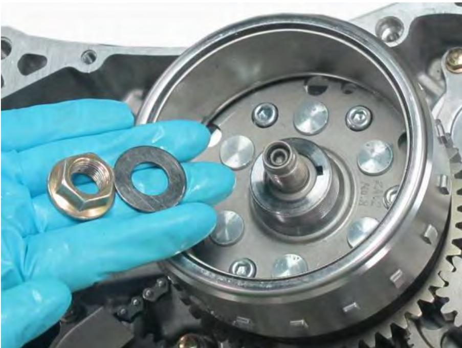
Install the washer and flywheel nut.
