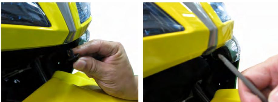
Align the two posts with the grommets. Carefully push on the small black cover.
