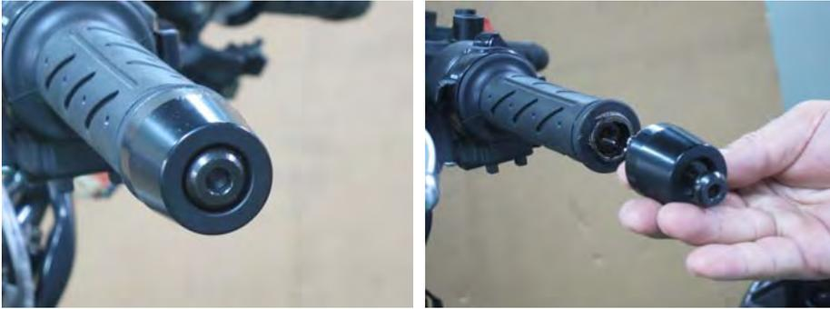
Remove the bar ends with a 6 mm Allen.
