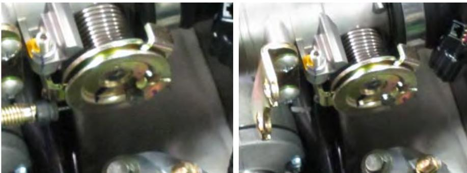
Connect the throttle cables to the throttle drum.
