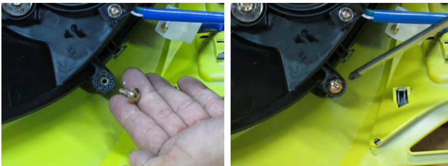
Install the headlight assembly mounting screws and tighten securely with a #2 Phillips.
