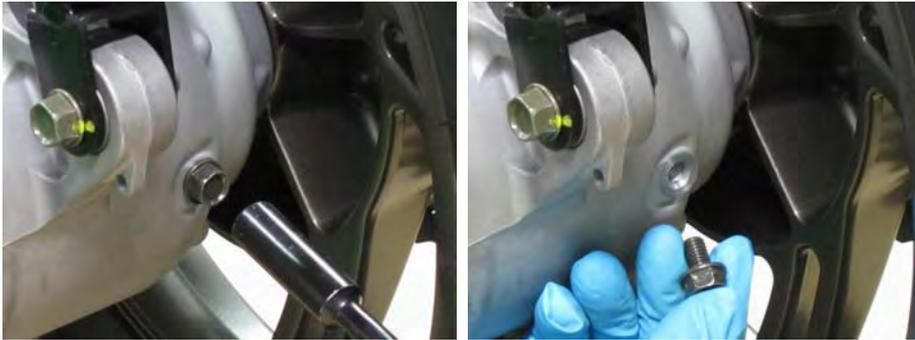
Remove the transmission oil level check bolt with a 12 mm socket. The oil level is correct when oil flows from the bolt hole. Install the oil level check bolt and tighten it to specification with a 12 mm socket.
