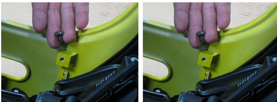
Remove the two rear center cover screws.
