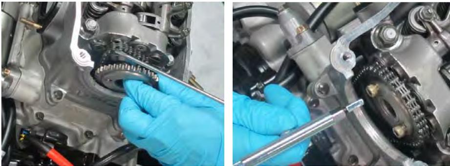
Install the camshaft sprocket onto the camshaft so the camshaft sprocket boss fits into the appropriate hole on the camshaft sprocket.
