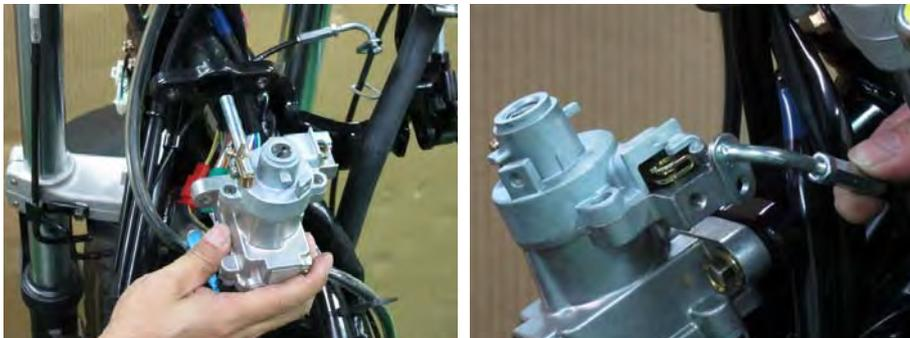
Fit the end of the seat latch cable into the ignition switch.
