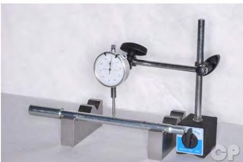
Check the front axle runout. The axle runout specification is half of the total indicator reading. Replace the axle if the measurement exceeds 0.2 mm or 0.008 in.
