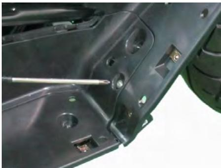
Install the mounting screw with a #2 Phillips on right side.
