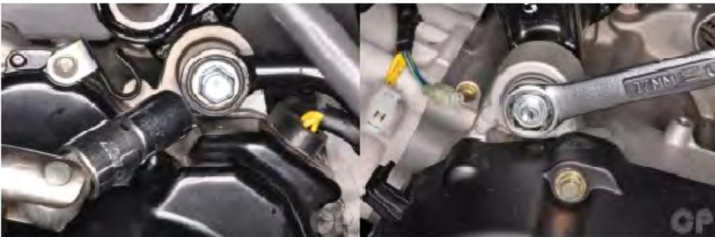
Loosen the engine mounting bracket damper bolt and nut with a 17 mm wrench for the nut and a 14 mm socket for the bolt.
