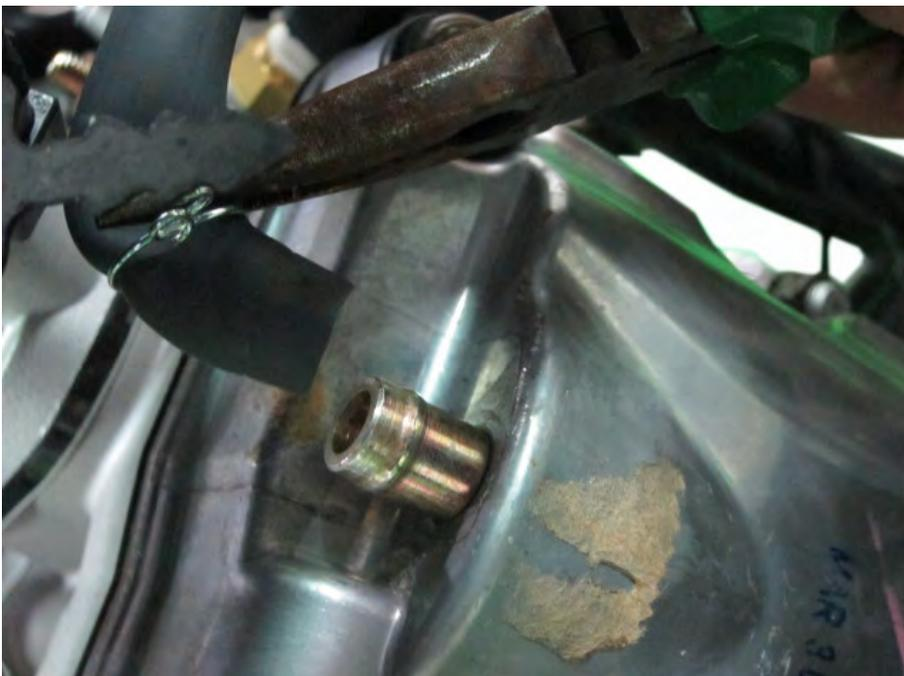
Disconnect the blow-by tube mounting the cylinder head with a splicer.
