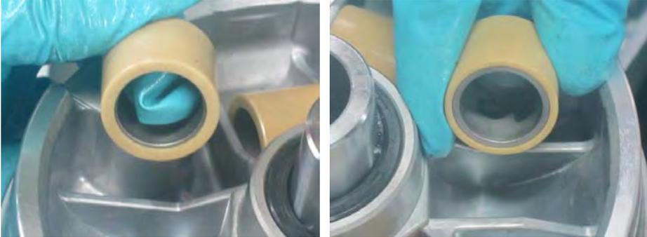
Remove the rollers and check them for excessive or uneven wear.
