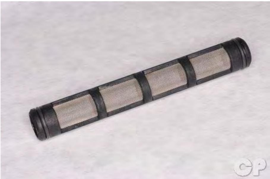
Remove the O-rings from the oil strainer screen and inspect them. Replace the O-rings if they are in poor condition. Inspect the oil strainer screen for debris and damage. Clean it with a high flash point solvent and compressed air. Metal debris in the strainer screen can be an indicator of engine wear or damage.
