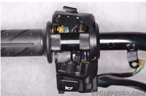
Align the left switch housing and install it onto the handlebar. The post in the switch housing must fit into the corresponding hole in the handlebar. Fit the left side of the switch housing into the plastic ring as shown.
