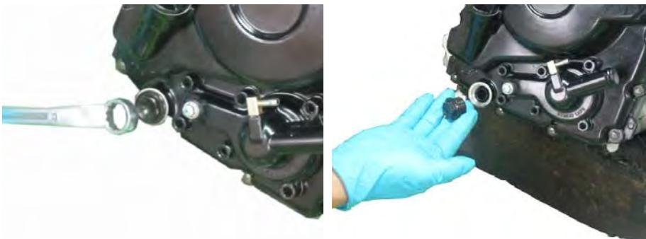
Remove the oil strainer screen bolt with a 17 mm socket. Inspect the strainer screen bolt O-ring and replace it as needed.
