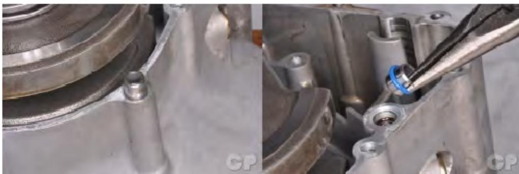
Remove the two dowel pins from the crankcase. Inspect the O-ring and replace it as needed.
