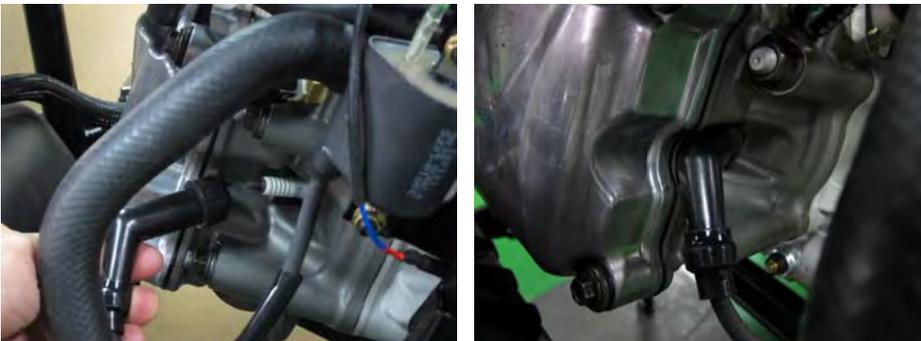
Install the spark plug wire over the plug.
