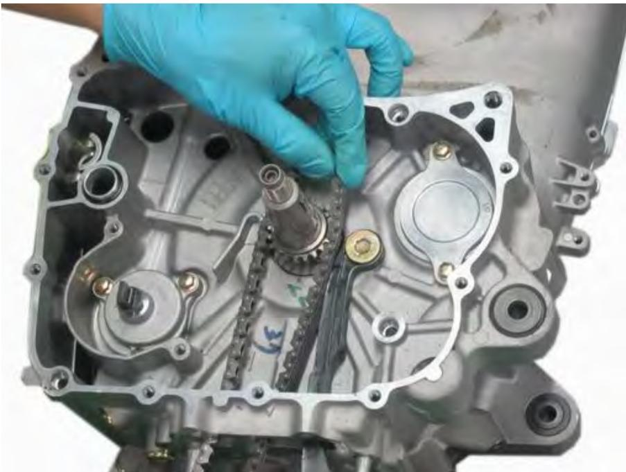
Remove the cam chain from the crankshaft and crankcase. Inspect the cam chain for wear and damage. Replace the cam chain as needed.
