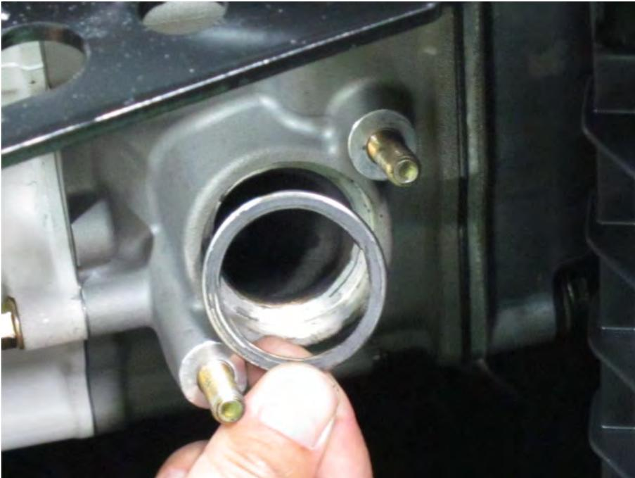
Insert a new exhaust pipe gasket into the exhaust port.
