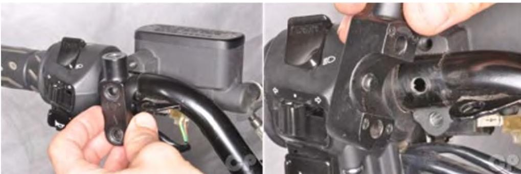
Remove the master cylinder clamp.
