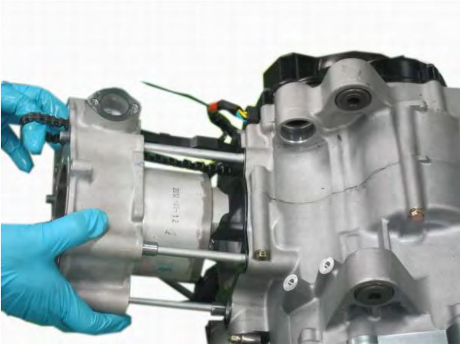
Slide the cylinder off of the studs and piston. Guide the cam chain through its opening and do not allow it to fall into the crankcase. Remove the cylinder.
