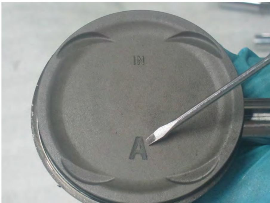
Clean the piston ring grooves and apply fresh engine oil to the piston rings. Spread the rings the minimum amount possible to install them. Do not try and force them on the piston.
