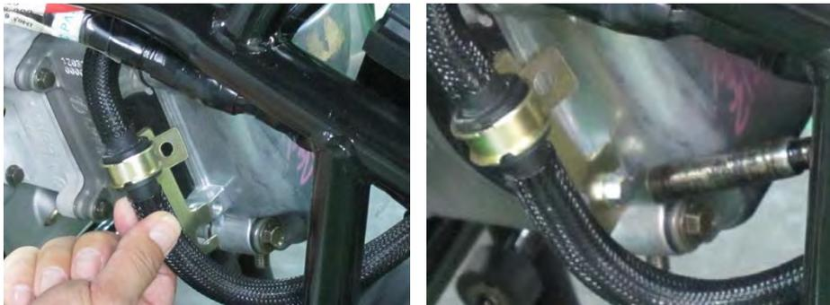
Fit the fuel stay into place. Tighten the stay bolt securely with an 8 mm socket.
