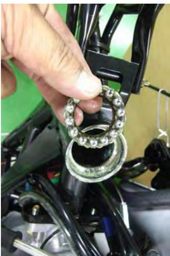
Lubricate the upper bearing with grease and set it into place.
