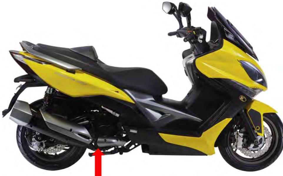
Inspect the telltale hole in the generator cover below the water pump for signs of coolant leaking. If there is coolant coming from this hole the mechanical seal is compromised and must be replaced.
