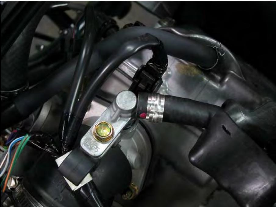
Inspect the fuel hose for signs of deterioration or damaged. Replace the fuel hose as needed.
