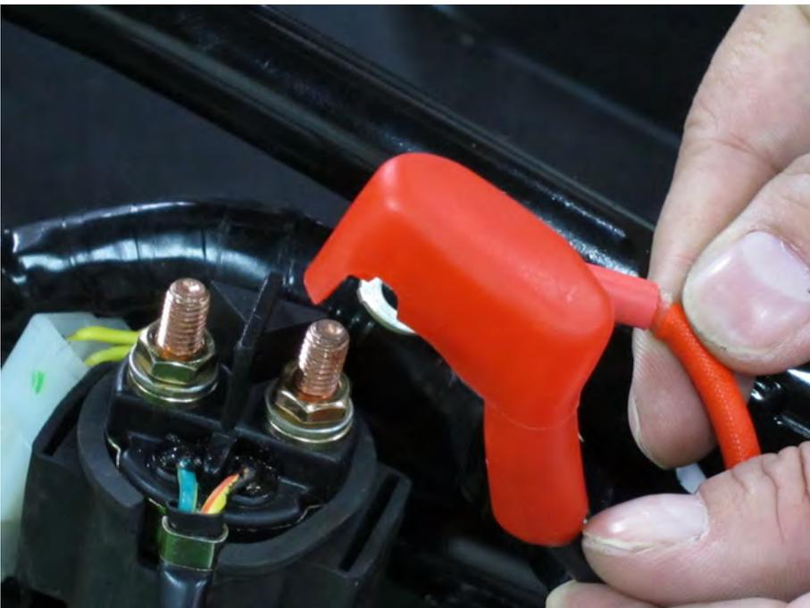
Remove the leads from the starter relay.
