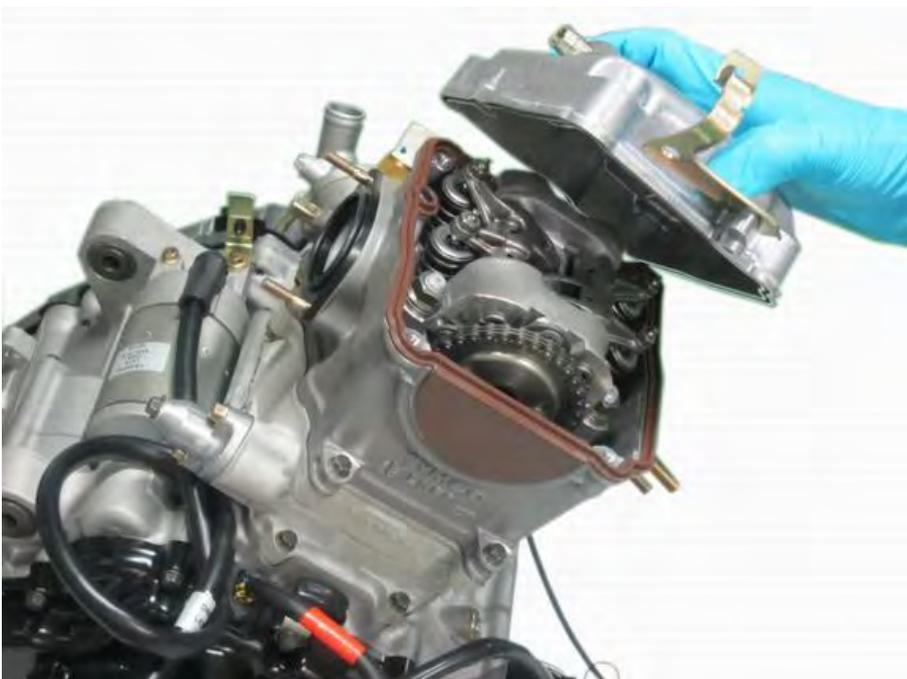
Install the cylinder head cover over the gasket. Make sure the ridge on the gasket fits into the groove on the cylinder head cover correctly. Align the bolt holes and dowel pin.
