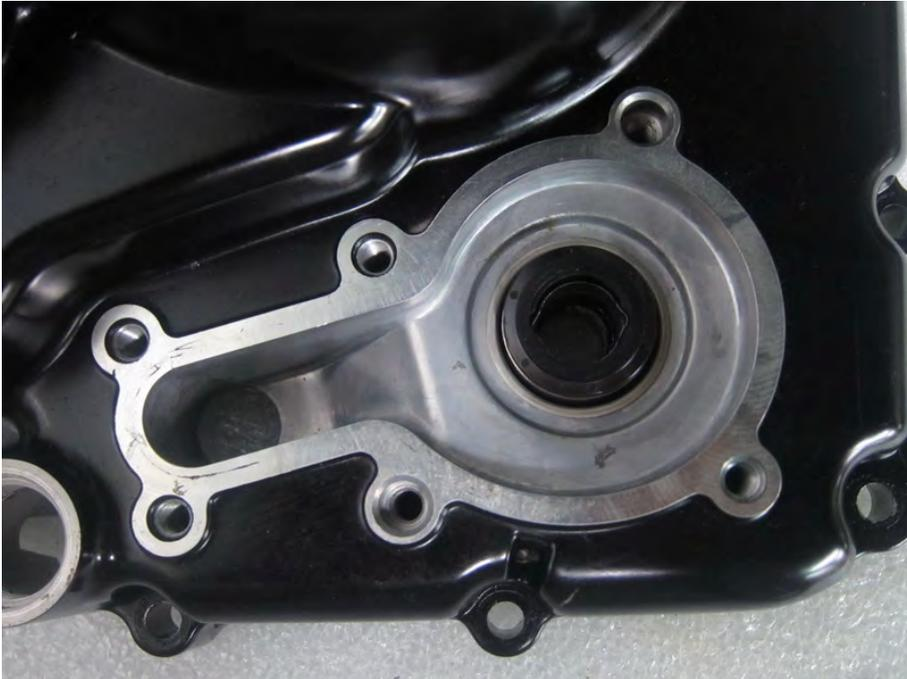
Apply silicone sealant to the outside of the mechanical seal. Press in the seal with a suitable drive that is the same outside diameter as the oil seal.
