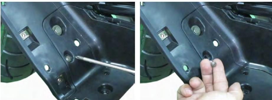
Remove the mounting screw with a #2 Phillips on left side.
