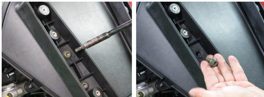
Remove the four cover windshield bolts with a 6mm Allen. There are two bolts on each side.
