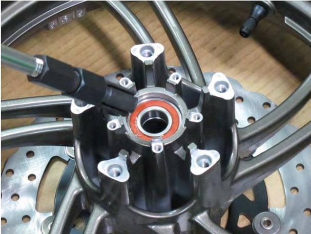
Remove one of the bearings with a bearing puller.
