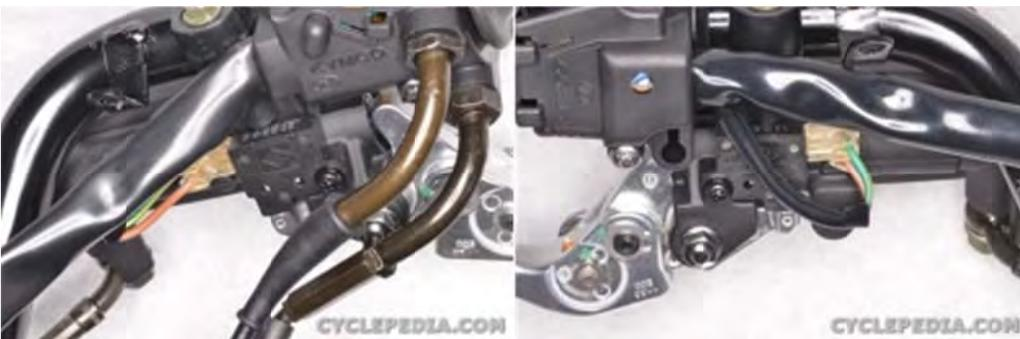
Plug in the brake light switch connectors.
