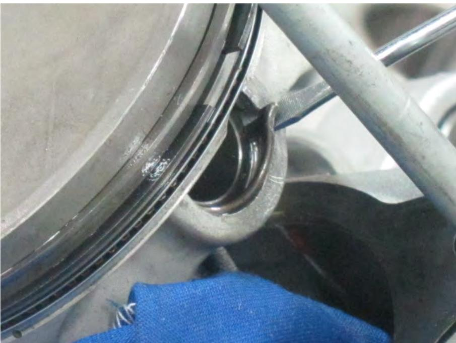
Remove the piston pin clips with a pick or needle nose pliers. Discard the piston pin clips.
