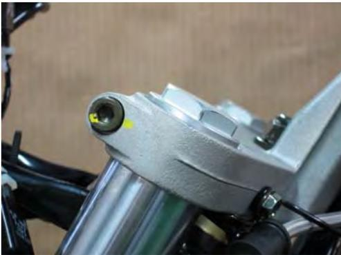
Tighten the fork caps securely with a 30 mm socket. Tighten the upper fork clamp bolts to specification with a 6 mm Allen socket.
