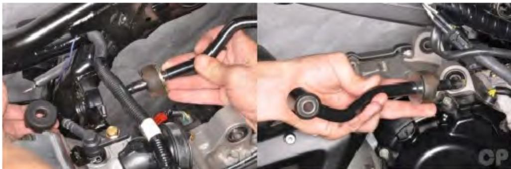
Remove the engine mounting bracket damper assembly.
