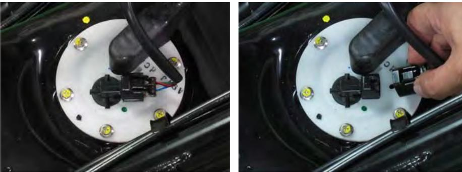
In order to release fuel pressure from the fuel pipe when removing the fuel injector, unplug the fuel pump connector. Start the engine and let it run until it dies of fuel starvation. Turn the ignition switch off.
