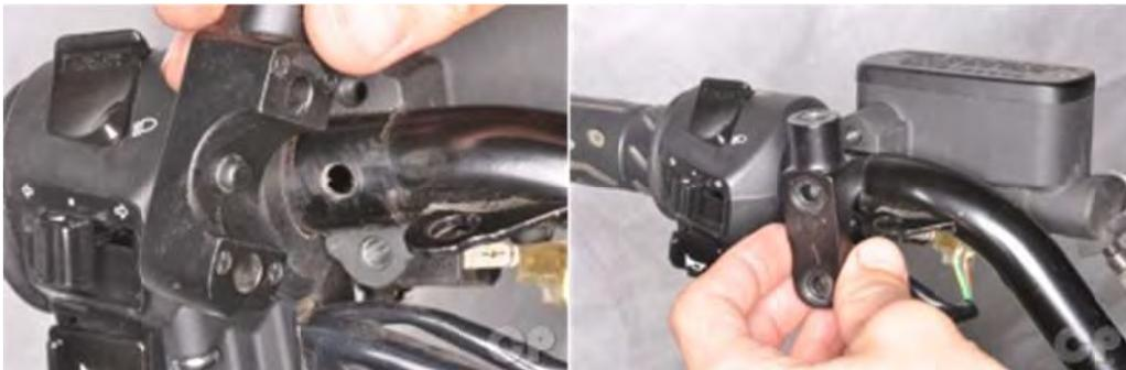
Install the master cylinder clamp. Be sure to insert the pin on the clamp into the hole on the handlebar.
