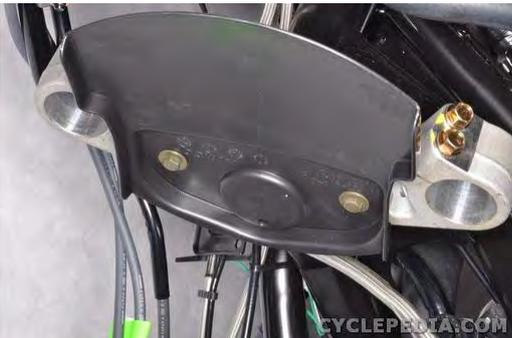
Remove the two inner front fender bolts with an 8 mm socket.
