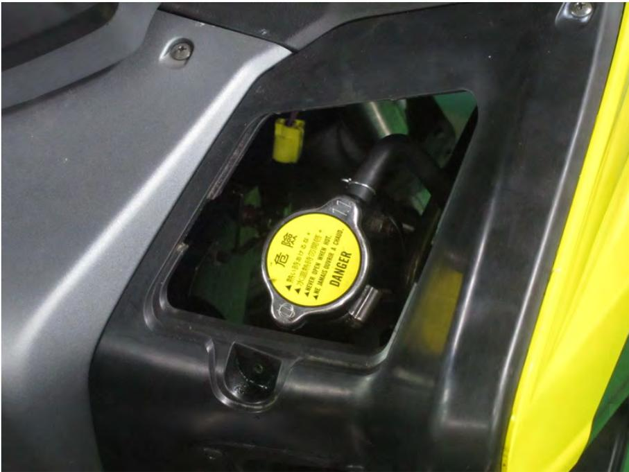
Fill the cooling system with a mix of distilled water and Coolant Concentrate. Continue filling until the coolant reaches the bottom of the filler neck as shown.
