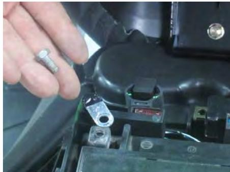
Remove the negative battery cable bolt with a 10 mm socket or #3 Phillips screwdriver.
