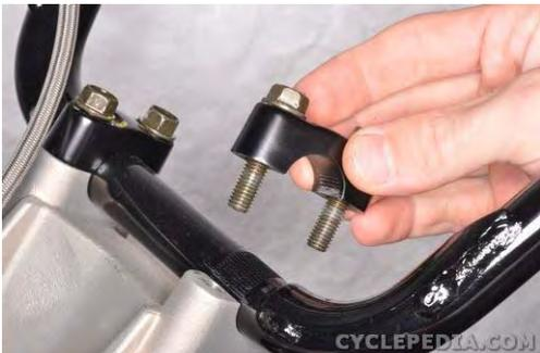
Remove the handlebar holders and bolts.
