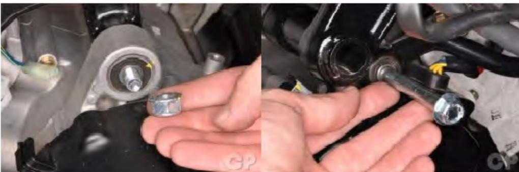
Remove the engine mounting bracket damper bolt and nut.
