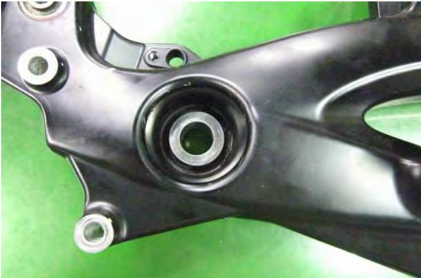
Remove the collar into the rear fork.
