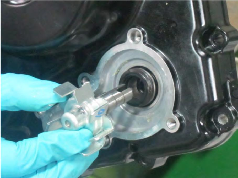
Remove the impeller.
