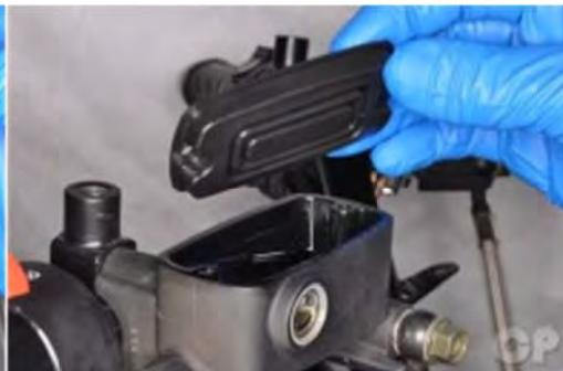
Remove the master cylinder cover, plastic piece and rubber accordion diaphragm. Pour out any remaining brake fluid.
