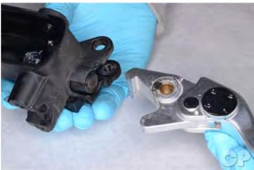
Remove the brake lever.
