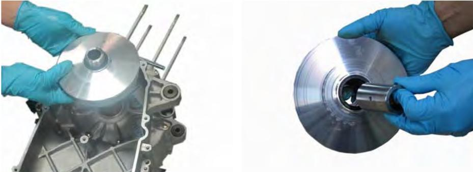
Remove the right (movable) face of the drive pulley from the crankshaft.
