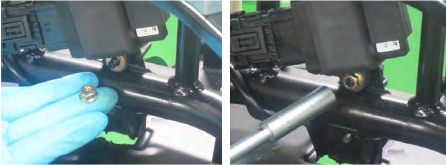
Install the two mounting nuts and tighten securely with a socket.
