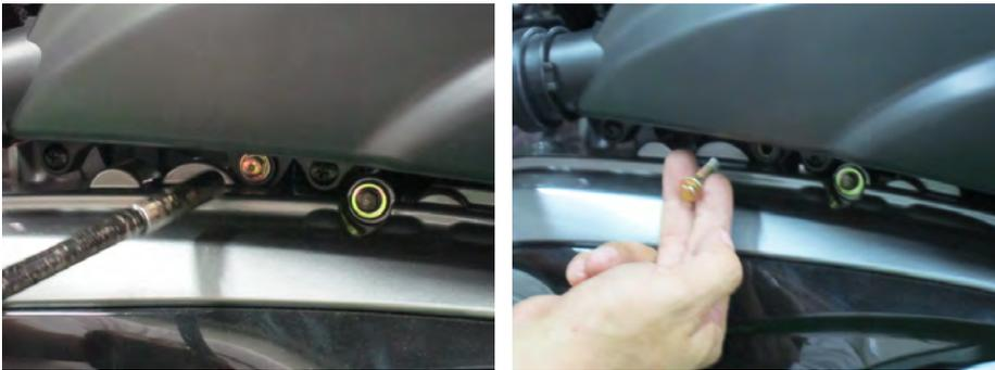
Remove the left fender mounting bolts with a 8 mm socket on the front side.
