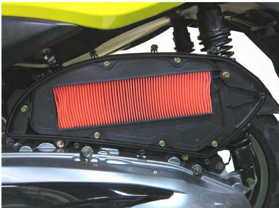
Insert the 7 air filter bolts. Tighten the air filter bolts securely with an 8 mm socket or a #2 Phillips screwdriver.
