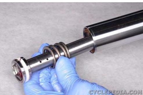
Remove the damper rod and rebound spring.
