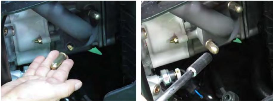
Install the two exhaust pipe joint nuts with a 12 mm deep well socket.
