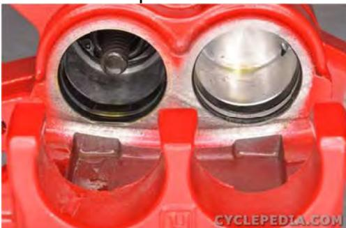
Install the new caliper piston fluid seal and dust seal, making sure they are fully seated in their grooves.
