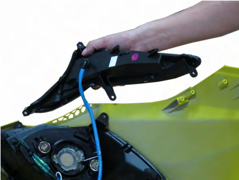
Install the turn signal light assembly.
