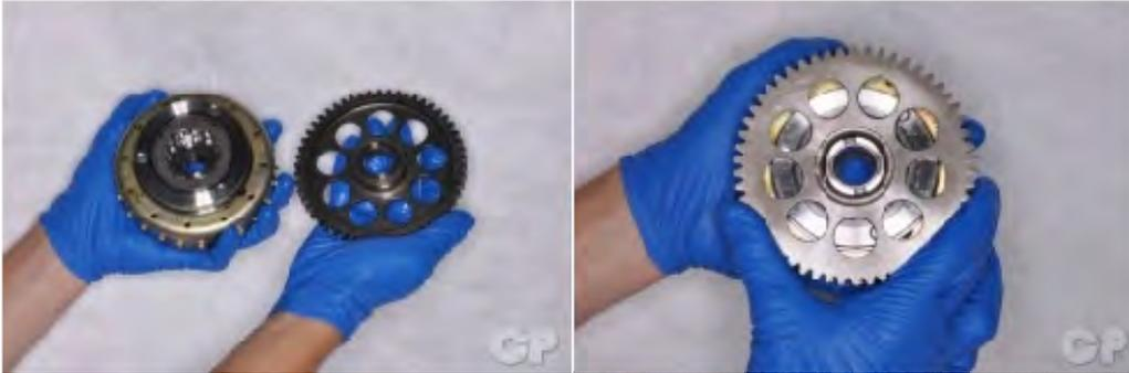
Fit the boss of the starter driven gear into the starter clutch. The starter clutch should only allow the driven gear to turn in one direction. If the starter clutch allows turning both ways or will not let the driven gear rotate smoothly in one direction the starter clutch must be replaced.
