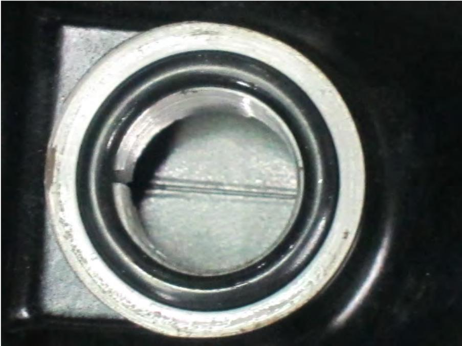
Position the piston at top dead center as above. The "T" mark should be aligned with the index notch in the timing inspection hole. Support the cam chain if the crank must be turned to position the piston correctly.
