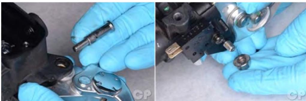
Apply a light coat of grease to brake lever pivot bolt. Insert the pivot bolt from above and thread on the nut.
