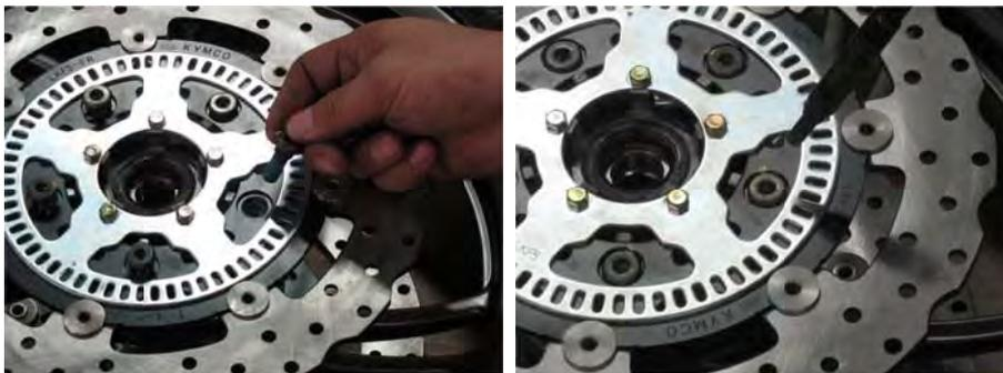
Coat the threads of the disc bolts in a non-permanent thread locking agent. Thread in the bolts and torque them to specification with an Allen socket.
