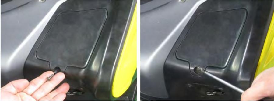
Install the radiator coolant panel screws and tighten securely with a #2 Phillips screwdriver.
