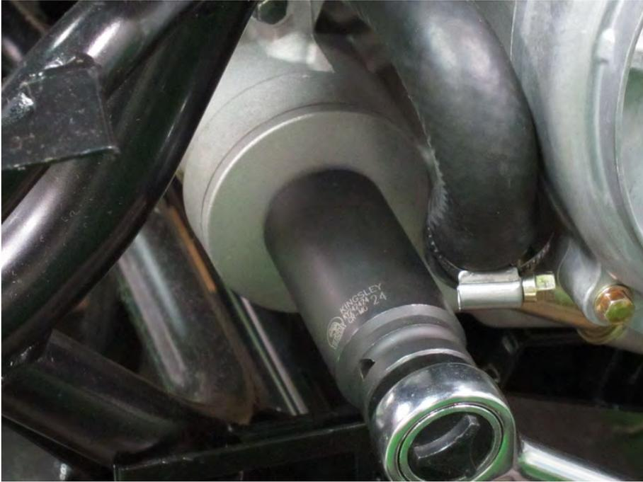
Loosen the oil filter cap with a 24 mm socket.
