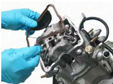
Remove the cylinder head cover and gasket.
