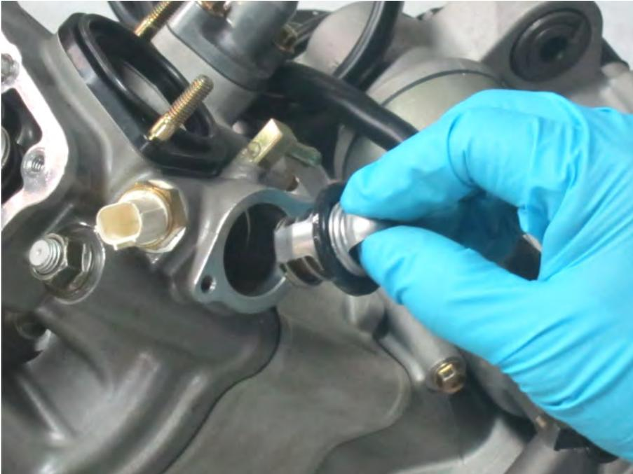
Lift out the thermostat. Remove the thermostat O-ring and discard it.
