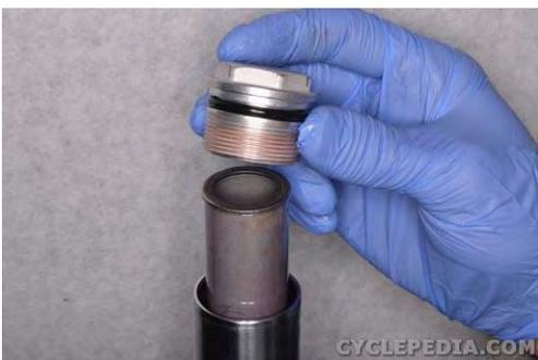
Remove the rubber fork cap with a 30 mm socket or wrench. Inspect the fork cap O-ring and replace it if needed.
