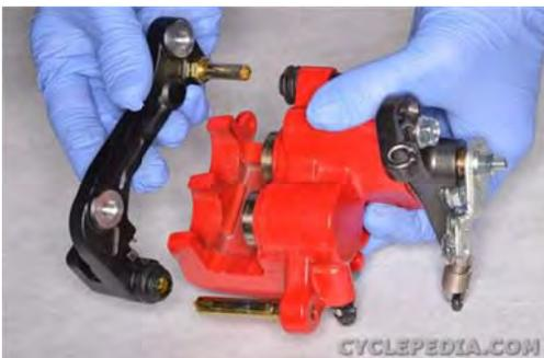
Apply a light coat of grease to the caliper bracket pins. Insert the caliper bracket pins into the boots.
