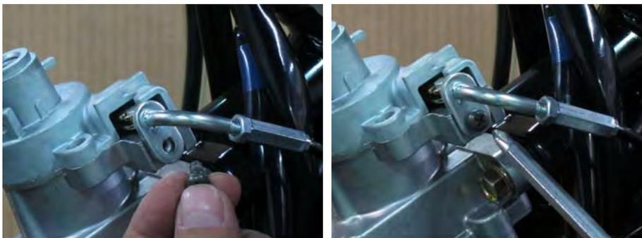
Install the seat latch cable screw and tighten it securely with a #2 Phillips screwdriver.
