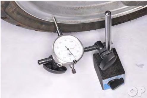
Place the wheel on a truing stand and use a dial indicator to check if the rim is out of true. The specifications for the front and rear wheels are the same. Check for lateral wobble. The service limit is 2.0 mm (0.08 in) or less.
