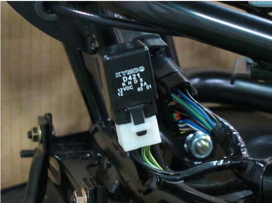
The ECU relay is located in the rear next to the ECU. Remove and disconnect the ECU relay.
