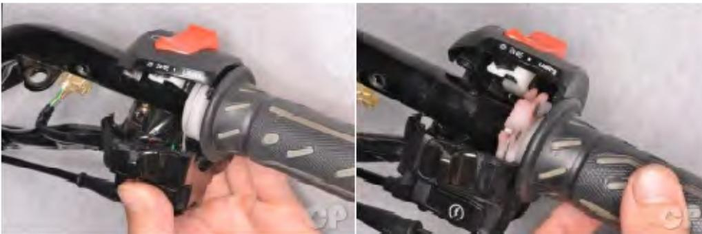
Separate the switch housing from the handlebar.
