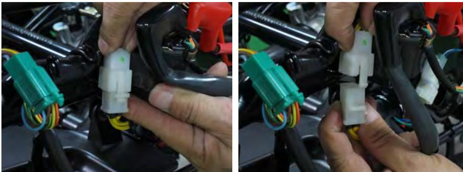
Disconnect the generator 3-pin connector.
