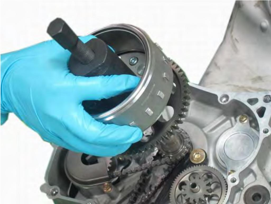
Remove the flywheel from the crankshaft.
