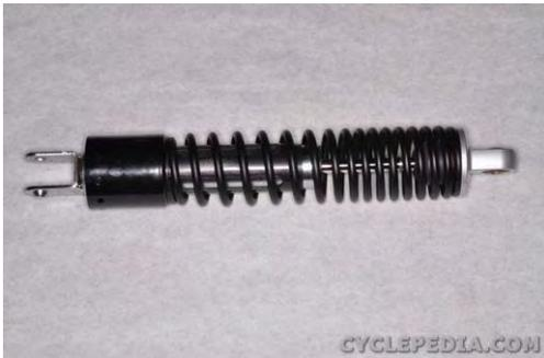
Check over the shock absorber for damage and oil leaks. Replace the shock absorber if needed. Do not attempt to disassemble the shock absorber.
