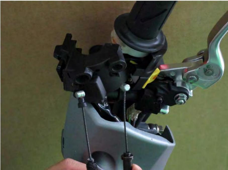
Route the throttle body end of the cables through the opening in the lower handlebar cover.
