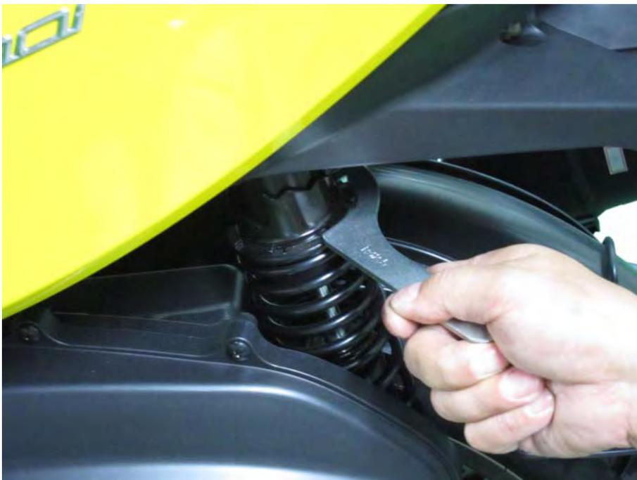
Use a pin spanner to adjust the rear shock spring preload. The shock absorbers are adjustable for pre-load. There are 5 settings. Position 1 is the softest and 5 is the stiffest.
