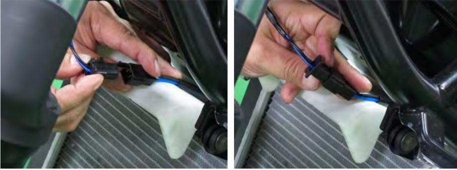
Plug in the cooling fan motor connector.
