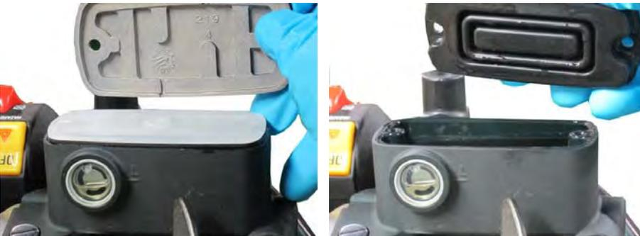
Remove the master cylinder cover, plastic piece and rubber diaphragm. Clean and inspect the rubber diaphragm for tears or other damage. Replace as necessary.
