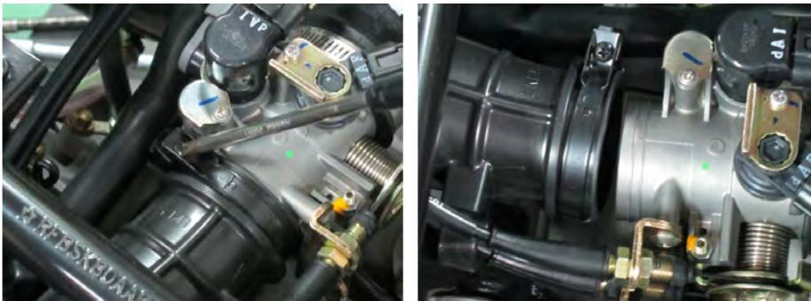
Remove the screw mounting the connecting tube airbox.
