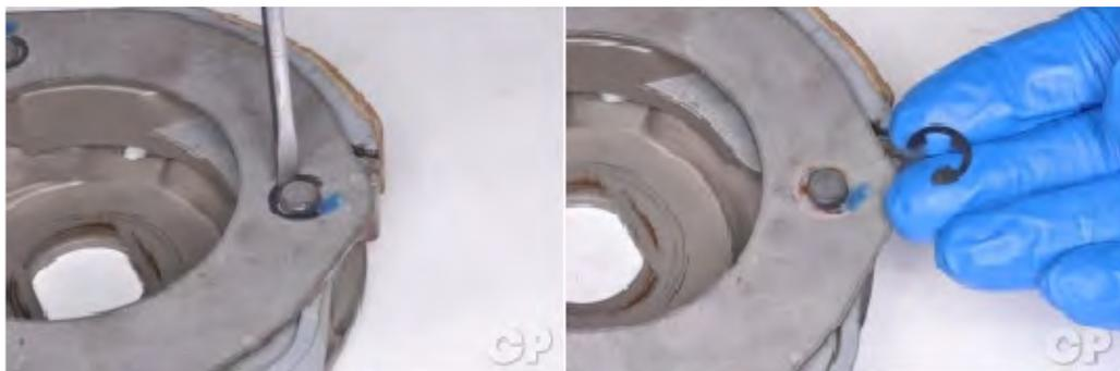
Remove the three circlips from the clutch pivot pins with a small flat blade screwdriver.
