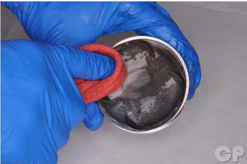
Clean the carbon build up off of the piston with a stiff bristled plastic brush or rag. Never use a wire brush to clean a piston.
