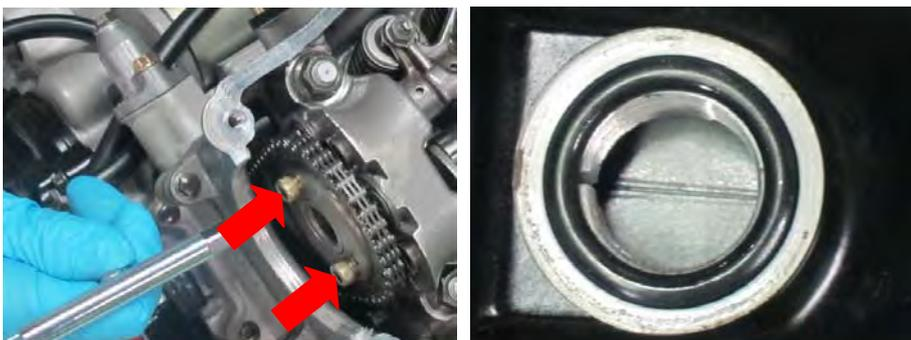
For correct engine timing the marks on the camshaft sprocket must be even with the cylinder head mating surface at the same time the "T" mark is lined up with the with the index notch in the timing inspection hole. The camshaft lobes should be facing down and their should be slack in the rocker arms.
