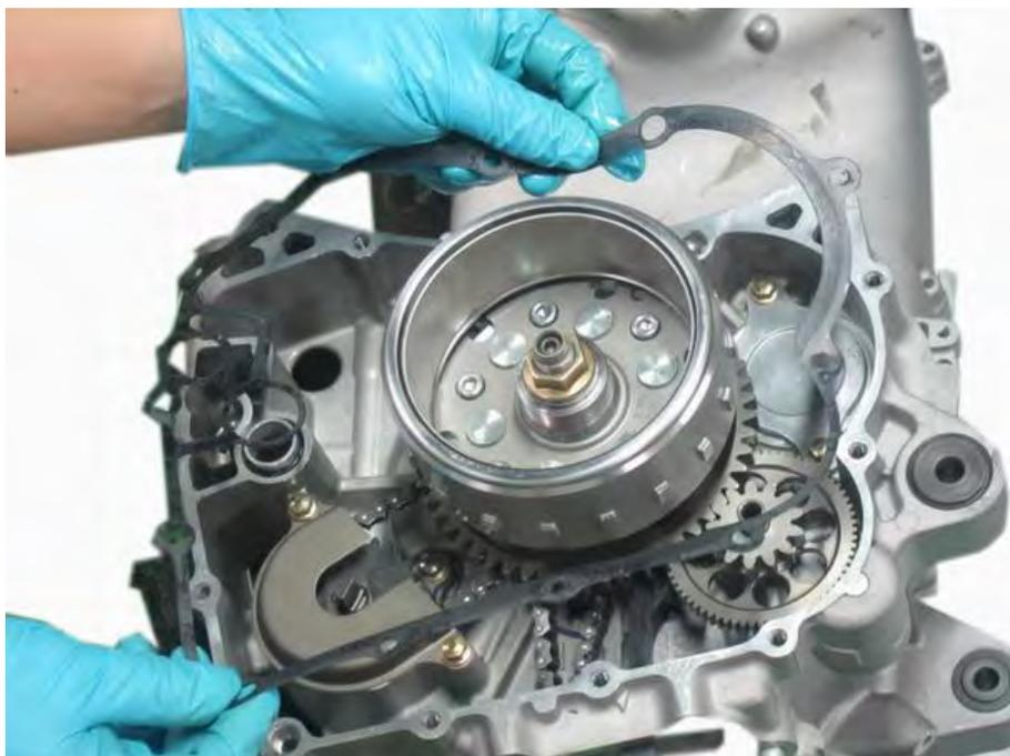
Remove the generator cover gasket.
