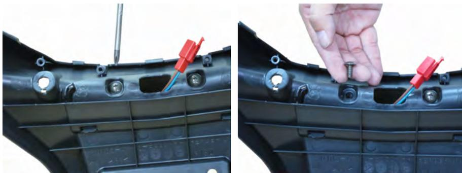
Remove the two license light cover screws with a screwdriver.
