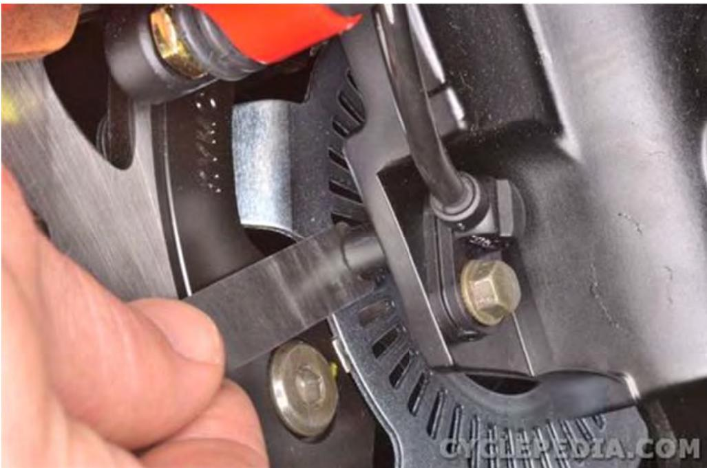
Check the speed sensor to rotor clearance with a feeler gauge and make sure that it is 0.3 - 1.2 mm (0.0012 - 0.048 in).
