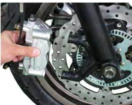
Remove the front brake caliper.
