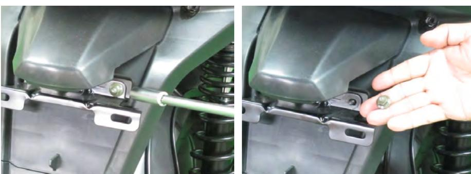
Remove the two license plate nuts with a 10 mm socket.
