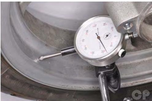
Check for radial hop. The service limit is 2.0 mm (0.08 in) or less.
