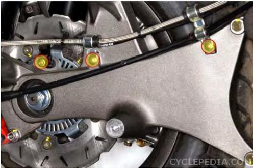
Install the rear wheel speed sensor and hose clamp bolts with an 8 mm socket.
