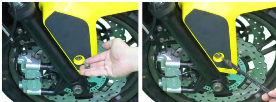
Install the forward front fender bolts with a 6 mm Allen on both side.
