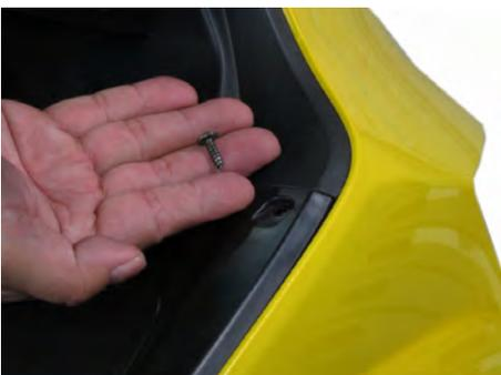
Remove the four front cover mounting screws with a #2 Phillips.
