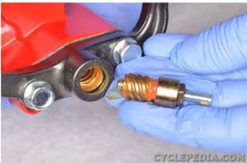
Lubricate the parking brake shaft with silicone grease. Insert the parking brake shaft and adjuster bolt into place.
