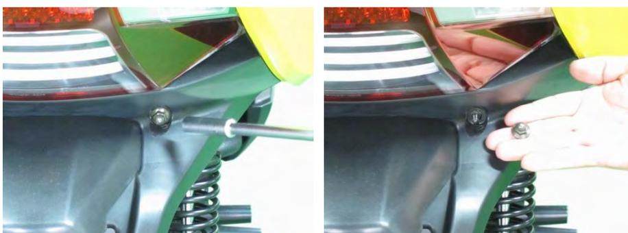
Remove the two lower body cover nuts with a 10 mm socket.
