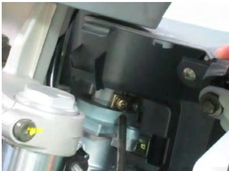
Install the bolt mounting the ignition switch and then collar ignition switch.
