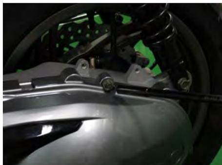
Insert the plastic cover bolts and tighten them securely with an 8 mm socket.
