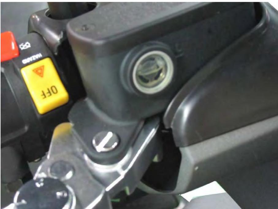
Turn the handlebars until the top of the master cylinder reservoir is level with the ground. Do this for both master cylinder reservoirs and check the level of brake fluid.
