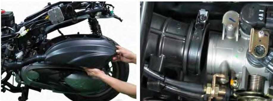
Fit the air box into the frame and guide the boot over the mouth of the throttle body.
