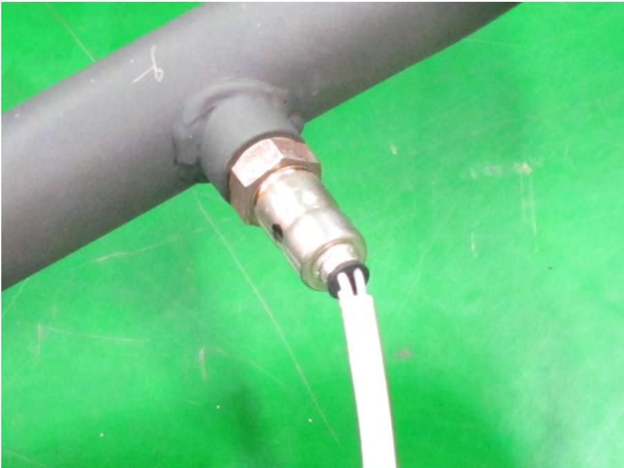
Remove the O<sub>2</sub> sensor with a 17 mm wrench.
