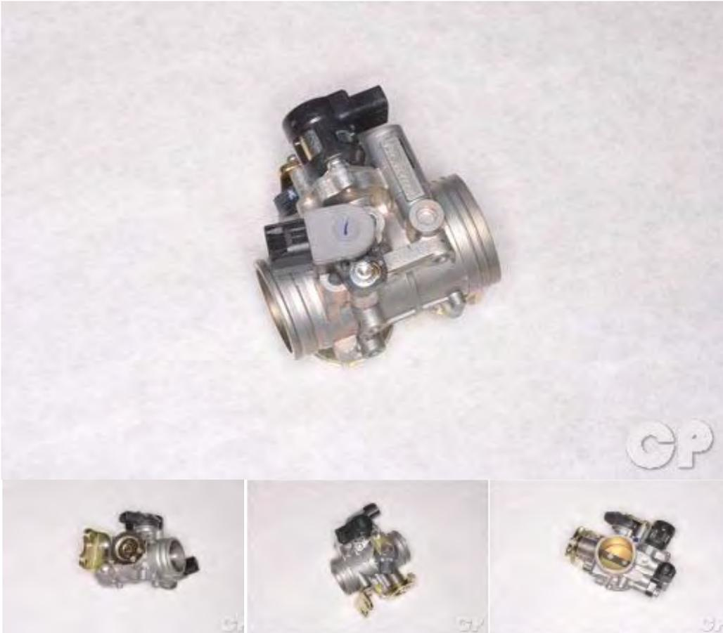
The throttle position sensor (TPS) and idle air bypass valve (ISC) have to be reset when the throttle body MAP, TPS, ISC or ECU have been reinstalled.
