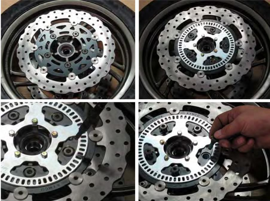
Remove the five mounting bolts with a 6 mm Allen.
