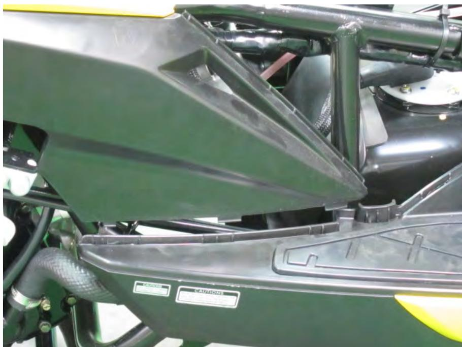
Carefully push the hooks into the corresponding tabs on both sides of the body cover.
