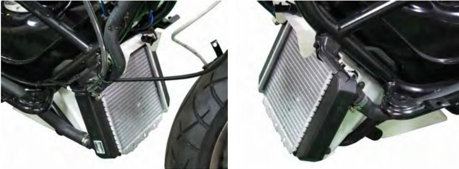
There are two coolant hoses that connect to the radiator. The top left hose runs to the filler neck and cap. The top right hose runs to the thermostat on the cylinder head. The bottom left hose runs to the water pump.
