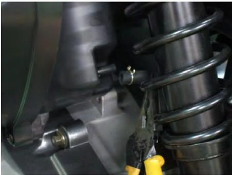
Disconnect the blow-by tube mounting the transmission box assy.
