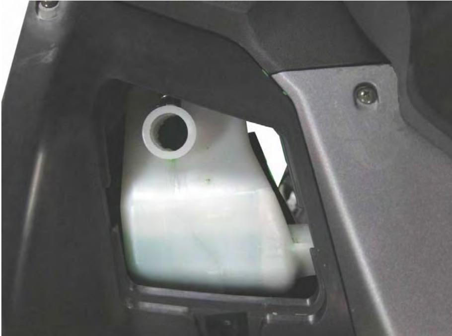
Open the coolant reserve tank lid. Siphon the coolant out of the reserve tank with an appropriate suction device. If a suction device is unavailable remove the reserve tank and pour it out. See the Radiator topic for more information.
