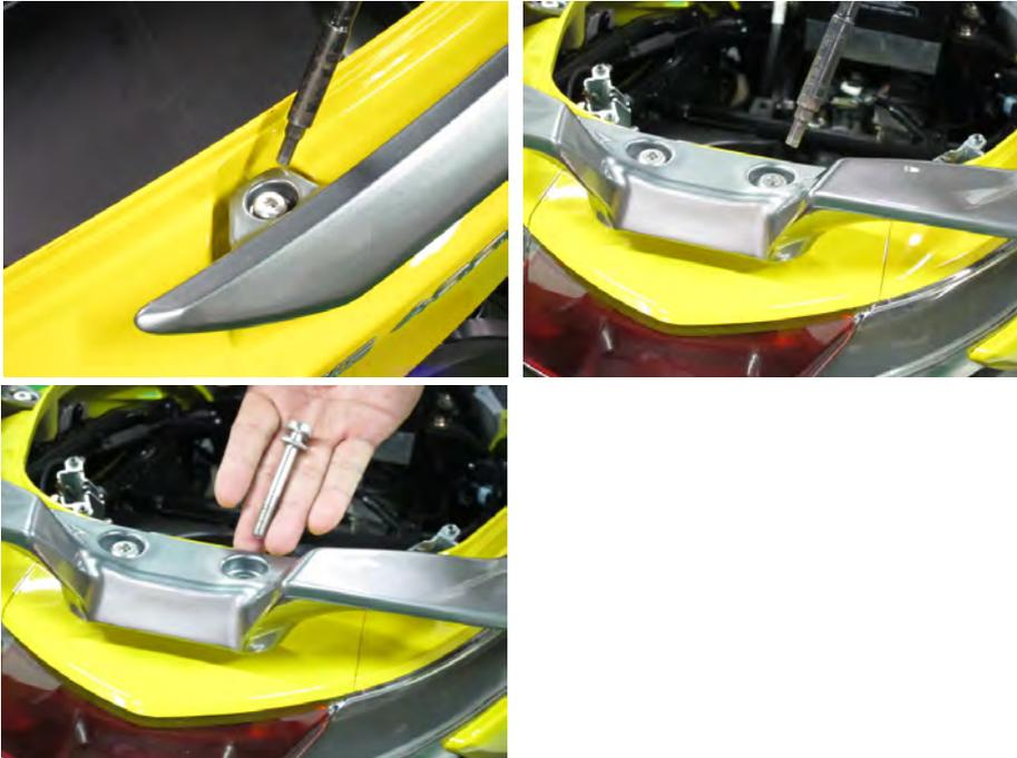
Remove the four carrier bolts with a 6 mm Allen.
