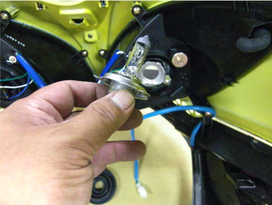
Fit the bulb into the lamp and then remove the headlight bulbs to free it from the lamp.
