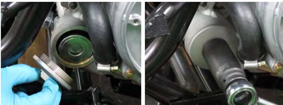
Install the oil filter cap with spring. Make sure the spring fits against the filter correctly. Tighten the oil filter cap securely with a 24 mm socket.
