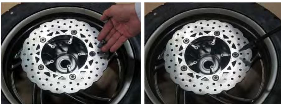
Apply a non-permanent thread locking agent to the threads of the rear disc bolts. Insert the bolts and tighten them to specification with a 6 mm Allen.
