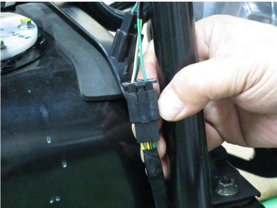
Unplug the three-pin side stand switch connector.
