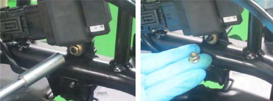
Remove the two mounting nuts with a socket.
