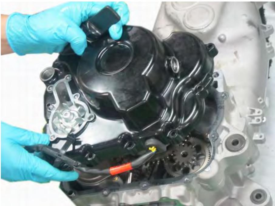
Fit the generator cover into place. Make sure the water pump shaft engages correctly with the oil pump shaft.
