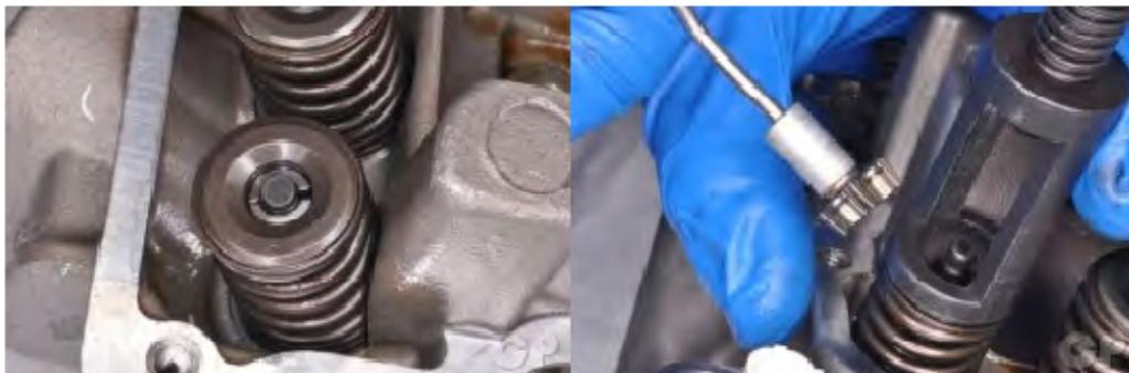
Remove the split keepers. There are two per valve.
