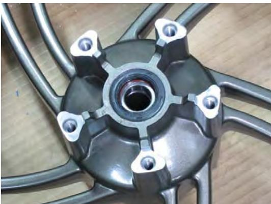
Apply grease to the lips of the dust seals. Drive in new dust seals. Use a suitable driver that has the same outside diameter as the seal. The dust seals should be flush with the wheel hub.
