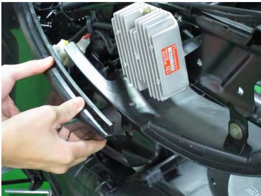
The regulator/rectifier is located on the right side of the vehicle.
