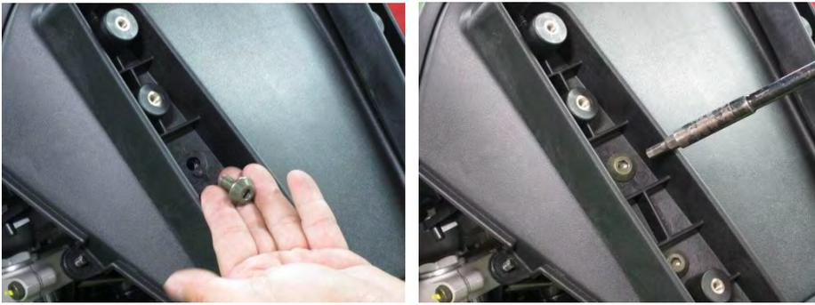
Install the four cover windshield bolts with a 6mm Allen.
