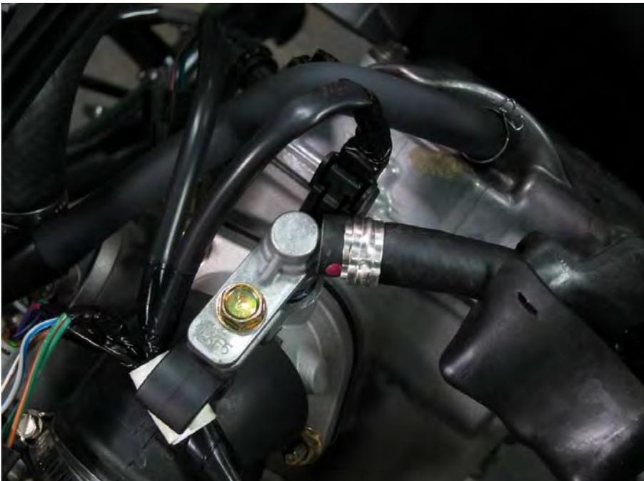
Inspect the fuel hose for damage and deterioration.
