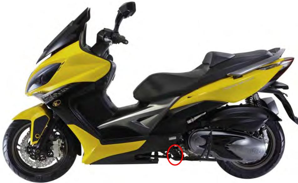
The VIN is stamped on a plate on the lower left side.
