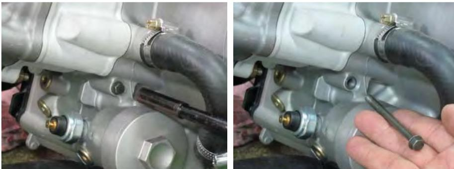
Loosen the 12 crankcase bolts in a crisscross pattern with an 8 mm socket. Remove the crankcase bolts from the left side of the engine.
