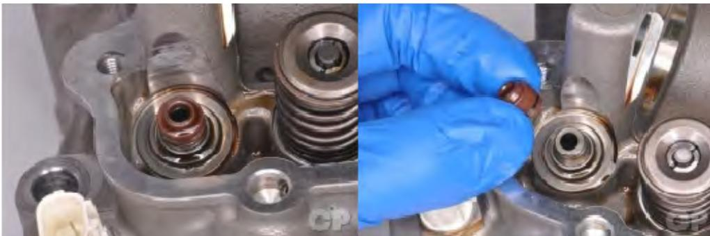
Remove the valve seal from the valve guide. The valve seals should be replaced if they are removed or you are going to install new valves.
