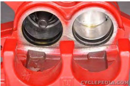
Each piston bore has two seals. The outer seal is the dust seal and the inner seal is the fluid seal.
