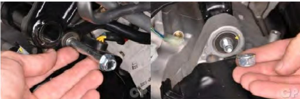
Insert the engine mounting bracket and damper bolt from the right side. Thread on the nut.
