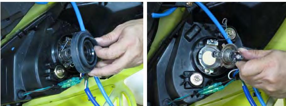
Slide back the rubber headlight covers and then remove the headlight bulbs to free it from the lamp.
