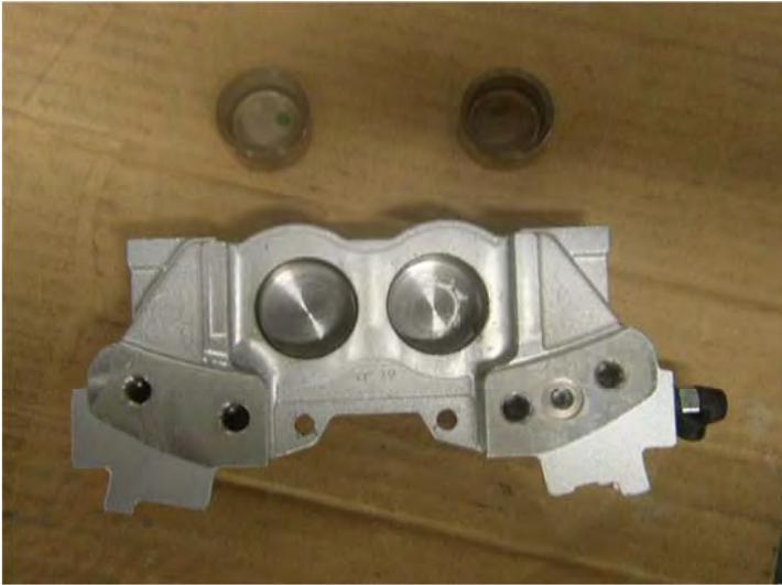
Inspect the pistons for wear and damage.
