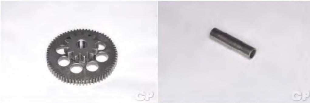
Inspect the starter idle gear and shaft for wear and damage. Replace the idle gear and shaft as needed.
