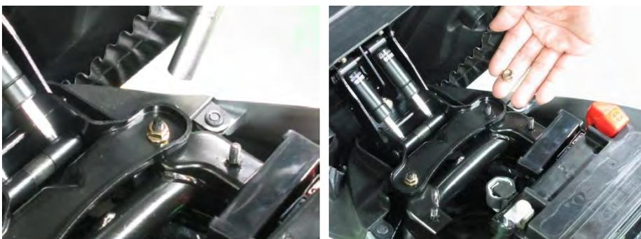
Remove the two luggage box hinge nuts with a 10 mm socket.
