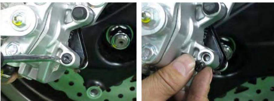
Remove the brake pad pin plug with a flat blade screwdriver.
