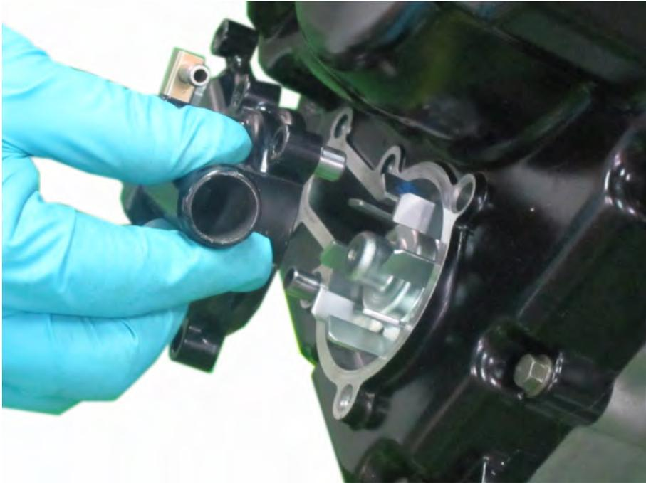
Remove the two dowel pins and the water pump cover gasket.
