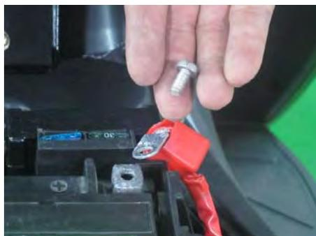
Remove the positive battery cable bolt with a 10 mm socket or #3 Phillips screwdriver.
