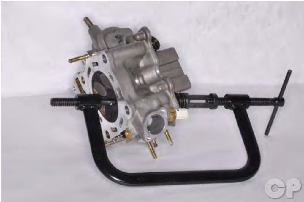
Push down the valve springs with a valve spring compressor.
