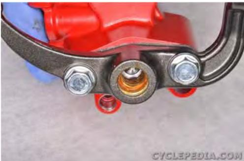
Remove the two parking brake bracket bolts.
