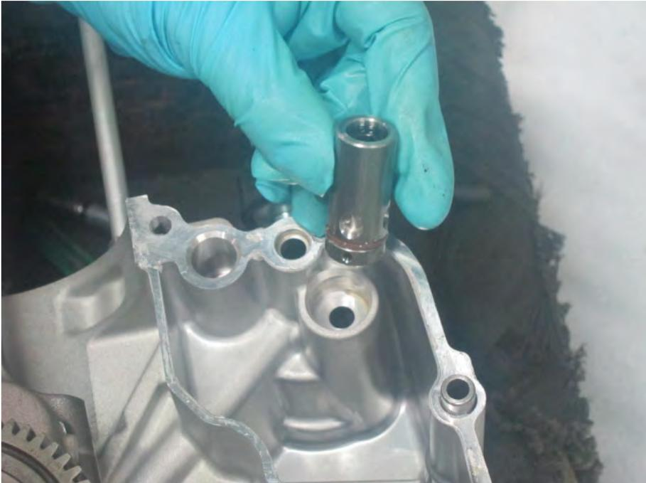
Remove the oil release valve. Inspect the O-ring and replace it as needed.
