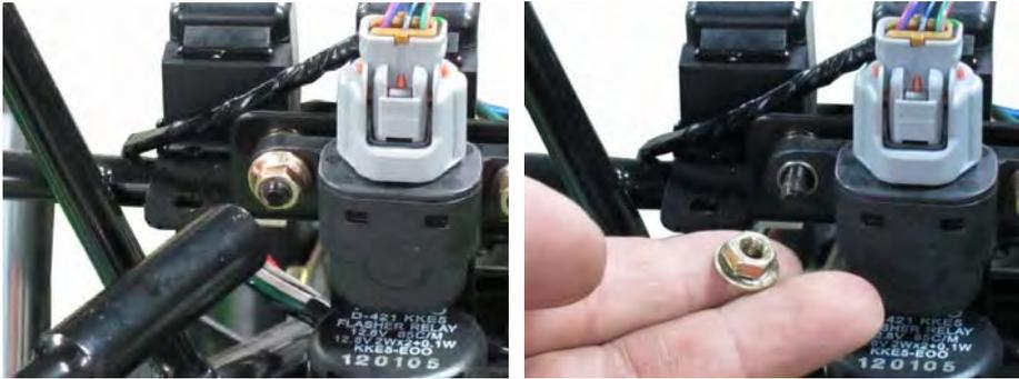
Remove the two tilt switch bolts with a 10 mm socket.
