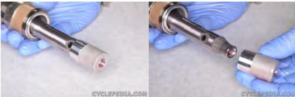
Remove the oil lock piece. The oil lock piece may come out with the damper rod in the inner fork tube or it may remain in the slider.
