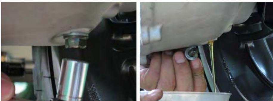
Place a suitable container under the drain plug to capture the final drive oil. Loosen the oil drain plug with a 12 mm socket. Remove the drain plug and slowly rotate the rear wheel to drain the transmission oil.
