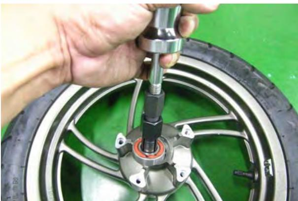
Repeat the procedure and remove the other bearing and seal.
