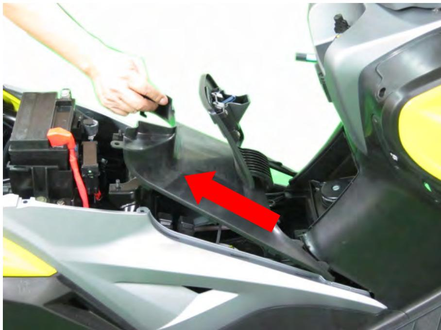
Pull the center cover back and up to free the claws and then move the cover backward to free it from the scooter.
