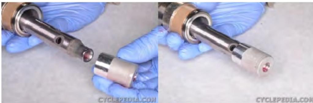
Place the fork oil lock piece on the end of the damper rod.
