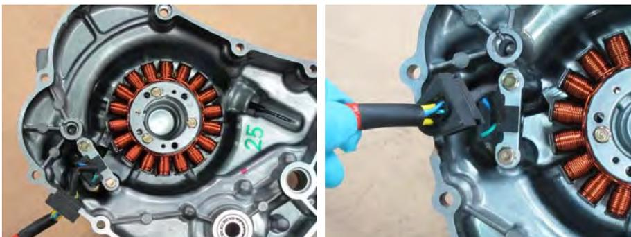
Coat the rubber grommet in silicone sealant where it contacts the generator cover. Fit the rubber wire grommet into its cutout in the crankcase cover.
