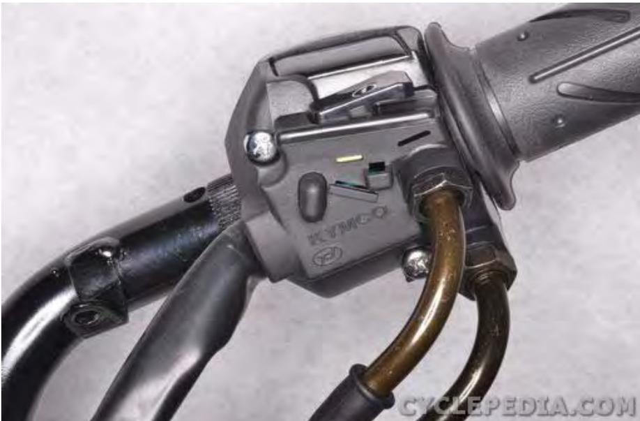
Remove the two right switch housing mounting screws with a #2 Phillips screwdriver.
