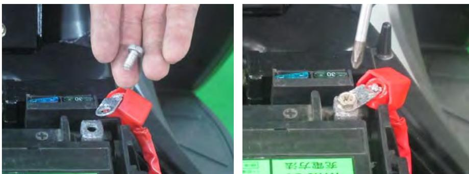
Connect the positive battery cable and install the bolt with a 10 mm socket or #3 Phillips screwdriver.
