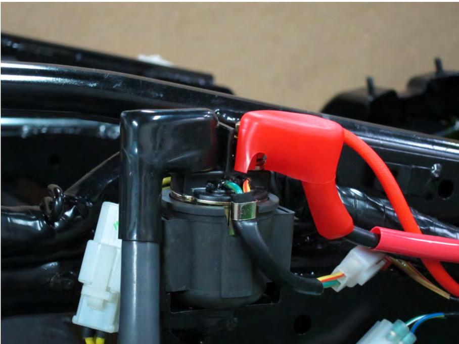
The starter relay is located on the right side of the vehicle.
