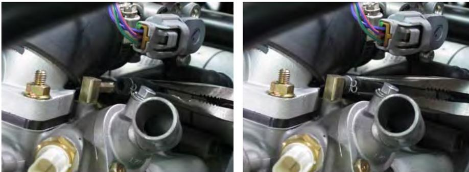
Install air bleed hose and secure it with the clamp.
