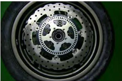
Install the front wheel speed sensor rotor. Tighten the five bolts securely.
