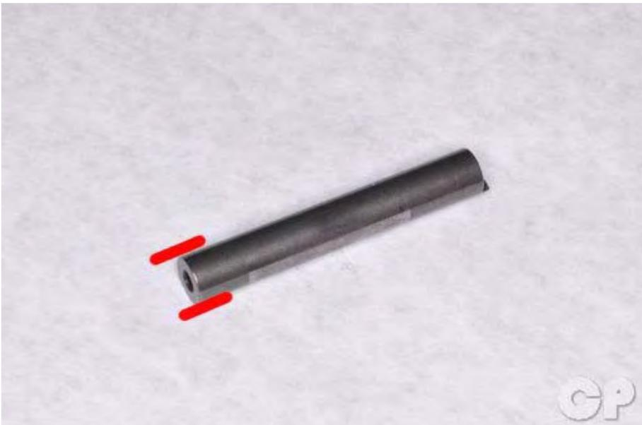
Inspect the rocker arm shaft outer diameter for the intake and exhaust valves.
