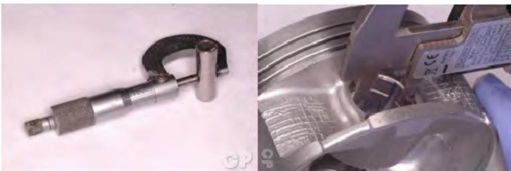
Measure the piston pin diameter with a micrometer. Measure the piston pin bore diameter with vernier calipers or a small bore gauge. Measuring at three different points for each. Replace the parts if any of the specifications are not met.
