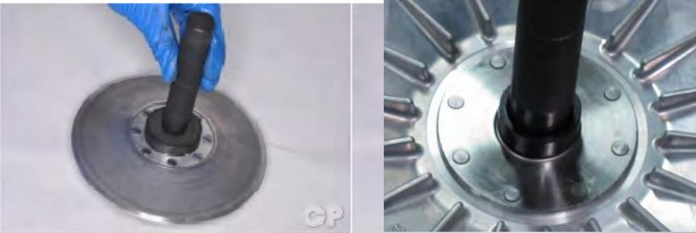
Drive in the new seals with a suitable driver with the same outside diameter as the seal.
