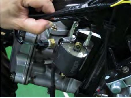
Remove the two ignition coil leads.
