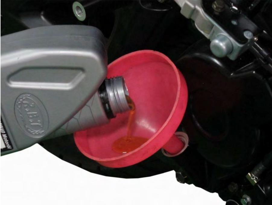
Add the oil to the engine through the oil filler/dipstick hole.
