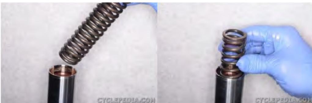
Fully extend the fork and insert the fork spring with its tightly coiled end facing down towards the axle.
