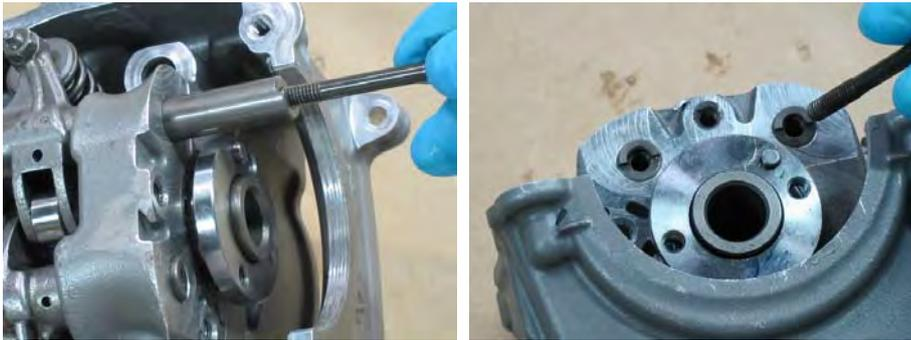
Wipe the rocker arm shafts clean. Insert the rocker arm shafts through the camshaft holders and rocker arms. Install the rocker arm shafts so that the end sits as shown.
