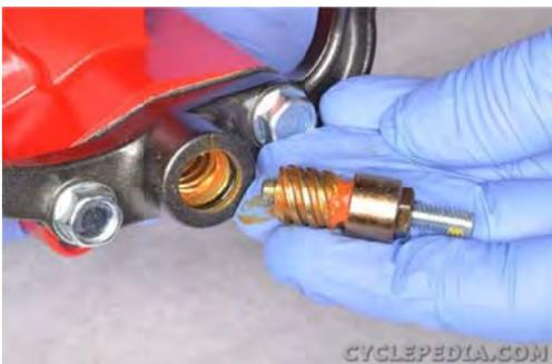
Remove the parking brake shaft and adjuster bolt.
