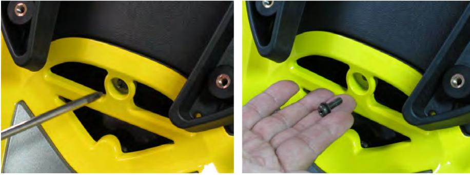
Remove the center front cover mounting screw with a #2 Phillips
