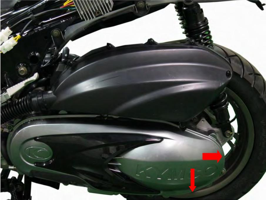
The oil drain bolt and oil filler bolt are located on the transmission.
