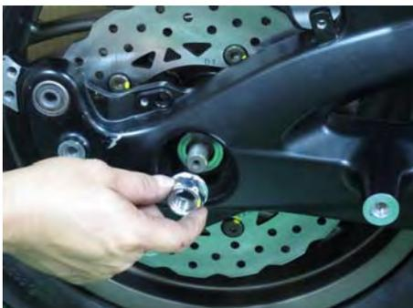
Remove the rear axle nut with a 24 mm socket.
