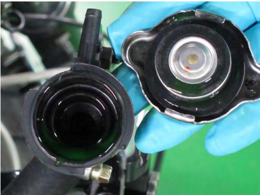
Wet the seal of the radiator cap and install.
