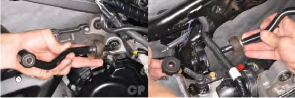
Fit the engine mounting bracket and damper assembly into place.
