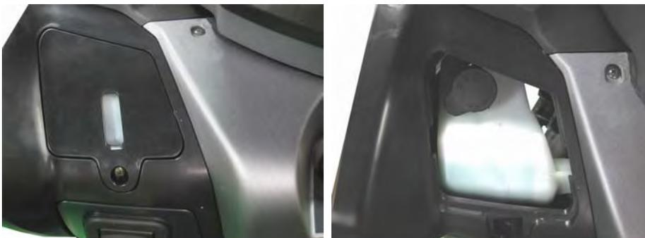
The coolant reserve tank is behind the inner cover.
