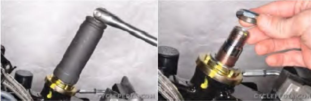
A special lock nut wrench is needed to loosen the steering stem lock nut. Remove the steering stem lock nut.
