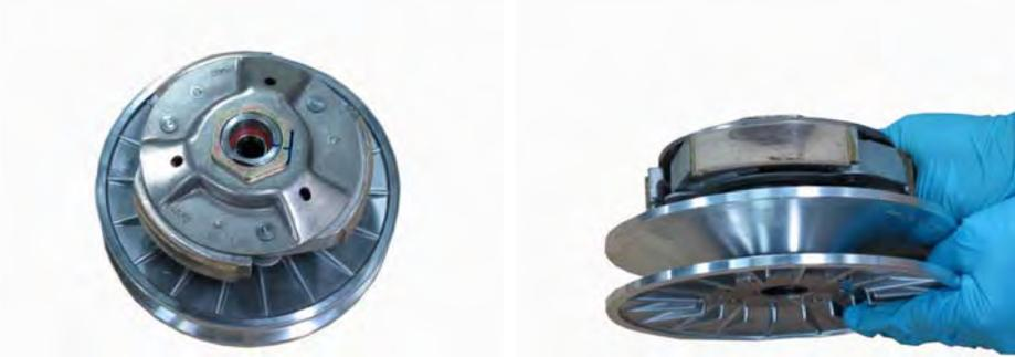
Inspect the clutch shoe lining thickness.
