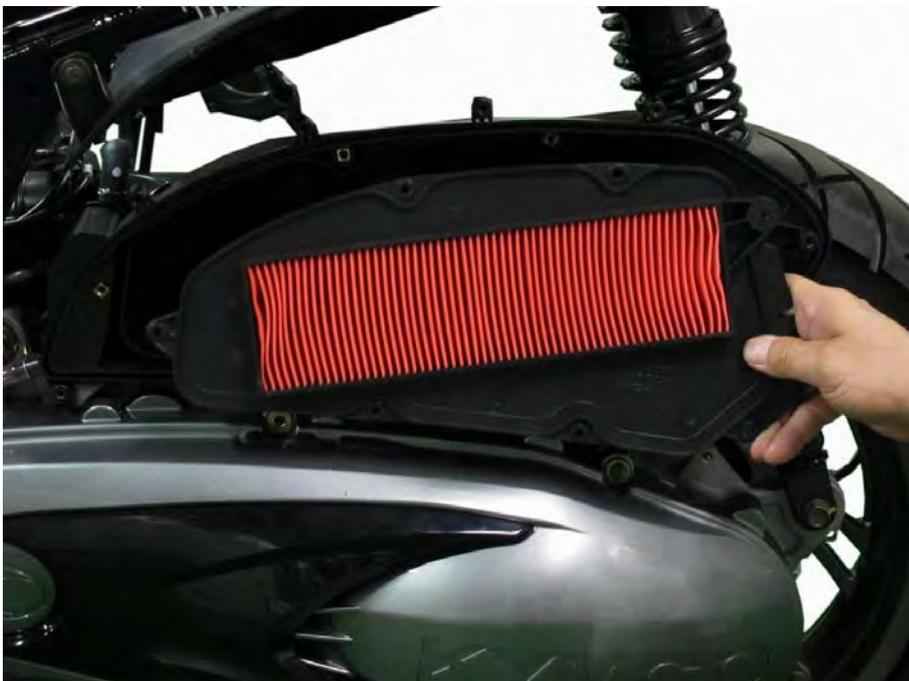
Remove the air filter from the airbox. Discard the air filter in favor of a new item.
