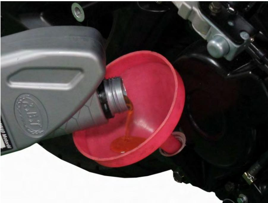
If the oil level is at or below the lower mark add more of the same type and brand of oil to the engine through the oil filler hole. If the oil level is too high remove the drain plug and the excess oil.
