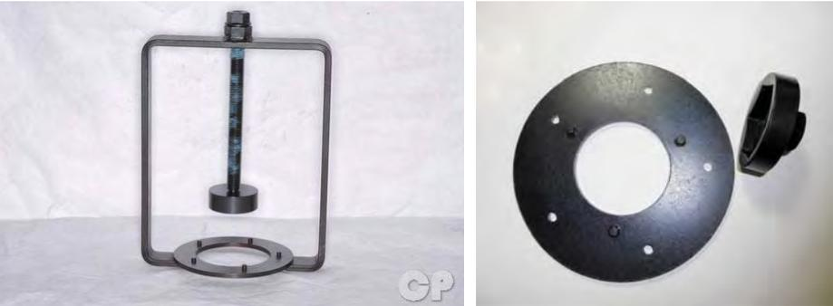
Fit the clutch and fitting tool into the clutch spring compressor tool.
