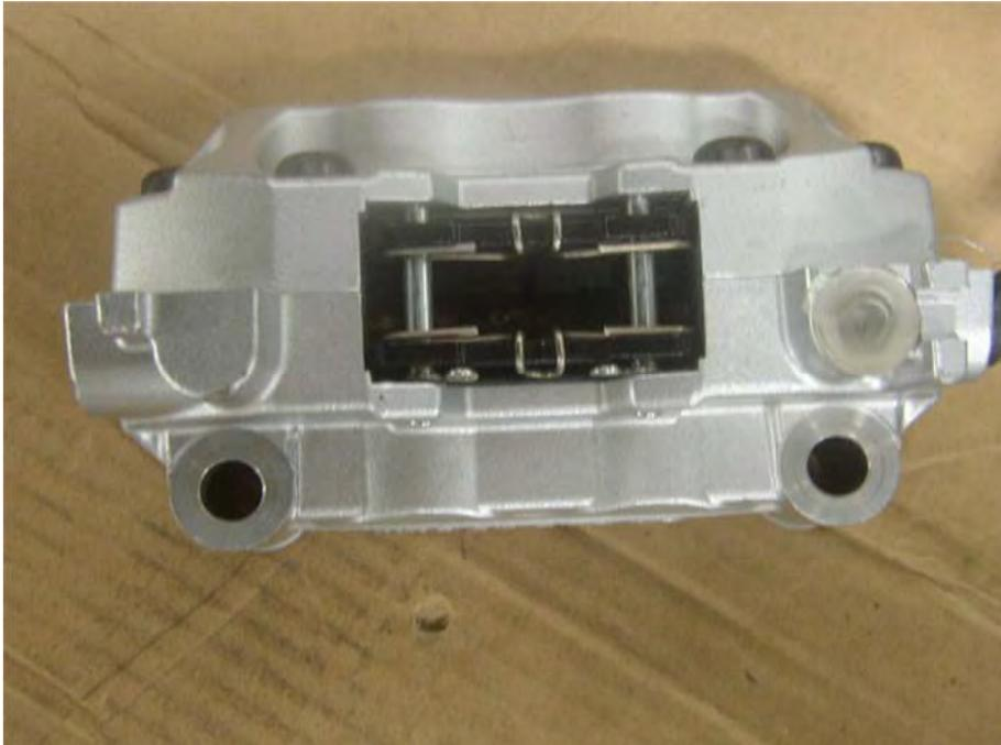
Remove the pad retainer from the brake caliper bracket if needed.
