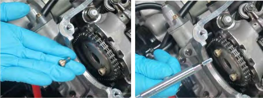
Apply a small amount of blue Loctite (non-permanent) to the threads of the camshaft sprocket bolts. Thread in the camshaft sprocket bolts and tighten to specification using a 5 mm Allen socket.
