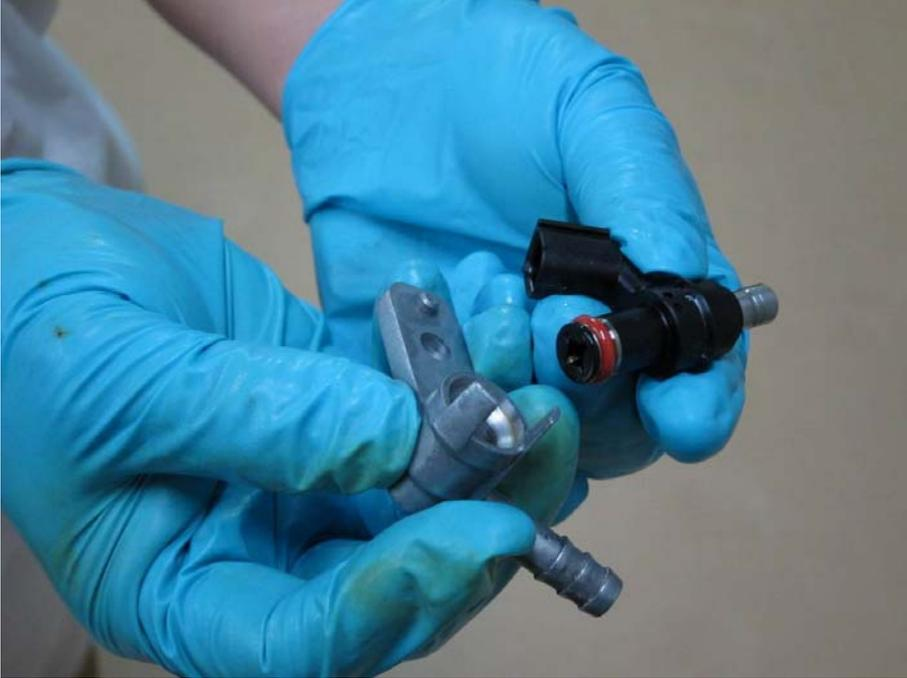
Fit the fuel injector pipe onto the top of the injector.
