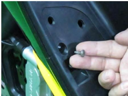
Remove the left leg shield mounting screws with a #2 Phillips.
