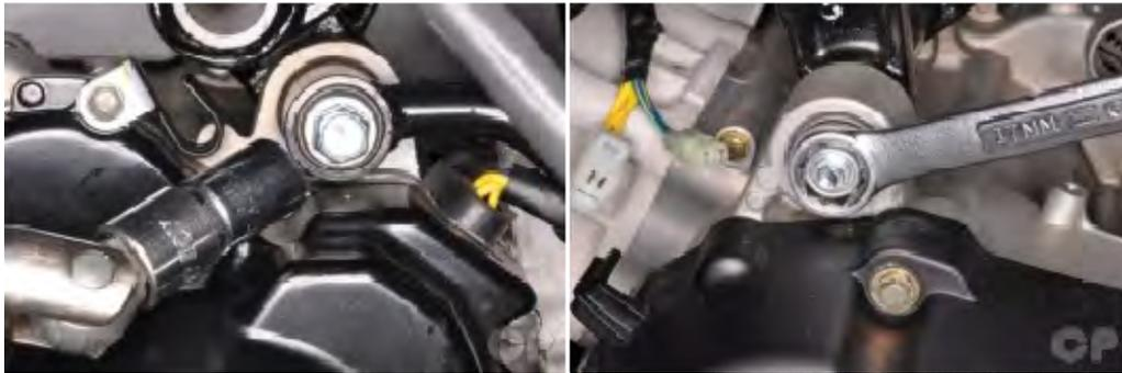
Tighten the engine mounting bracket damper bolt and nut with a 17 mm wrench for the nut and a 14 mm socket for the bolt.
