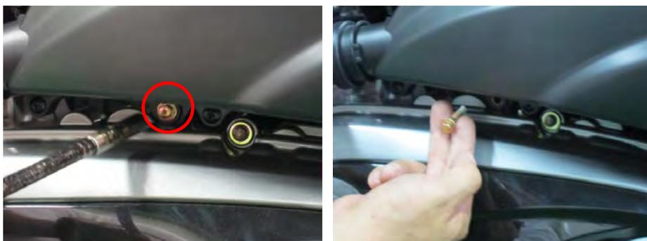
Remove the two air box bolts with an 8 mm socket.
