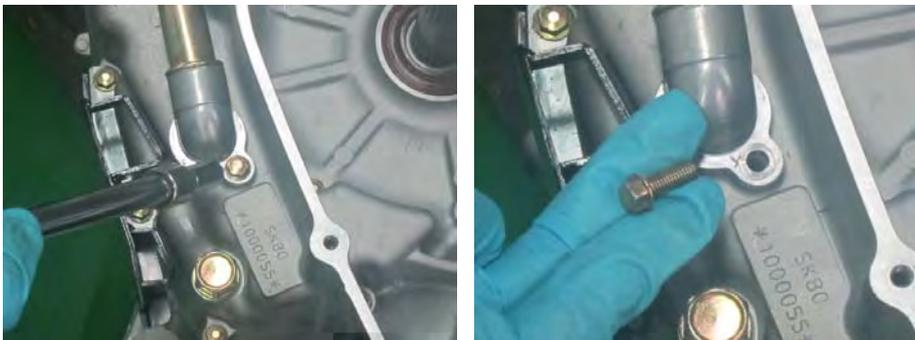
Loosen the right crankcase coolant hose clamp with a 8mm socket. Slide up the clamp and free the coolant hose from the right crankcase cover. Allow any remaining coolant to drain into a suitable container.
