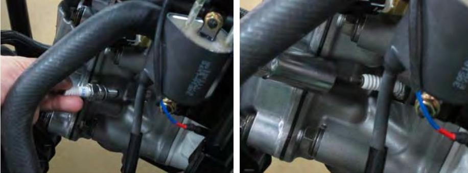
Thread the spark plug by hand before using a socket to tighten. Torque to specification with a 5/8" spark plug socket. Do not over tighten the spark plug. The cylinder head is made out of soft metal, and it can be easily damaged.
