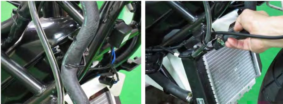
Route the filler neck coolant hose through the guide to the top left of the radiator.
