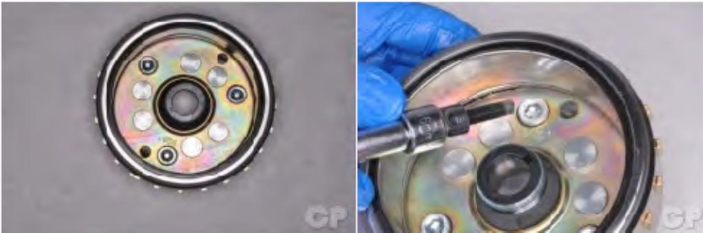
Remove the three starter clutch mounting bolts with a 6 mm Allen socket.
