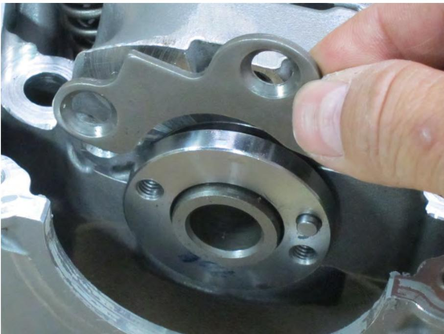
Install the camshaft set plate so it fits into the groove on the camshaft and between the projections on the rocker arm shafts.
