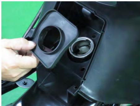
Remove the fuel cap with the key.
