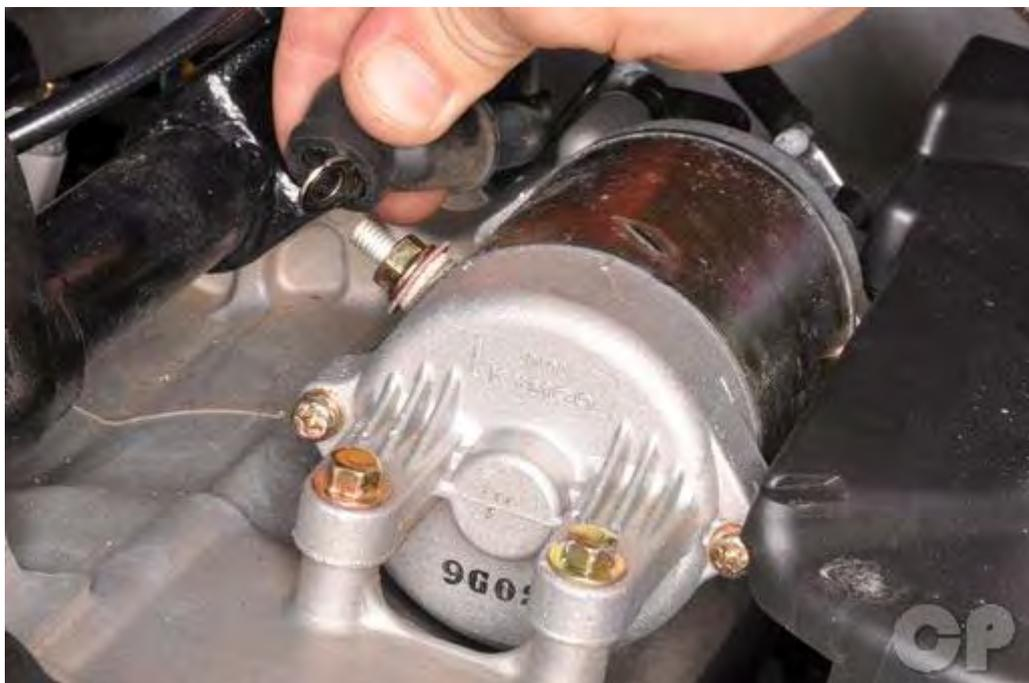
Remove the starter motor lead nut with a 10 mm wrench. Free the cable lead from the starter motor. Thread the nut back on to keep track of it.
