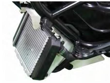
Fit the radiator into place so that the post on the frame fits into the rubber grommet on the right side of the radiator.
