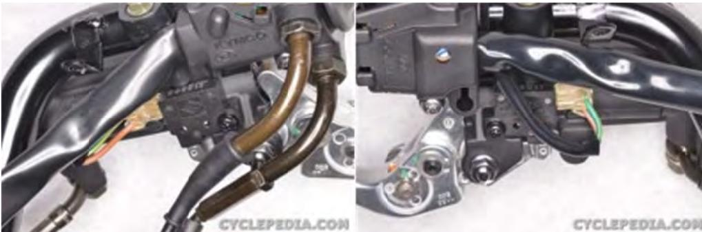
Unplug the brake light switch connectors.
