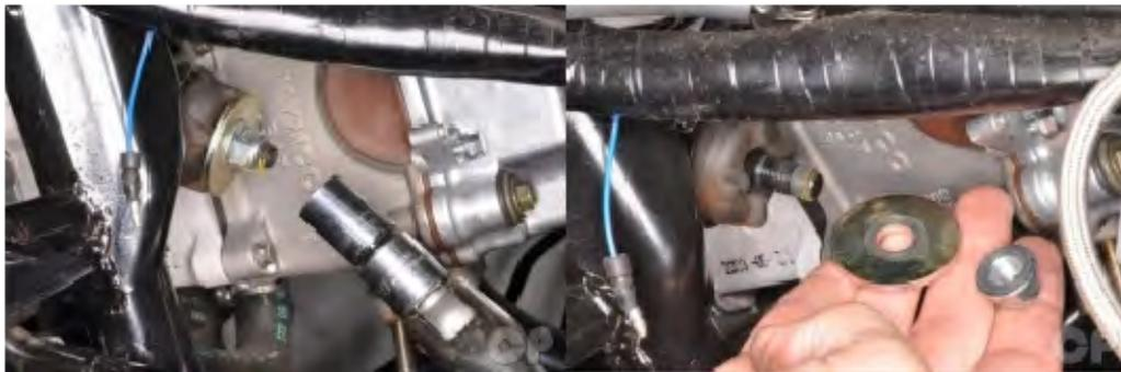
Loosen the engine mounting bracket damper nut with a 14 mm socket.
