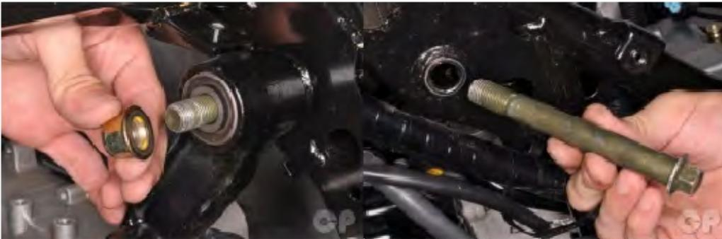
Remove the engine mounting nuts and bolts from both sides.
