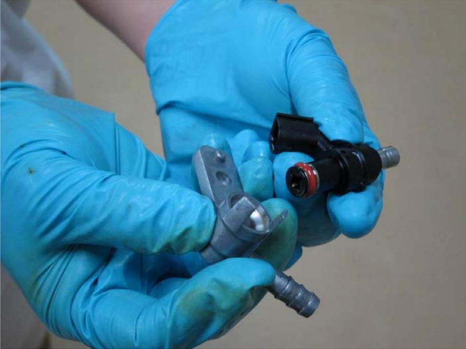
Lift the fuel pipe off the top of the injector.
