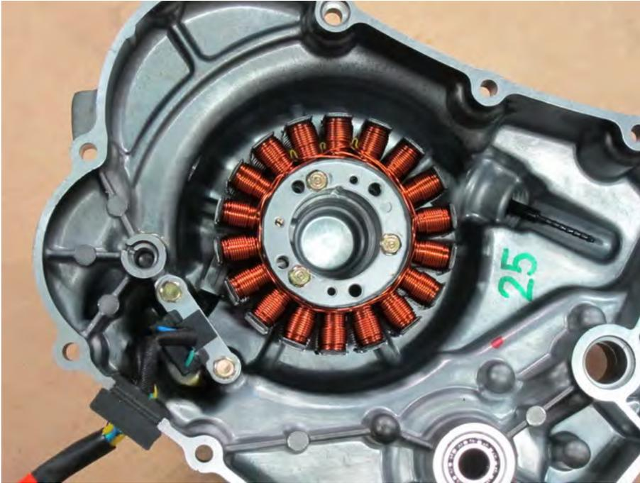
Fit the stator and the crankshaft position sensor into the generator cover together as shown. Insert the two crank position sensor mounting bolts and the three stator mounting bolts. Tighten the bolts securely with an 8 mm socket.
