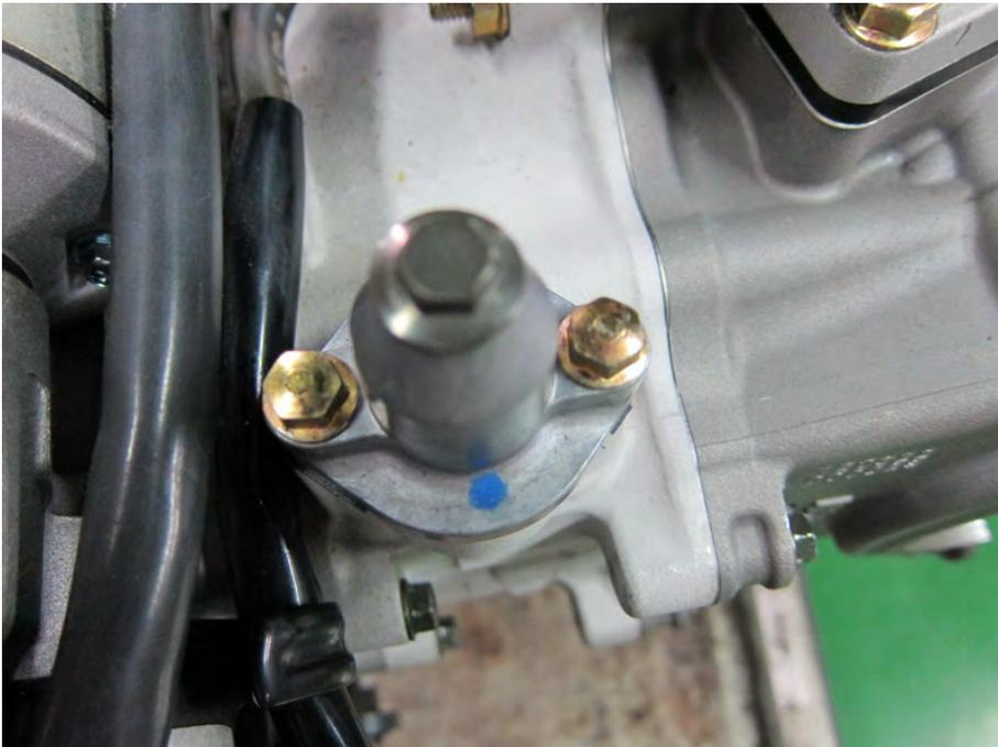
The cam chain tensioner is located on the back of the cylinder.
