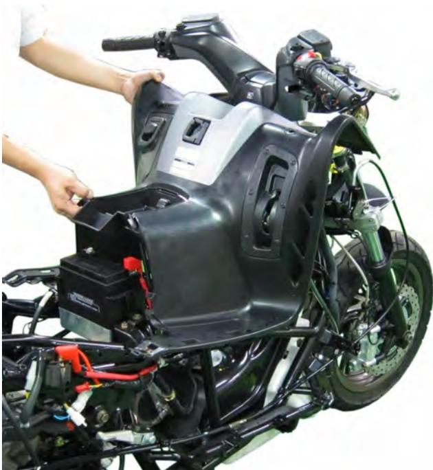
Install the inner cover and align the bolt holes.
