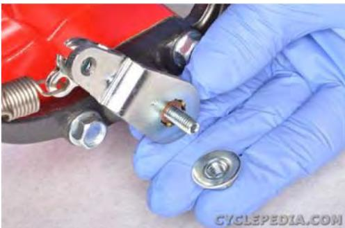
Remove the parking brake lock nut.
