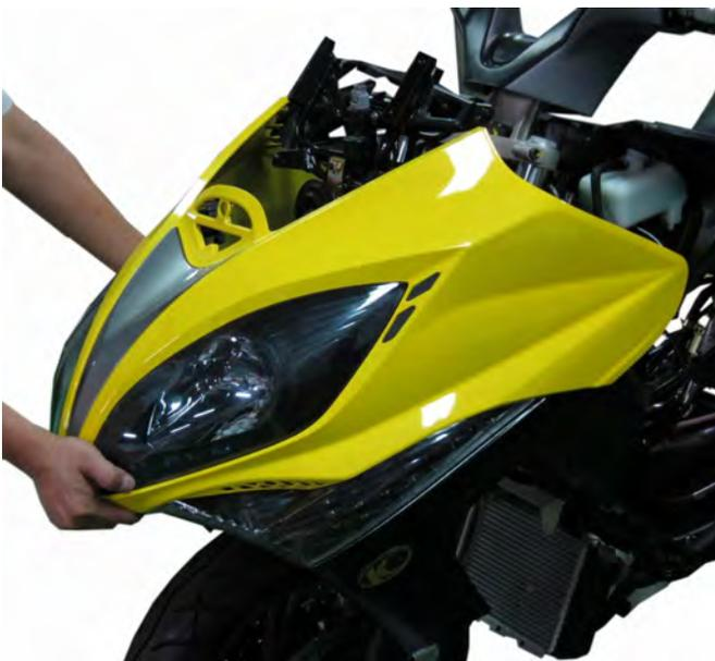
Align front cover tabs. Install the front cover.
