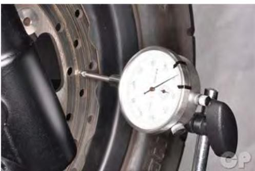
Check if the brake rotor runout is within the service limit.
