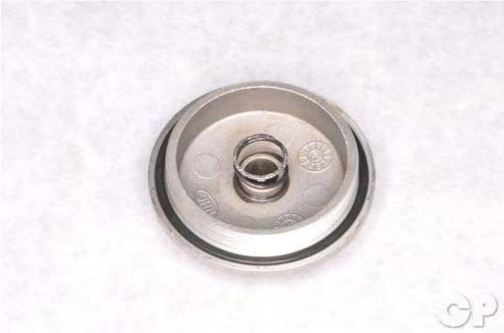
Inspect the oil filter cap O-ring and spring. Replace the items if they are in poor condition.
