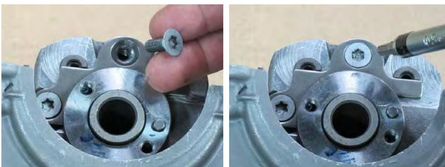
Apply a small amount of blue Loctite (non-permanent) to the threads of the set plate bolt. Thread in the bolt and tighten it to specification with a 5 mm Allen socket.
