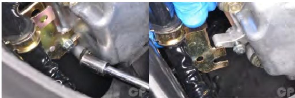
Loosen the fuel hose stay bolt with an 8 mm socket. Free the fuel hose stay from the cylinder head cover.
