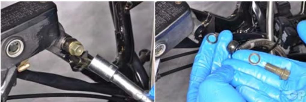
Remove the brake hose banjo bolt from the master cylinder using a 12 mm socket. Discard the sealing washers.
