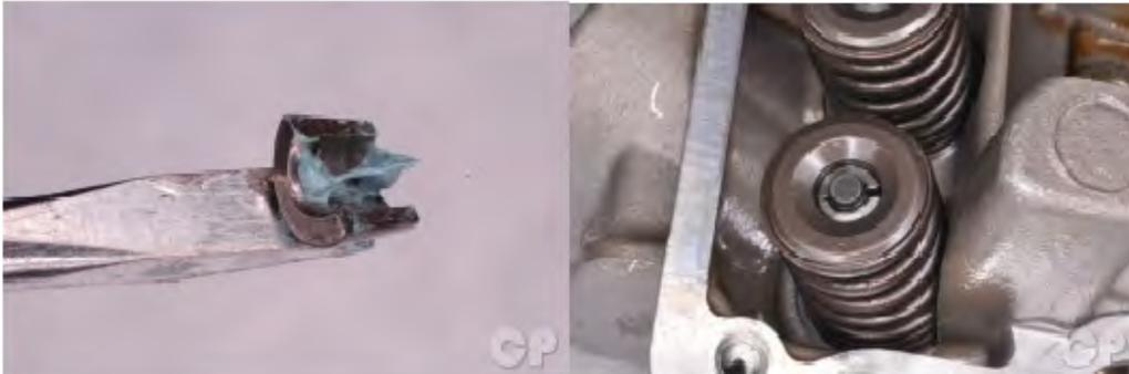
Apply grease to the inside of the split keepers. Apply a dab of grease to the end of a flat blade screwdriver. Set the keeper in the grease on the screwdriver and insert it onto the valve stem. Repeat this with the other keeper.
