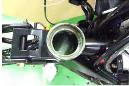
Inspect the bearings and races for wear and damage.
