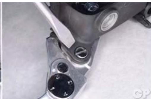
Loosen the brake lever pivot nut with a 10 mm socket and the pivot bolt with a flat blade screwdriver.
