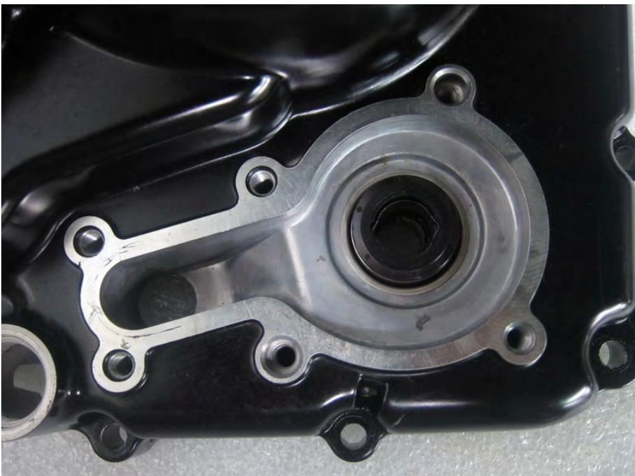
To replace the mechanical and oil seals drive them out from the inside of the generator cover.
