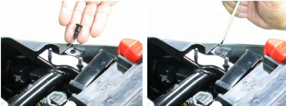
Install the two seat plastic screws from the front of body cover.
