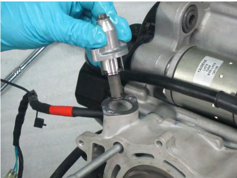
Lift the cam chain tensioner out of the cylinder.
