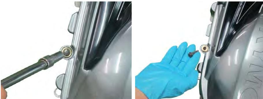
Remove the crankcase cover protector on the left side of the engine with a 8mm socket.
