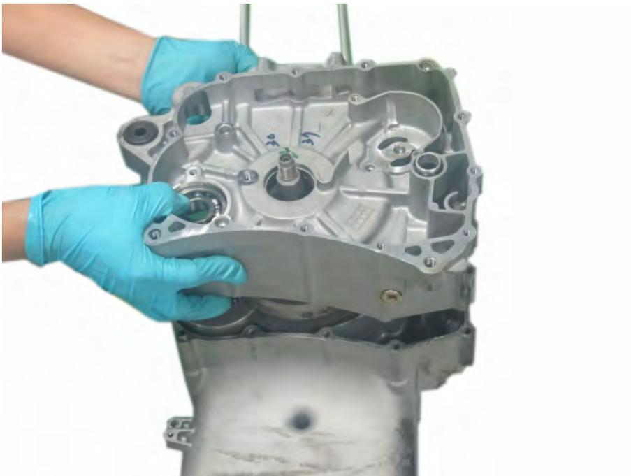
Separate the halves of the crankcase. If needed gently tap the reinforced areas of the right crankcase half with a rubber mallet. Lift the right crankcase off of the left.
