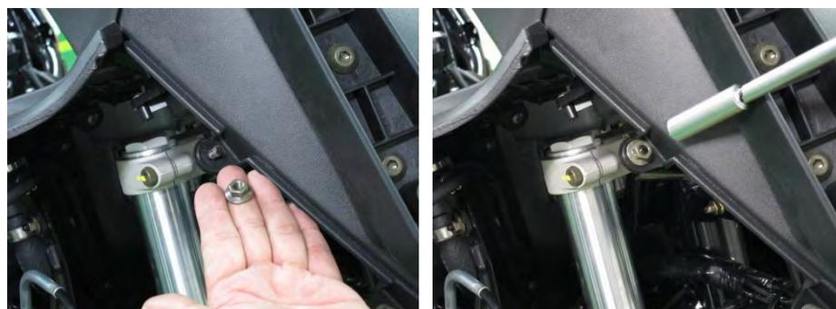
Install the two nuts mounting on the front cover meter on both side.
