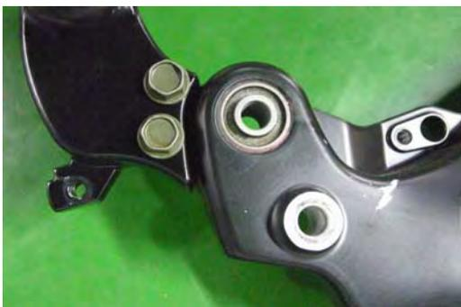
Inspect the shock absorber bushings for wear and damage.
