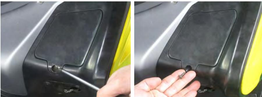
Remove the radiator coolant panel screws with a #2 Phillips screwdriver.
