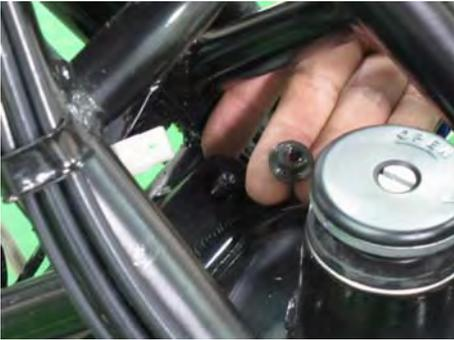
Remove the front fuel tank mounting nuts.
