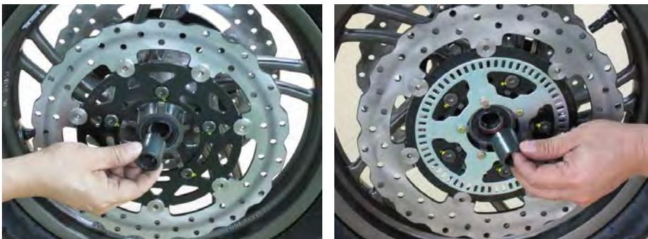
Remove the collars from each side of the wheel. Inspect the bearing seals and the O-rings seals on the collars. Replace the seals if they are in poor condition.
