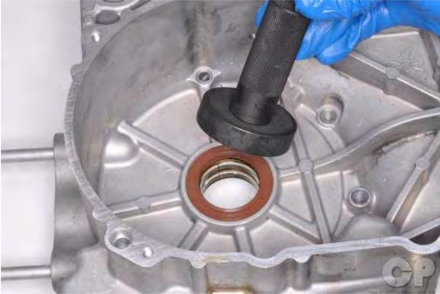
Drive the new seal into the left crankcase from the outside with a suitable driver. The driver should have the same outside diameter as the seal. Lubricate the new crankshaft seal lips with fresh engine oil.
