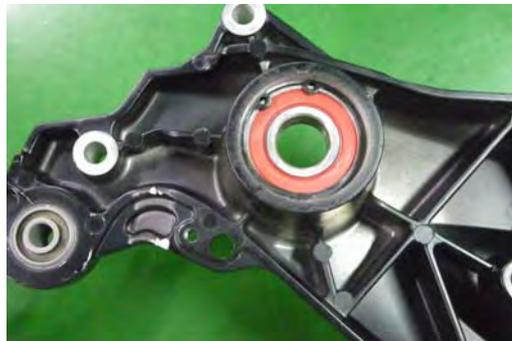
Inspect the wheel bearing by turning it with a finger. Replace the bearing and seal as needed. Remove the seal and snap ring. Drive the bearing out from the inside out. Drive in the new bearing with a suitable driver that is the same outside diameter as the bearing. Install the snap ring into the groove. Apply grease to the lips of the new seal and drive it into place in the same manner as the bearing.
