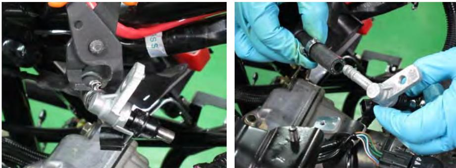
Loosen the fuel hose clamp with a special tool A120F00030.
