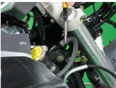
Remove the bottom hose is the overflow hose that runs to the filler neck.
