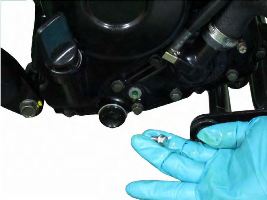
Remove the drain bolt and sealing washer and allow the coolant to drain into a suitable container.
