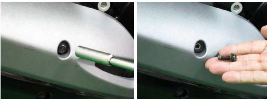
Remove the four muffler heat shield bolts with a 10 mm socket.
