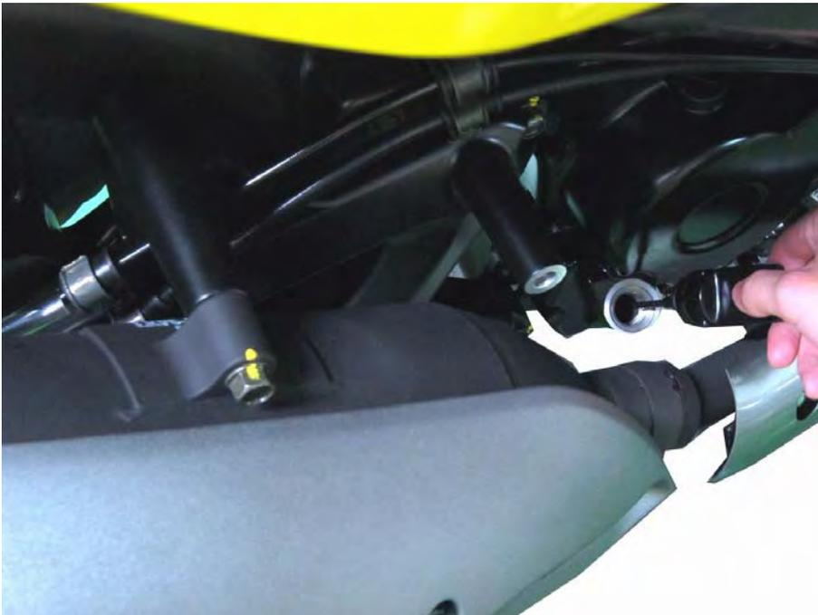
Remove the oil filler cap/dipstick and wipe off the oil. Inspect the O-ring and replace it as needed. Insert the dipstick in without threading it in. Remove the dipstick and check the oil level.
