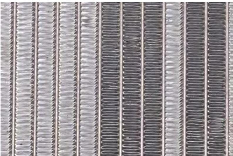
Check the radiator for any bent or damaged fins. Use a small flat blade screwdriver to straighten them out, but be careful not to puncture the radiator.
