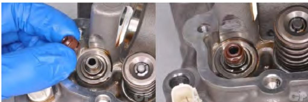
Coat the new valve seal in fresh engine oil and install it onto the valve guide.
