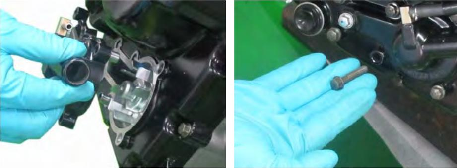
Install the water pump cover and insert the four bolts.
