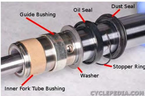
Slide on the guide bushing, washer, oil seal, stopper ring, and dust seal from the top of the fork tube. Note the orientation of the seals.
