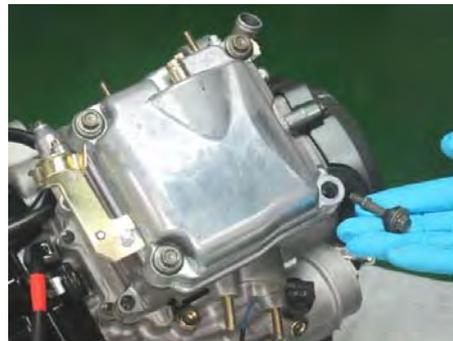
Loosen the four cylinder head cover bolts with a 10 mm socket.
