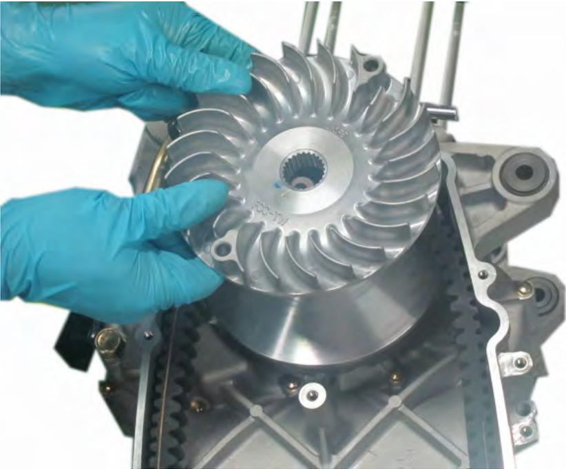
Remove the left face of the drive pulley.
