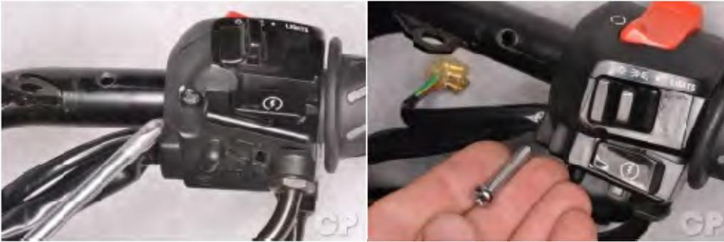
Remove the two right switch housing mounting screws with a #2 Phillips screwdriver. Disconnect the switch.
