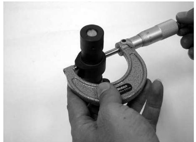
Check each camshaft for wear or damage.
