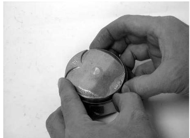
Install the piston rings onto the piston and measure the piston ring-to-groove clearance.
