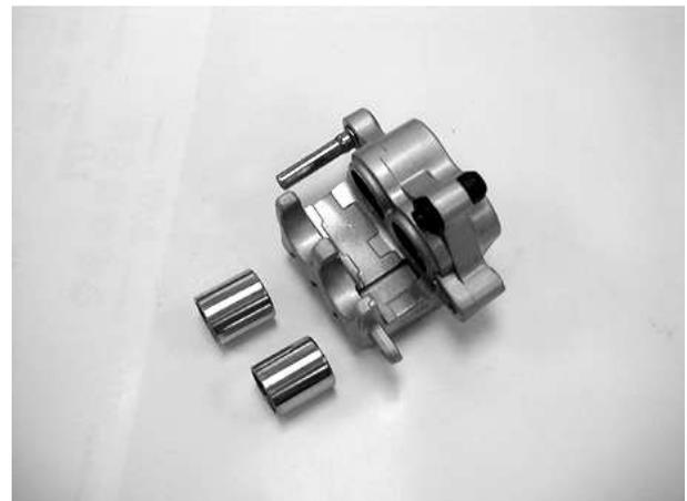
Check each caliper and caliper cylinder for scratches or wear and measure the caliper cylinder I.D.
