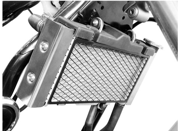
Connect the overflow tube and secure with the tube clamp.
