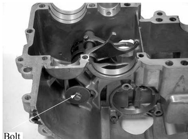
Remove the transmission fork shaft and transmission forks.
