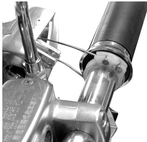
When installing the master cylinder and clutch lever holders, align the tab on the holder with the hole in the handlebar with the holder "UP" mark facing up. First tighten the upper bolt and then the lower bolt.
