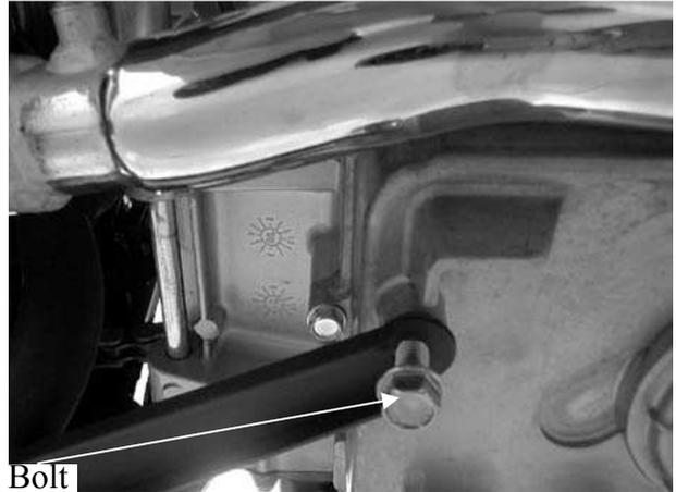
Remove the exhaust muffler hanger lock bolt.
