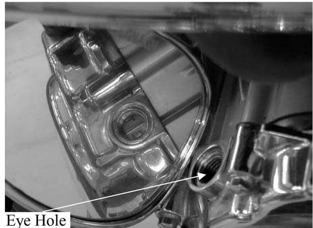
Warm up the engine and check the ignition timing with a timing light. When the engine is running at the specified rpm, the ignition timing is correct if the "F" mark aligns with the index mark on the crankcase within  $\pm 2^\circ$ .
