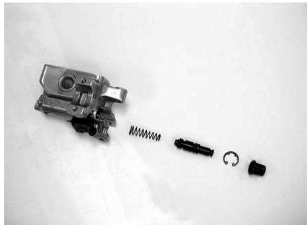
Install the main piston and snap ring.
