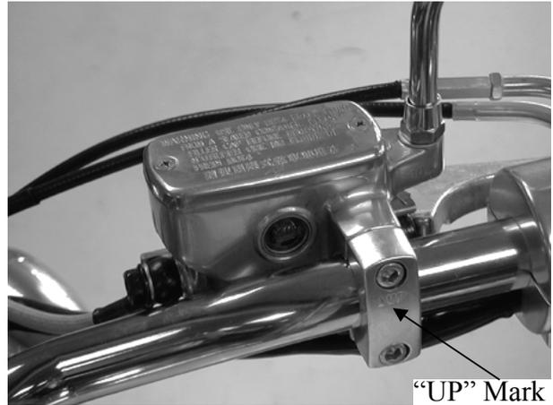
Install the brake fluid tube with the bolt and two sealing washers. Then, install the rearview mirror.
