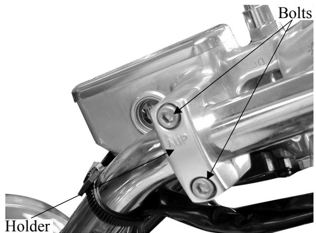
Remove the two left handlebar switch housing screws and the housing. Remove the two clutch lever holder bolts and the clutch lever holder.
