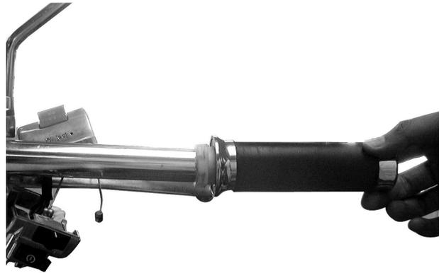
Connect the throttle cable to the throttle grip. Apply grease to the throttle cable. Install the throttle housing by aligning the pin on the housing with the punch hole in the handlebar. Then, tighten the two screws.
