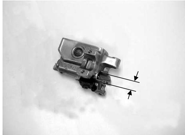
Measure the brake master cylinder piston O.D.
