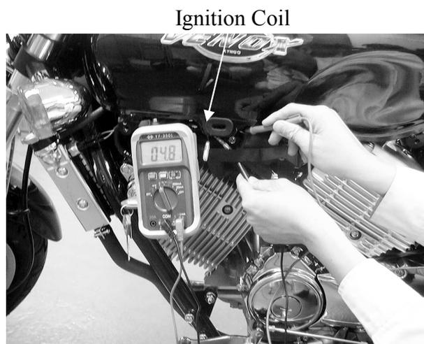
Measure the secondary coil resistance between the spark plug wire and the primary coil terminal.
